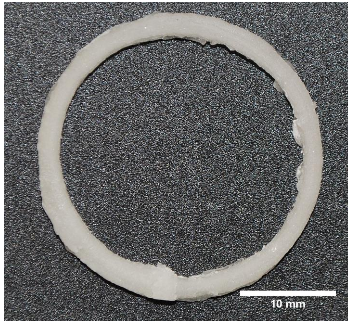
Figure 4-11. Additively manufactured ring that was UV-cured using a modified VAP system [54]. The ring was cured every few layers.
