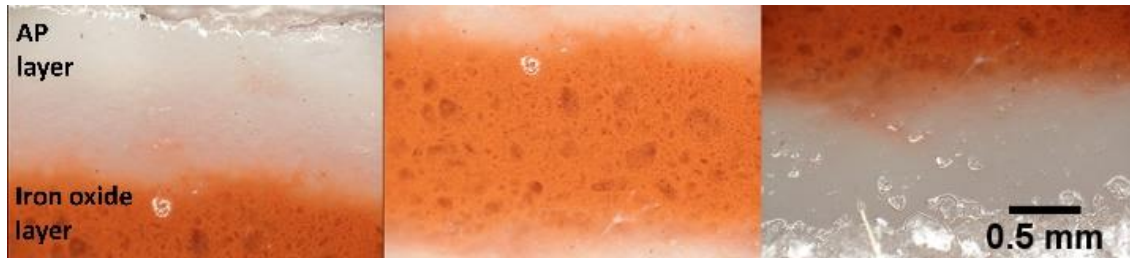
Figure 6-1. Microscopic images of LFeOCP. The outer layers are monomodal 60-130 \mu\text{m} AP/HTPB (85 wt.% solids loading) propellant and the middle layer is catalyzed with 1 wt.% iron oxide [59].
