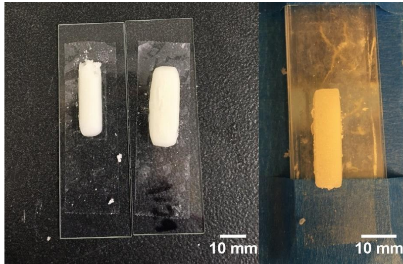
Figure 3-2. Top views of 3D printed propellant strands with 85 wt.% solids loading and varying CFR. 3D printed (left) monomodal coarse propellant (which is slightly deformed), (middle) propellant with a CFR of 4:1 (which has overhang), and (right) propellant with a CFR of 1:1 (which maintains shape well).
