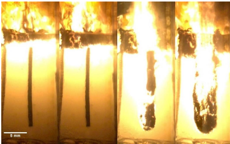
Figure G-6. Convective burning of Al/PVDF wire embedded in AP/HTPB propellant at 3.45 MPa. There are 0.1 s between frames.
