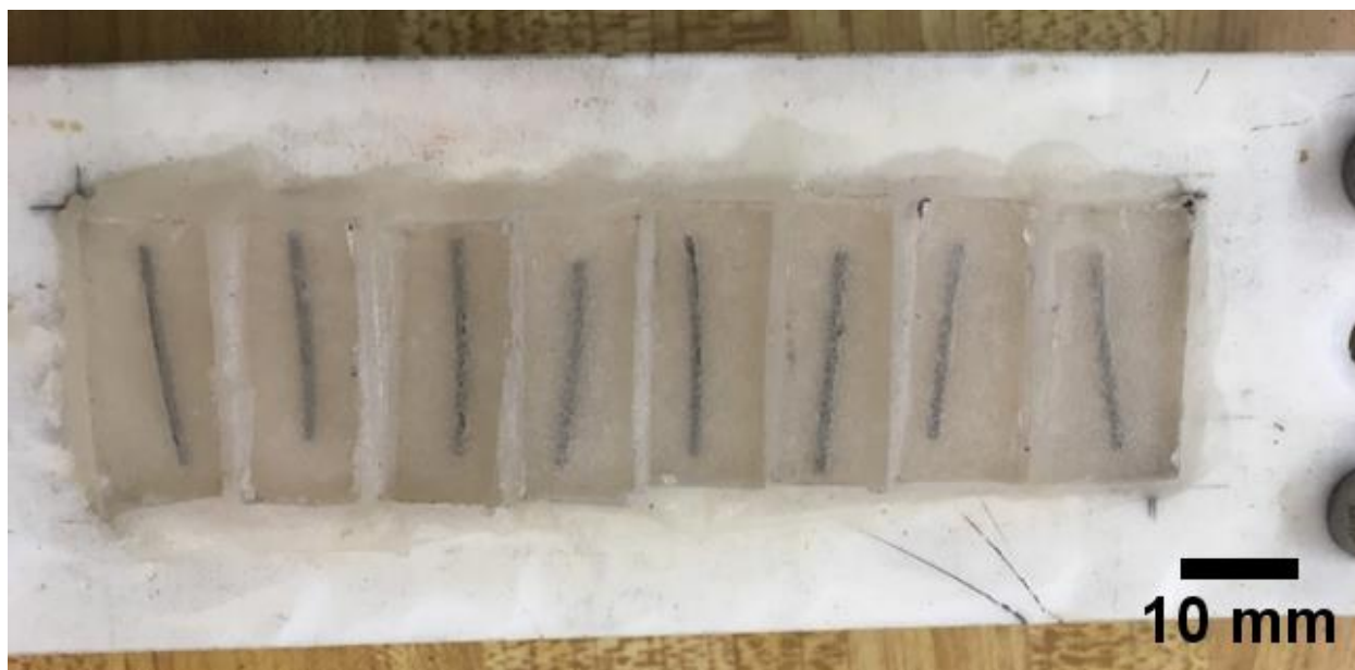
Figure G-1. Embedded Al/PVDF filament in AP/HTPB with polycarbonate window in a Teflon mold. After curing, the propellant is cut into strands. The windows are approximately 11 x 24 mm.
