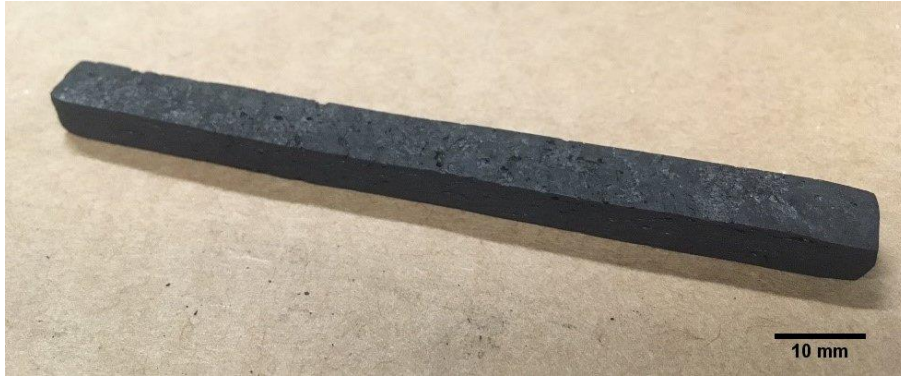
Figure E-5. Pyrolyzed C bar for flexural strength testing [66].
