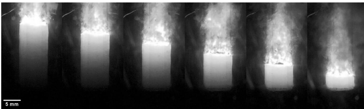
Figure 3-8. A printed HTPB strand burning at 10.34 MPa with 300 ms between each frame [37].
