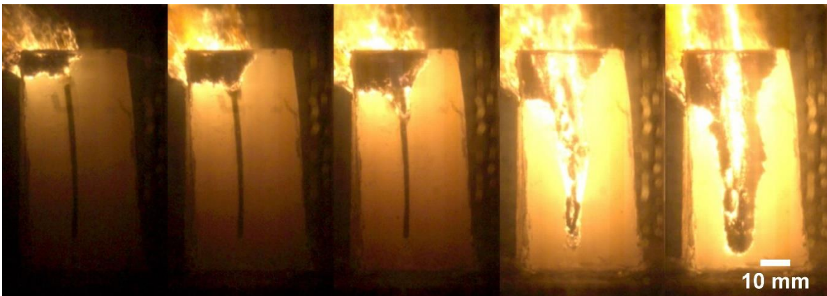
Figure G-8. Convective burning of Al/PVDF wire embedded in AP/HTPB propellant at 6.89 MPa. There are 0.1 s between frames.
