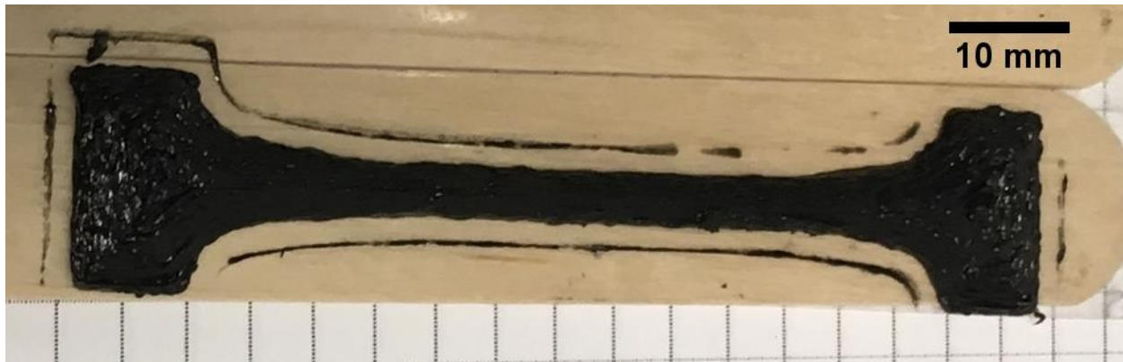
Figure E-1. An 80 mm long dogbone printed with 60 wt.% carbon fiber and polysiloxane. The height is 6.25 mm.
