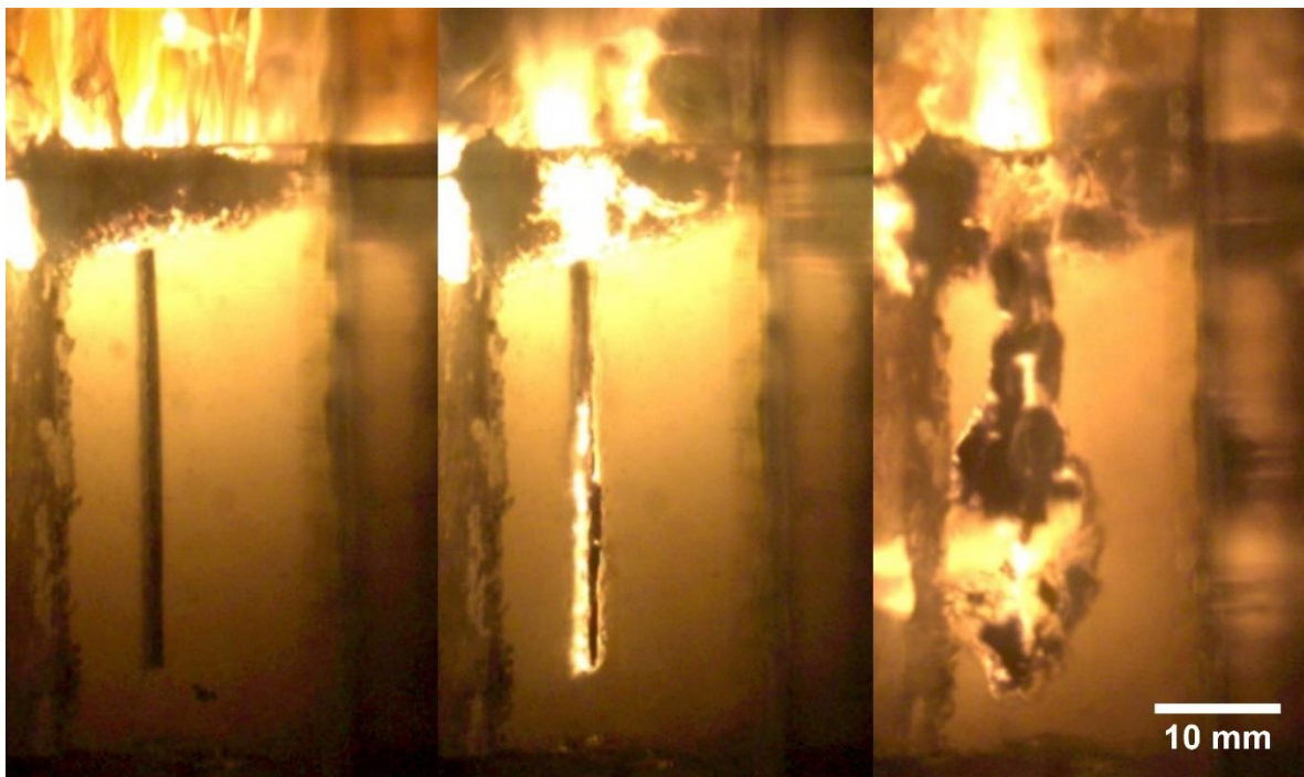
Figure G-4. Convective burning of Al/PVDF wire embedded in AP/HTPB propellant at 1.38 MPa. There are 0.1 s between frames.
