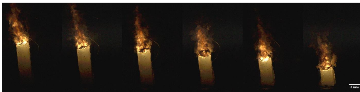
Figure 6-3. Layered printed propellant burning at 10.34 MPa with 29 ms in between frames. Outer layers are monomodal 60-130 \mu\text{m} AP/HTPB propellant and the middle layer is bimodal 90 \mu\text{m} and 60-130 \mu\text{m} AP/HTPB propellant (CFR 1:1). After flat ignition, a curved burning surface develops [45].
