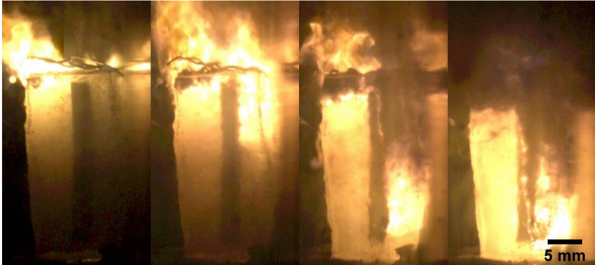
Figure G-12. Convective burning of Al/PVDF printed component embedded in AP/HTPB propellant at 3.45 MPa. There are 0.1 s between frames.
