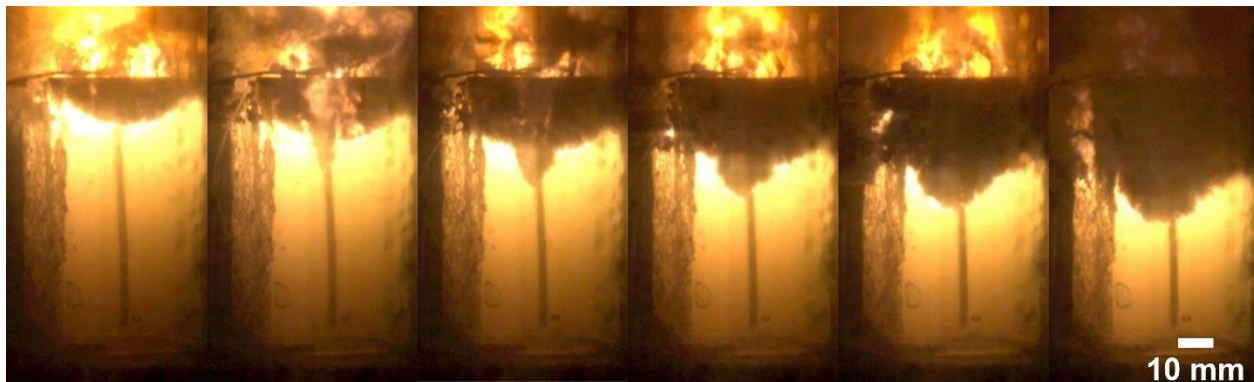
Figure G-10. Partial convective burning of Al/PVDF wire embedded in AP/HTPB propellant at 10.34 MPa. There are 0.1 s between frames.
