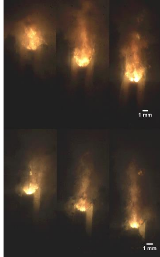
Figure 6-8. (Top) LFeOCP and (bottom) LnAlCP strands burning at 10.34 MPa with 116 ms in between frames. Even after flat ignition, a curved burning surface develops.
