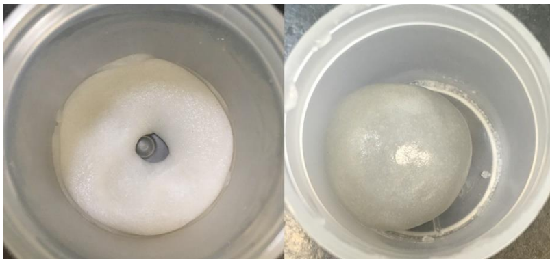
Figure H-3. Comparison of fresh propellant mixtures made via (left) Flacktek and (right) Resodyn mixers.
