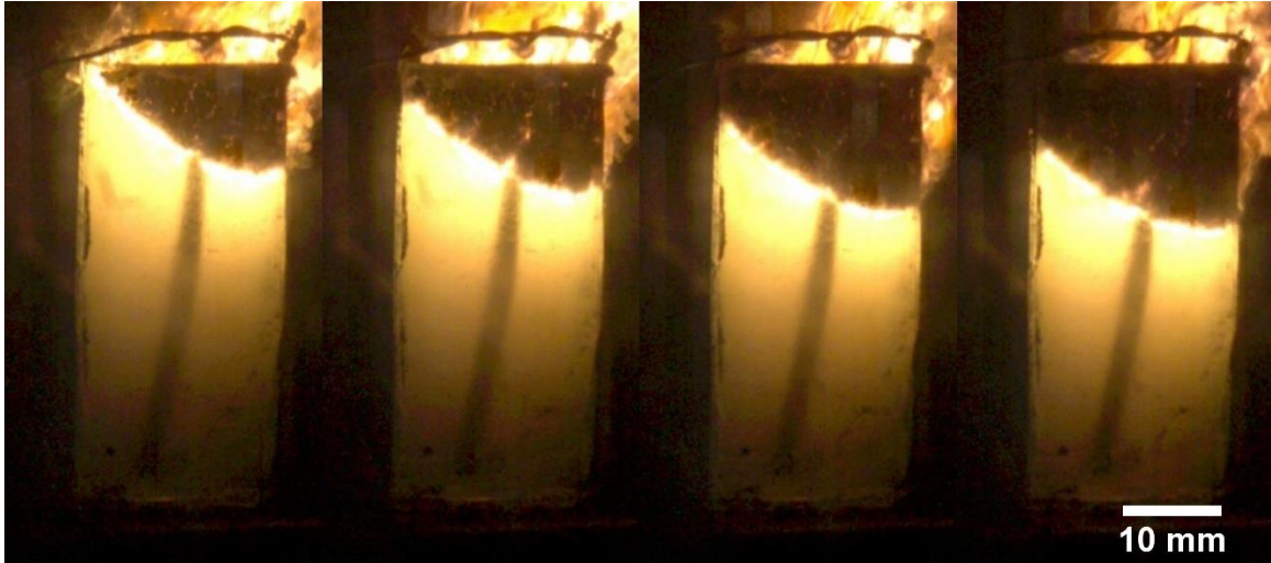
Figure G-7. Conductive burning of Al/PVDF wire embedded in AP/HTPB propellant at 6.89 MPa. There are 0.1 s between frames.
