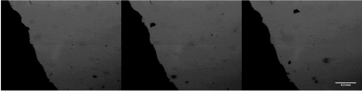
Figure I-4. Near surface combustion of propellant with the 3Al:Zr additive at atmospheric conditions. There is 0.1 ms between the frames and no surface reactions are seen.
