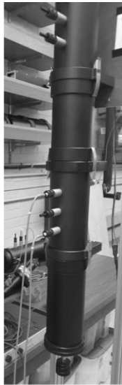
(a) Standing Wave Tube (Type 4206 Large tube)
