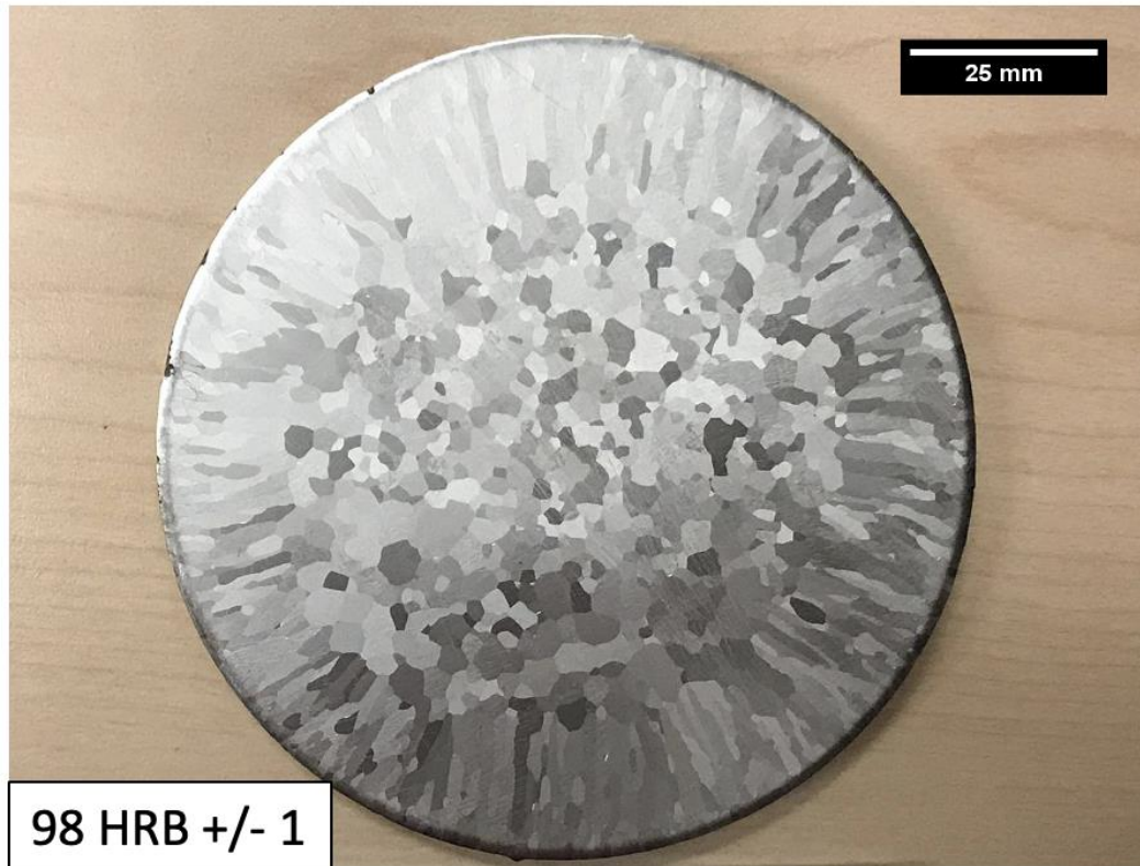
Figure 42 Fe-4Si-4Cr ingot cross section in the as-cast microstructure and hardness.
