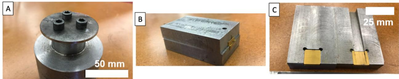
Figure 23 FM/HCE set up. A) Rotating workpiece assembled to a mandrel B & C) Insert cutting tools assembled to the holders in two different positions.
