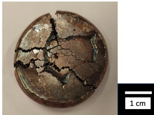
Figure 22 Fe-6.5Si wt% sample failing after only 5% reduction during hot rolling.
