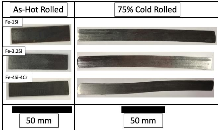
Figure 21 Workability test results after 75% cold work reduction. Graph reports results for Fe-1Si, Fe-3.2Si, and Fe-4Si-4Cr alloys.
