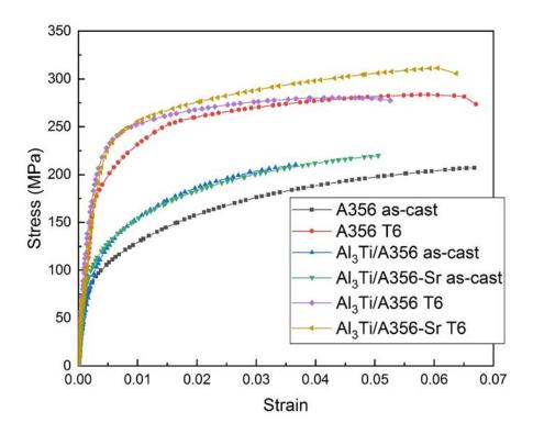
Figure 4.5. Stress-strain curves of A356 and Al<sub>3</sub>Ti/A356 composites
