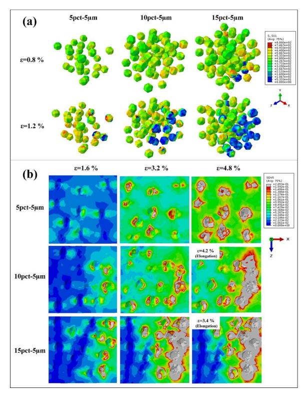
Figure 6.10. (a) S11 stress component distributions on the Al<sub>3</sub>Ti particles at different nominal strains of 5, 10, and 15pct-5 $\mu$ m RVEs; (b) The matrix damage parameter  $D_{\eta}$  distribution at different nominal strains of these three RVEs.
