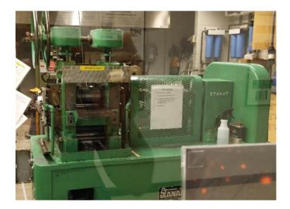
Figure 3.1. The laboratory rolling mill for rolling process.
