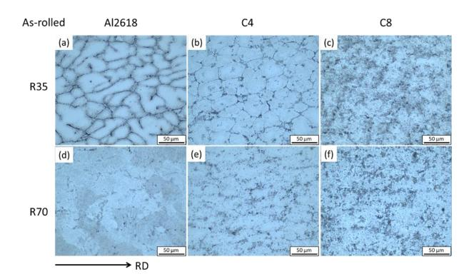
Figure 7.2. OM images of the as-rolled Al2618 alloy and TiB<sub>2</sub>/Al2618 composites taken from RD-TD plane (a) Al2618-R35, (b) C4-R35, (c) C8-R35; (d) Al2618-R70; (e) C4-R70; and (f) C8-R70.
