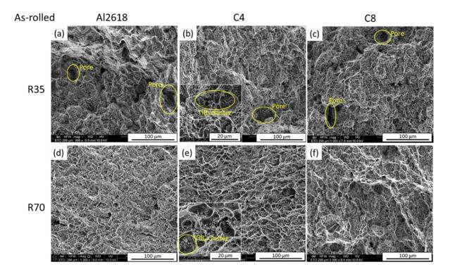
Figure 7.9. Typical fracture surfaces of the as-rolled Al2618 alloy and TiB<sub>2</sub>/Al2618 composites; (a) Al2618-R35, (b) C4-R35, (c) C8-R35; (d) Al2618-R70; (e) C4-R70; and (f) C8-R70.
