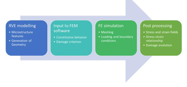
Figure 2.5. Flow chart showing typical procedure for micromechanical simulations on the microstructure-based RVE by FEM.
