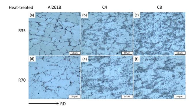
Figure 7.4. OM images of the heat-treated Al2618 alloy and TiB<sub>2</sub>/Al2618 composites (a) Al2618-R35, (b) C4-R35, (c) C8-R35; (d) Al2618-R70; (e) C4-R70; and (f) C8-R70.
