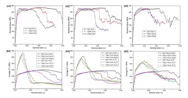
Figure 6.9. (a1)~(a3) The simulation stress-strain curves of of 5, 10, and 15pct-5µm RVEs, respectively. (b1)~(b3) The average S11 stress component of Al<sub>3</sub>Ti and A356 matrix phases corresponding to the RVEs in Figs. 6.9(a1)~(a3), respectively.
