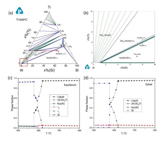
Figure 5.6. (a) A calculated isothermal section of Al-Si-Ti ternary system at 540 °C; (b) Magnified red rectangular area in the Al-rich corner in figure (a); (c) and (d) The evolution of phase fractions in the Al-7.10 at. % Si-1.34 at. % Ti alloy simulated under equilibrium condition and Scheil condition, respectively.
