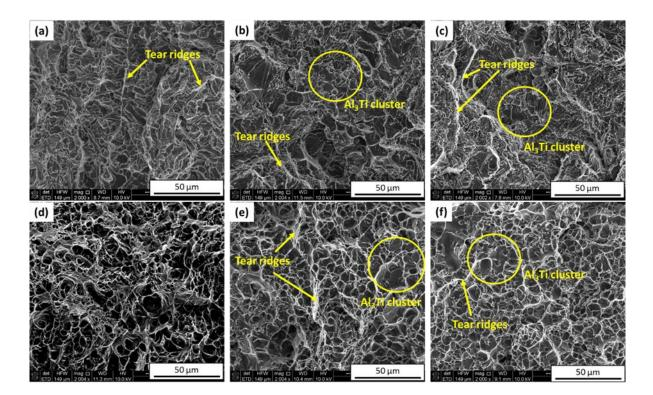
Figure 4.6. Typical fracture surface of as-cast (a) A356 alloy, (b) Al<sub>3</sub>Ti/A356 and (c) Al<sub>3</sub>Ti/A356-Sr composites; and T6 treated (d) A356, (e) Al<sub>3</sub>Ti/A356 and (f) Al<sub>3</sub>Ti/A356-Sr composites.
