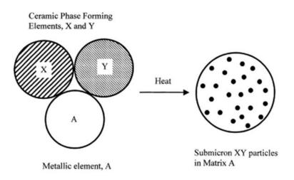
Figure 2.2. Schematic figure for the fabrication XD dispersion-hardened composites. (S. Tjong & Ma, 2000)
