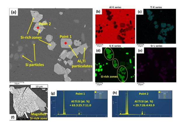
Figure 4.4. EDS analysis of a T6 treated Al<sub>3</sub>Ti/A356-Sr sample (a) Back scattered electron image with an inserted image shows the magnified structure of Si-rich zone); (b)~(e) Elemental mapping of Al, Ti, Si and Sr, respectively; (f) a magnified SEM image showing the structure of a Si-rich zone; (g) and (h) spectra of point 1 and point 2 in figure (a), respectively.
