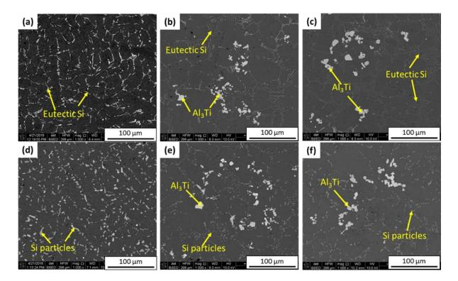
Figure 4.1. Backscattered electron images of as-cast (a) A356 alloy, (b) Al<sub>3</sub>Ti/A356 and (c) Al<sub>3</sub>Ti/A356-Sr composites; and T6 treated (d) A356, (e) Al<sub>3</sub>Ti/A356 and (f) Al<sub>3</sub>Ti/A356-Sr composites.
