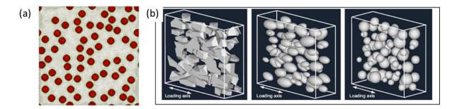
Figure 2.4. (a) 2D multi-particle RVE model with round inclusions (Qing, 2013b); (b) 3D multiparticle RVE models with different particle morphology (Chawla et al., 2006).
