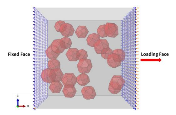
Figure 6.4. Schematic image of loading and boundary conditions on the 3D RVEs.
