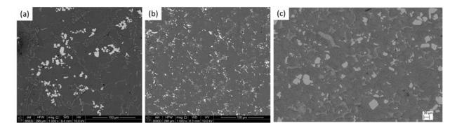
Figure 2.1. Microstructure of (a) Al<sub>3</sub>Ti/A356 composite (S. Ma & Wang, 2019); (b) TiB<sub>2</sub>/Al2618 composite (S. Ma et al., 2020); (c) Al-5Ti-1B master alloy with TiB<sub>2</sub> at the α-Al grain boundaries and Al<sub>3</sub>Ti in a-Al grain centers (X. Wang et al., 2015).
