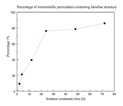
Figure 5.2. Percentage of intermetallic particulates containing lamellar structure in the Al-Si-Ti alloy after different solution treatment time.
