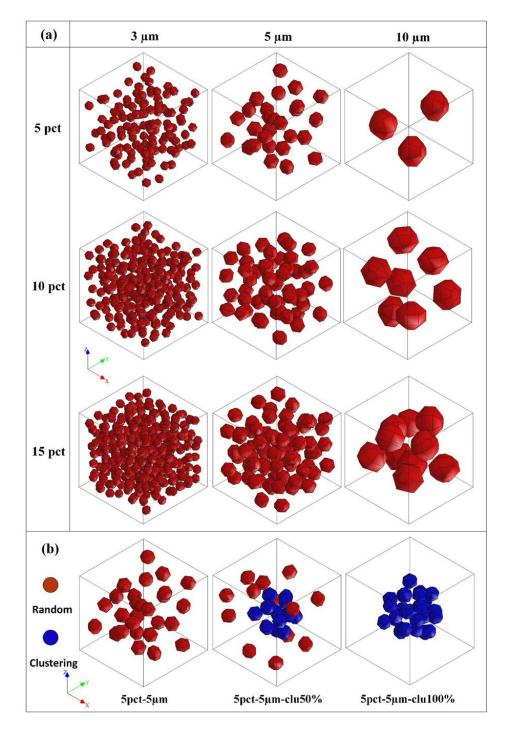
Figure 6.2. (a) Examples of 3D automatically generated RVEs containing randomly distributed Al<sub>3</sub>Ti particles with various sizes and volume fractions. (b) 5pct-5µm RVEs with random distribution, 50 % particle clustering, and 100 % particle clustering. (The edge length of all the RVEs in this figure is 30 µm)
