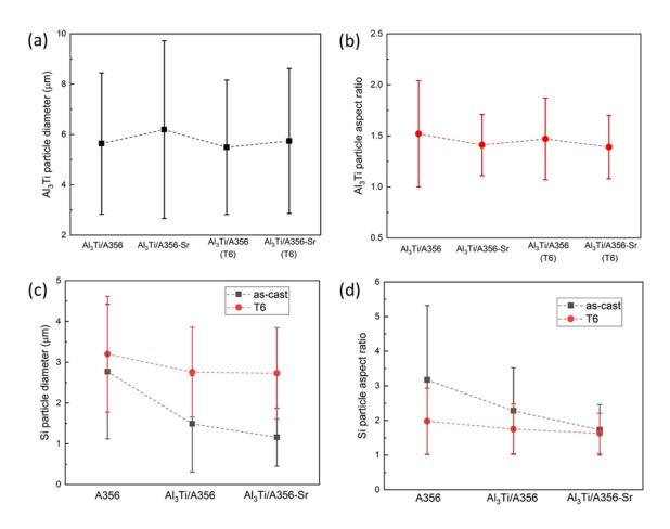
Figure 4.2. Statistics of (a) average particle diameter and (b) average aspect ratio of Al<sub>3</sub>Ti particles; (c) average particle diameter and (d) average aspect ratio of Si particles in different samples.
