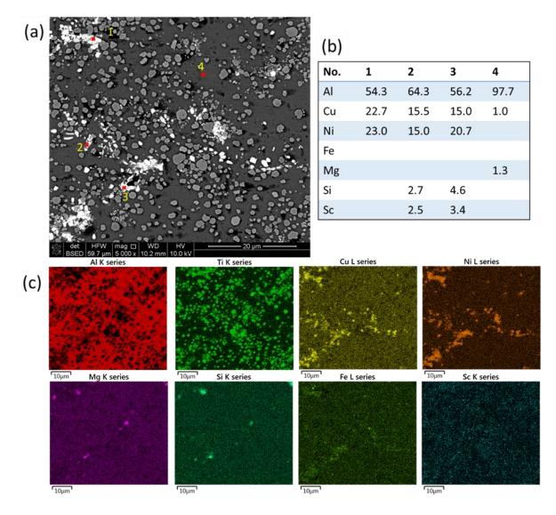
Figure 7.6. EDS analysis of heat-treated TiB<sub>2</sub>/Al2618 composite (C8-R60 sample) (a) Electron image; (b) Elemental composition from the point analysis in figure (a) (in at. %); (c) Elemental mapping.
