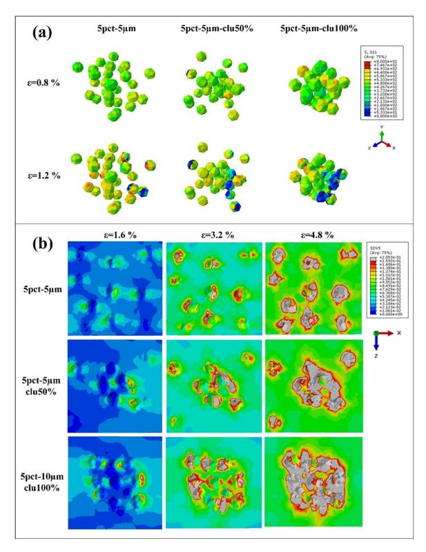
Figure 6.12. (a) S11 stress component distributions on the Al<sub>3</sub>Ti particles at different nominal strains of 5pct-5 $\mu$ m, 5pct-5 $\mu$ m-clu50% and 5pct-5 $\mu$ m-clu100% RVEs; (b) The matrix damage parameter  $D_{\eta}$  distribution at different nominal strains of these three RVEs.
