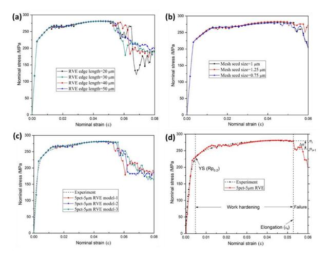
Figure 6.6. Effect of (a) the selected RVE edge length; (b) mesh density; and (c) model variation on the simulation nominal stress strain curves; (d) comparison between the nominal stress-strain curves from 5pct-5µm RVE and from experimental uniaxial tensile test.
