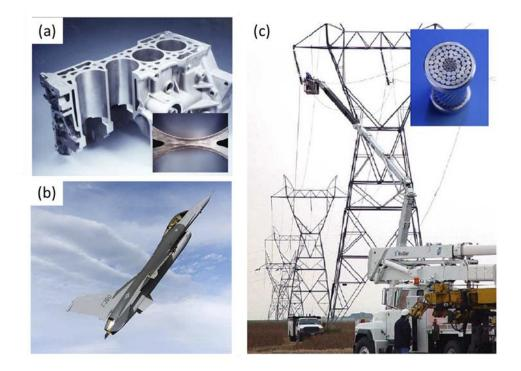
Figure 1.1. Examples of applications of AMCs in industries. (a) Honda Prelude 2.01-cylinder block (Donaldson Steven L & Miracle Daniel B, 2001); (b) F-16 illustrating ventral fins on the bottom of the fuselage aft (rearward) of the wings (Donaldson Steven & Miracle Daniel, 2001); (c) Conductor cables of power transmission towers (Miracle, 2005).
