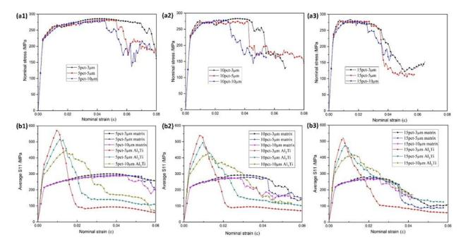
Figure 6.7. (a1)~(a3) simulation stress-strain curves of 5pct-3, 5, and 10µm RVEs, respectively. (b1)~(b3) the average S11 stress component of Al<sub>3</sub>Ti and A356 matrix phases corresponding to the RVEs in Figs. 6.7(a1)~(a3), respectively.
