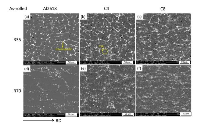
Figure 7.3. BSE images of the as-rolled Al2618 alloy and TiB<sub>2</sub>/Al2618 composites taken from RD-TD plane (a) Al2618-R35, (b) C4-R35, (c) C8-R35; (d) Al2618-R70; (e) C4-R70; and (f) C8-R70.
