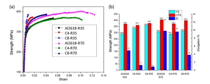
Figure 7.8. Uniaxial tensile properties of the heat-treated Al2618 and TiB<sub>2</sub>/Al2618 composites; (a) Tensile stress-strain curves; (b) Statistical histogram.
