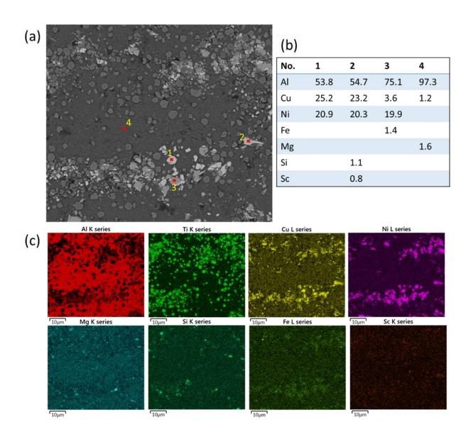
Figure 7.5. EDS analysis of as-rolled TiB<sub>2</sub>/Al2618 composite (C8-R70 sample) (a) Electron image; (b) Elemental composition from the point analysis in figure (a) (in at. %); (c) Elemental mapping.
