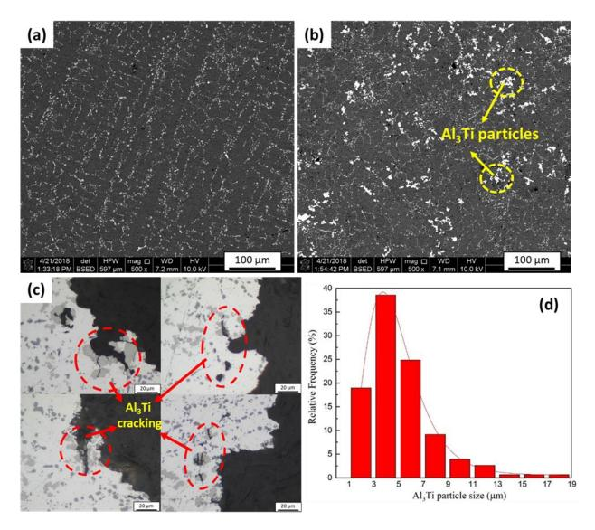
Figure 6.1. Backscattered electron images showing typical microstructure of (a) T6-A356 matrix and (b) T6-Al<sub>3</sub>Ti/A356 composite in this work; (c) Optical images showing four typical areas near the fracture surface of the Al<sub>3</sub>Ti/A356 composite after tensile test; (d) Particle size distribution of Al<sub>3</sub>Ti in the Al<sub>3</sub>Ti/A356 composite.
