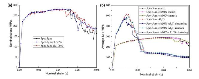
Figure 6.11. (a) Simulation stress-strain curves of 5pct-5μm, 5pct-5μm-clu50% and 5pct-5μm-clu100% RVEs, respectively. (b) The average S11 stress component of Al<sub>3</sub>Ti and A356 matrix phases corresponding to the RVEs in Figure 6.11(a), respectively.
