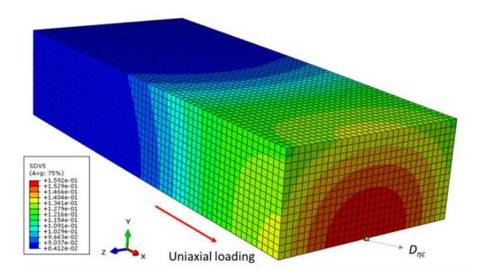
Figure 6.3. The critical value  $D_{\eta c}$  of the T6-A356 matrix determined by uniaxial tensile simulation. (SDV5 in the legend refers to  $D_{\eta}$ )
