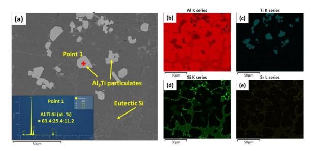
Figure 4.3. EDS analyses of as-cast Al<sub>3</sub>Ti/A356-Sr composite (a) Back scattered electron image with an inserted EDS spectrum from point 1 on an Al<sub>3</sub>Ti particle; (b)~(e) Elemental mapping of Al, Ti, Si and Sr elements, respectively.
