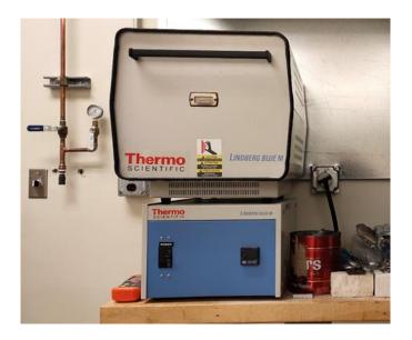
Figure 3.2. Heating oven for heat treatment of the samples.
