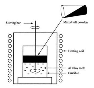
Figure 2.3. Schematic figure showing an apparatus of fabricating in-situ MMCs by flux-assisted synthesis. (S. Tjong & Ma, 2000)
