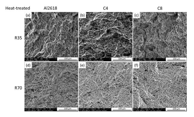
Figure 7.10. Typical fracture surfaces of the heat-treated Al2618 alloy and TiB<sub>2</sub>/Al2618 composites; (a) Al2618-R35, (b) C4-R35, (c) C8-R35; (d) Al2618-R70; (e) C4-R70; and (f) C8-R70.
