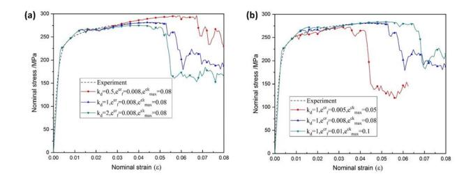
Figure 6.5. Effect of (a) the parameter  $k_d$  and (b)  $e_f^{cr}$  and  $e_{max}^{ck}$  on the obtained nominal stress-strain curves from RVE simulation.
