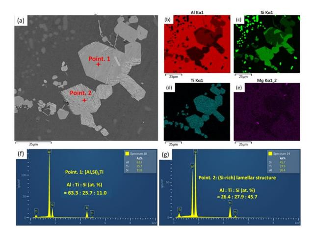
Figure 5.4. (a) Back-scattered electron image of the Al-Si-Ti alloy after 4 h solution treatment, with (b)~(e) EDS Elemental mapping of Al, Si, Ti and Mg elements, respectively, and (f)~(g) the EDS spectra from Point 1 on an intermetallic particulate and Point 2 on the lamellar structure in figure (a), respectively.
