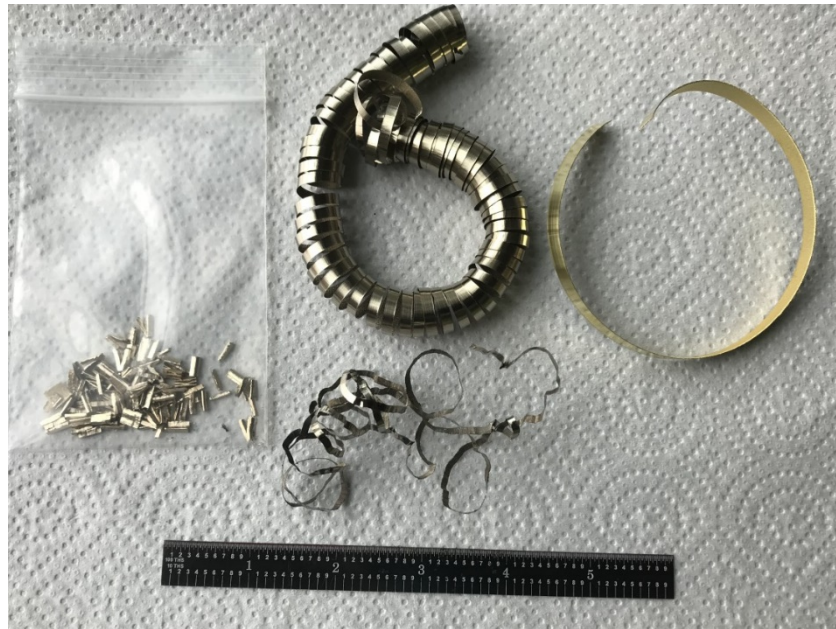
Fig. 2.3 An image showing chip types and shapes. Depending on material and cutting conditions, some chips are discrete, others are continuous with varying shapes including straight, coiled and helically wound shapes.
