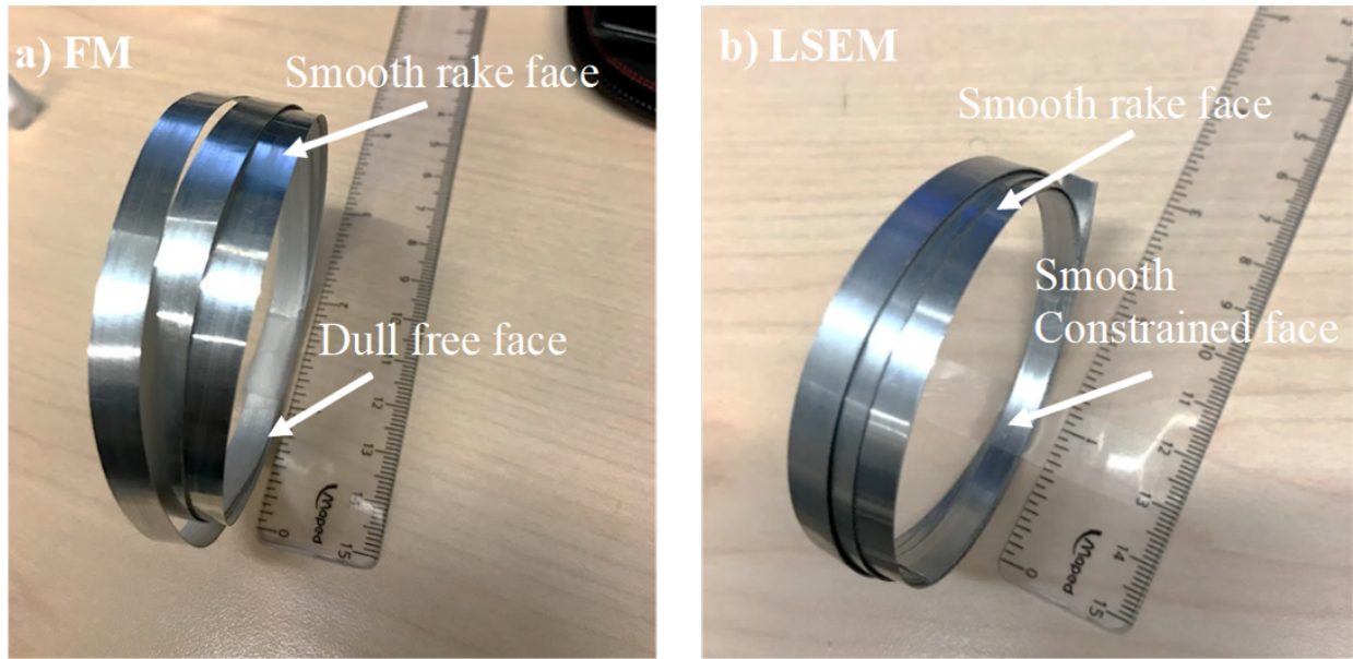
Fig. 5.6 Coils of Al 1100 chip produced by a) FM and b) HCE. The chips are intentionally coiled after the processing to show long samples.
