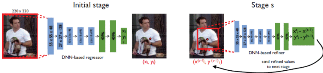
Figure 2.16: Deep pose Algorithm Architecture.
