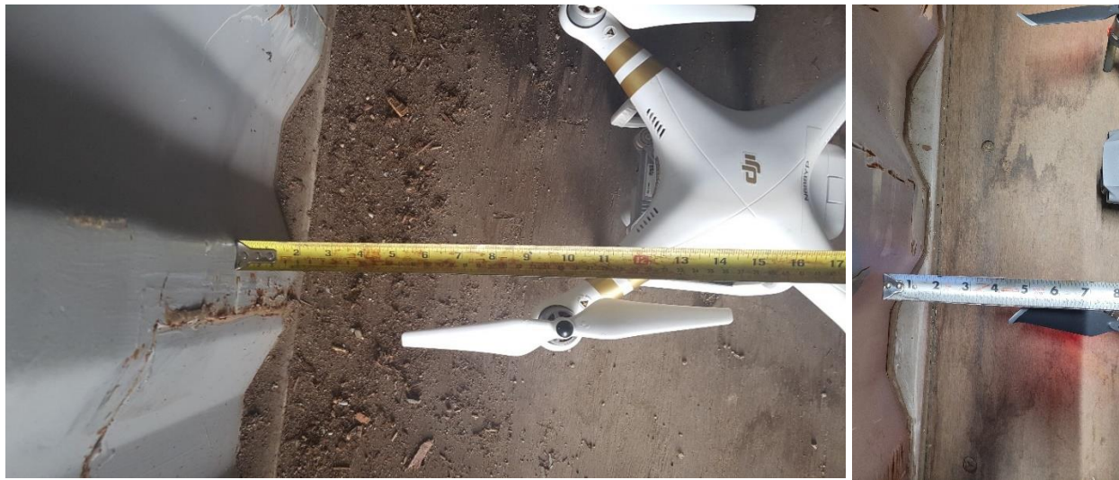
Figure 5 Distance where UAV performance will start to be affected by surrounding effect: 5 inches.
