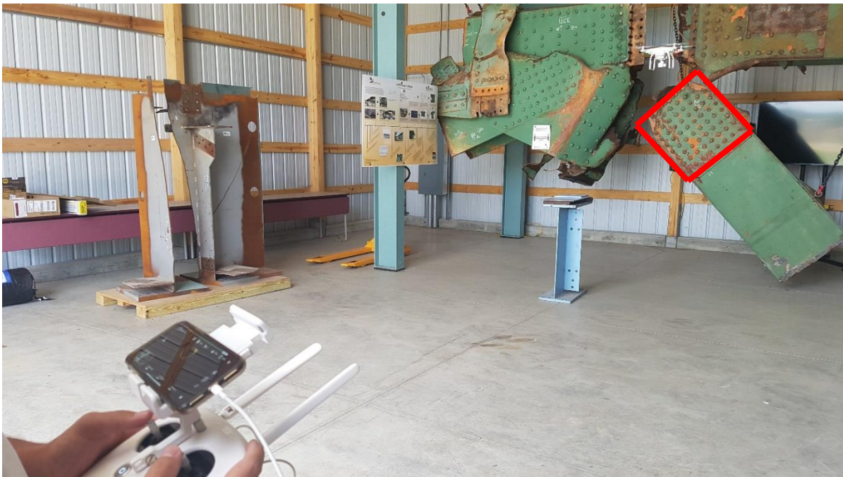
Figure 24 Inspection of I-35W Bridge elements at S-BRITE.
