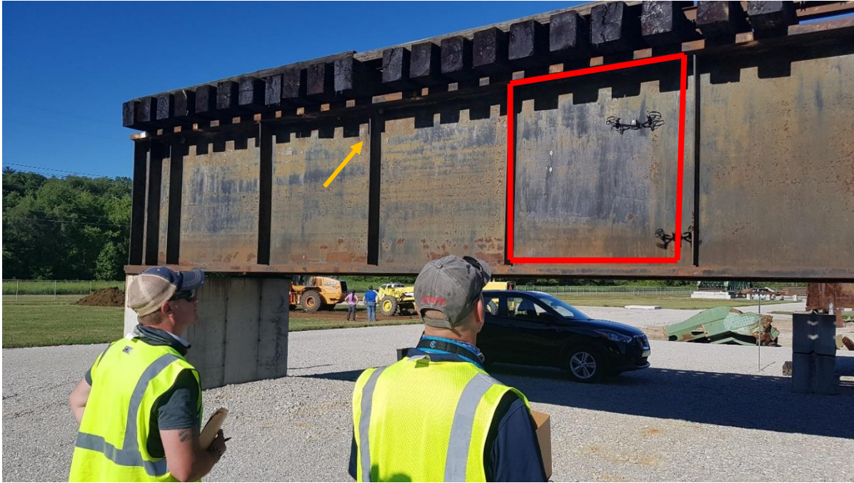
Figure 18 Inspection of welded bridge at S-BRITE.
