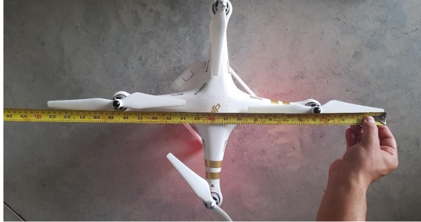
Figure 3 Process to measure Zone 1 around an UAV.
