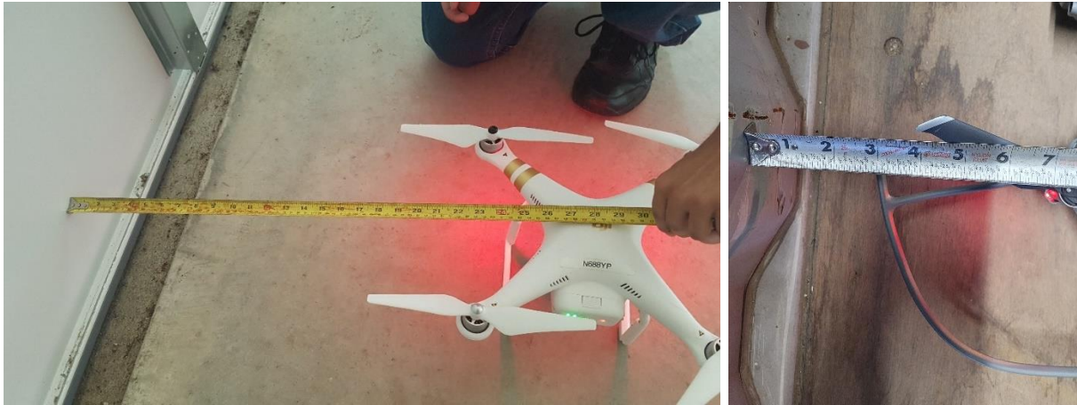
Figure 6 Delimitation of the end of Zone 2 around UAVs performed inside a shed and a cargo container at S-BRITE.
