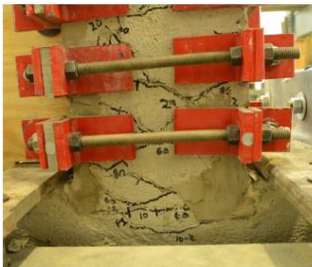
(a) North Column East Face, Repaired
