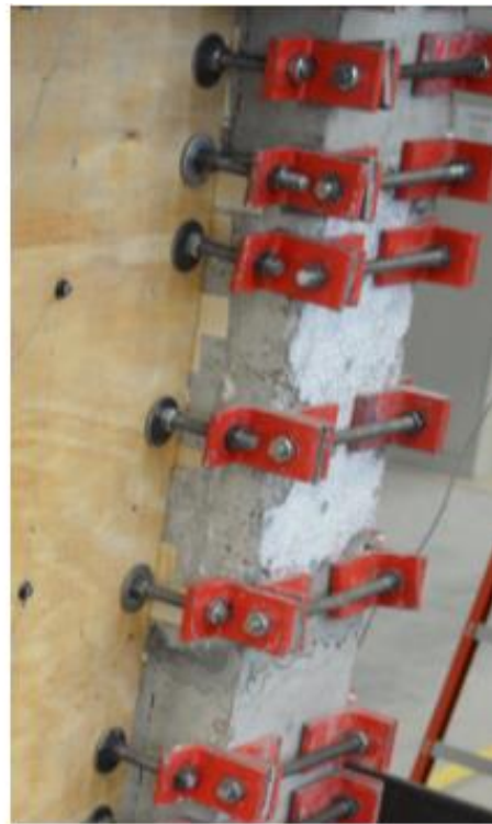
(b) Nuts used to adjust local infill position
