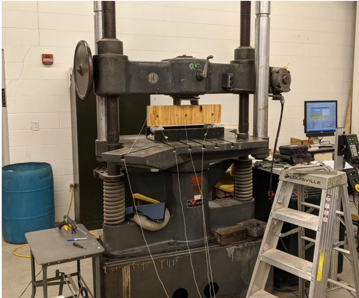
Figure A-23: Baldwin Southwark Tate-Emery Testing Machine with the Instron Extend Upgrade
