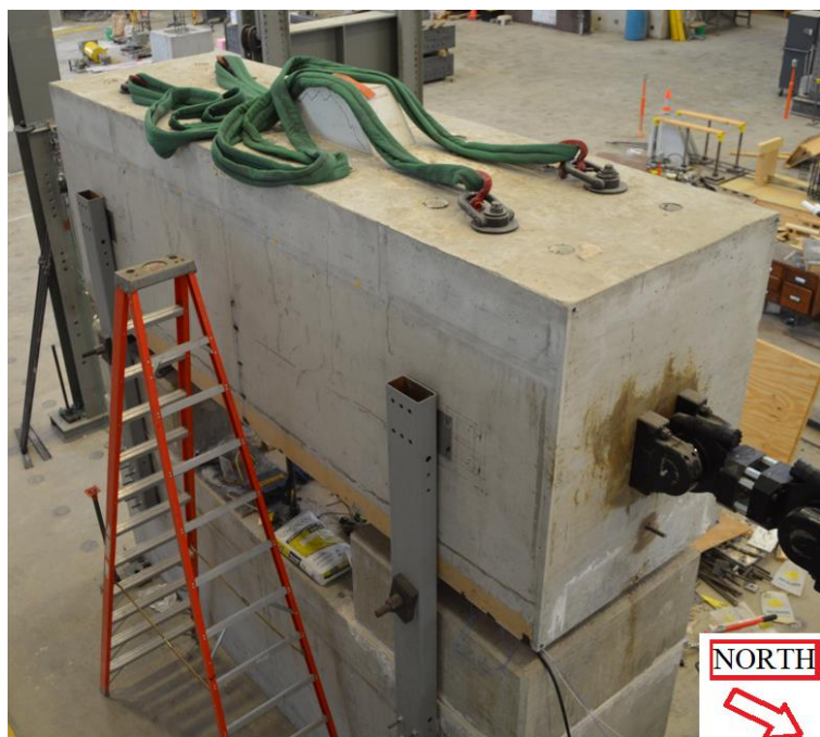
(a) External mass preparing for lift
