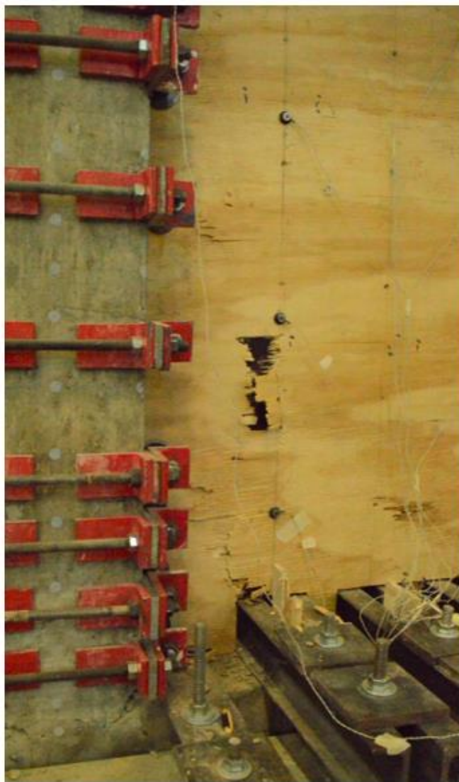
(a) North Edge Splitting, West Face
