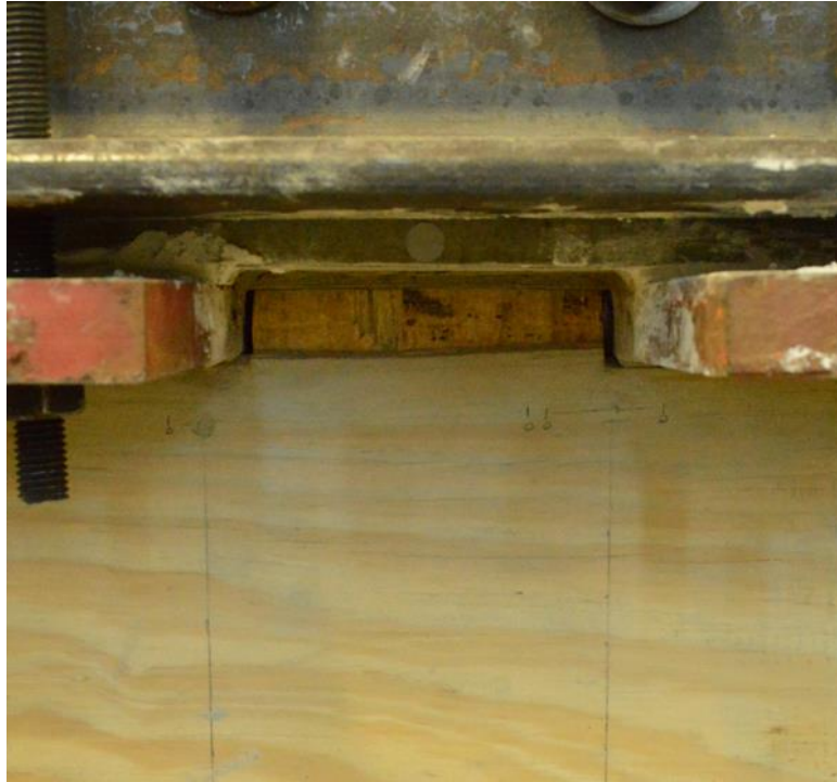
Figure 3-10: Single-ply Splitting at Infill Top, Western Face after Run 104 of Frame 2, Series F2-C-4PB
