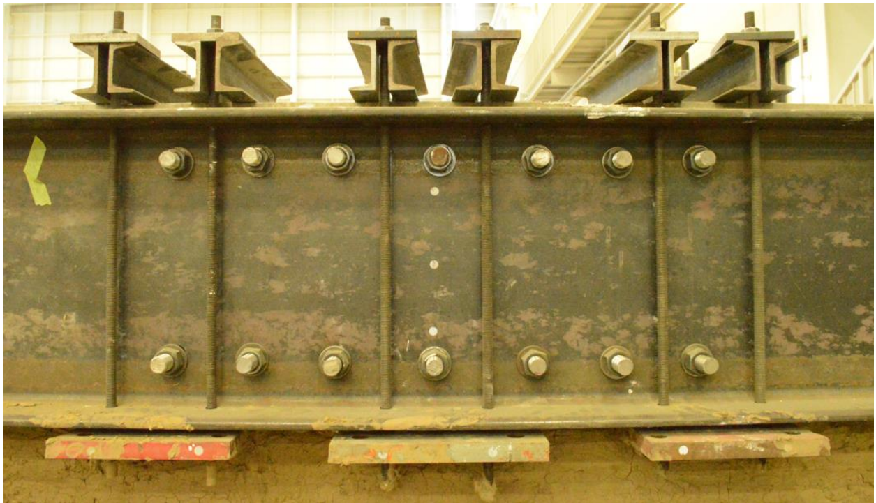
Figure A-17: Slip-critical Top Beam Connection and Vertical Clamping Devices (West Face)
