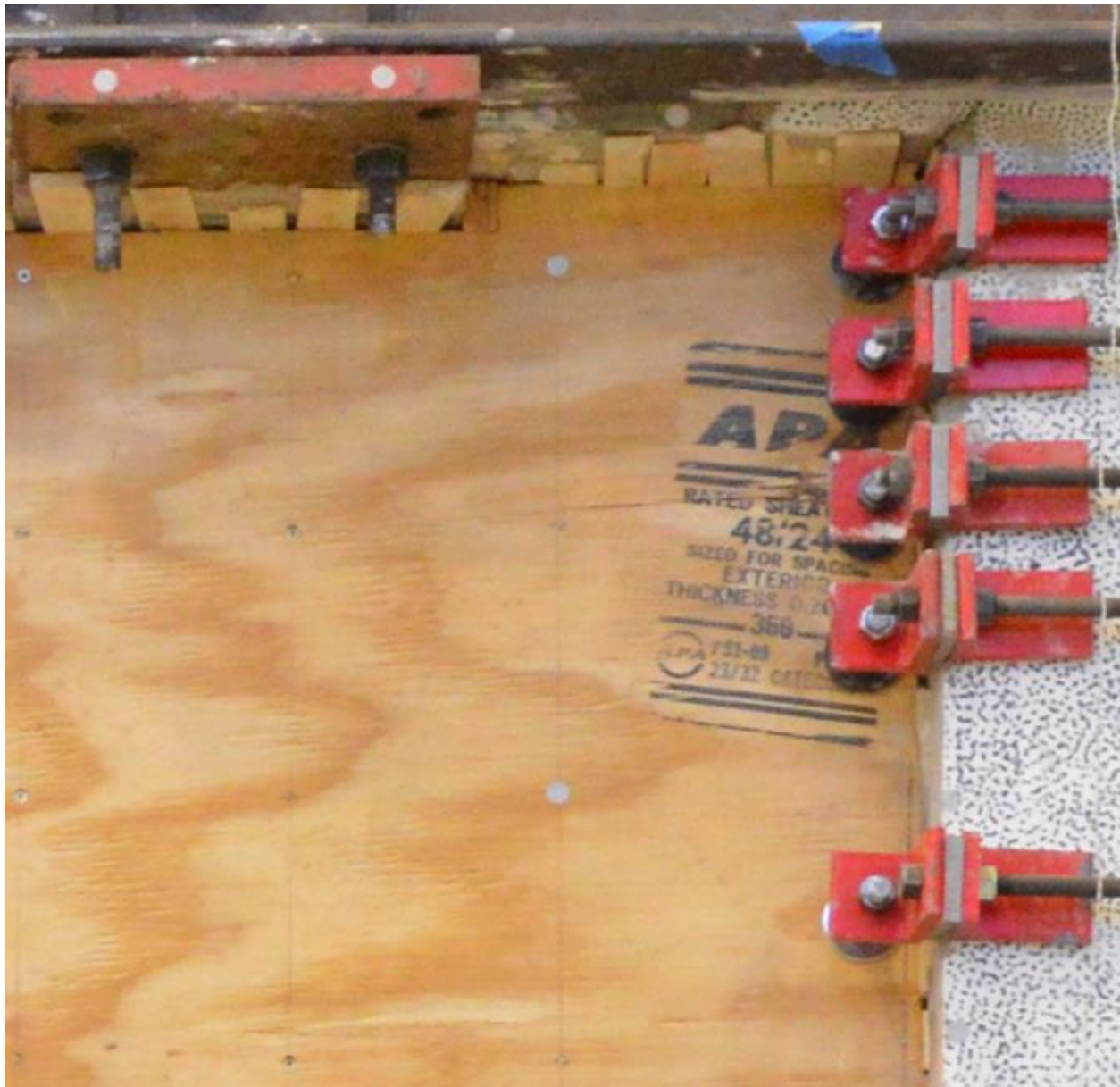
Figure 3-13: Shim Filled Edge Gap, Series F1-C-2PB
