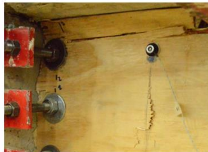
(c) North Edge Crushing, West Face Top
