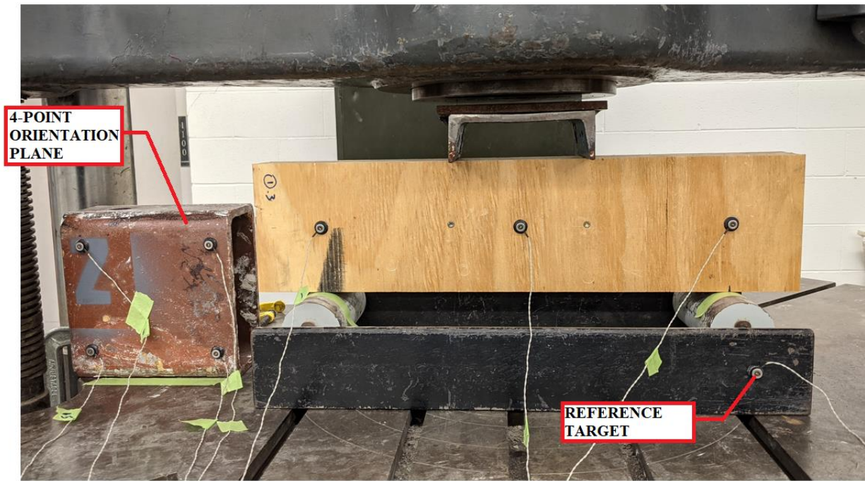
Figure 2-31: Modulus of Elasticity ( E_w ) Beam Test Setup
