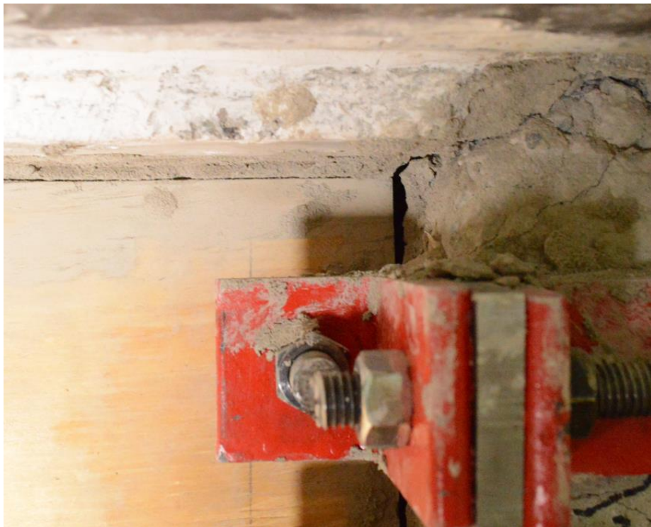
Figure 3-7: Mortar Edge-Joint after Deterioration during Series F2-C-4PB
