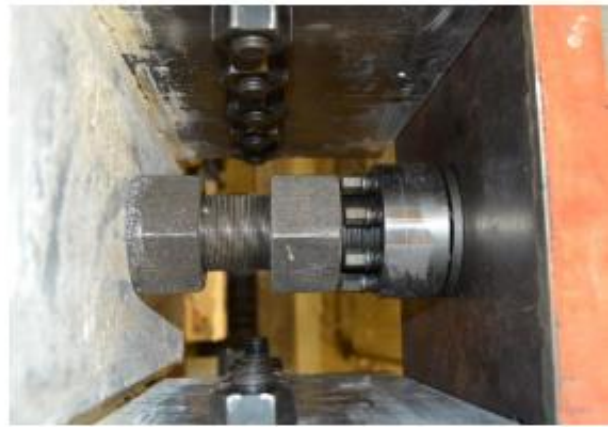
Figure A-18: Adjustable Bolts Preventing Slip between Confining Channels and Top Beam (Monical, 2022, Figure 2-16)
