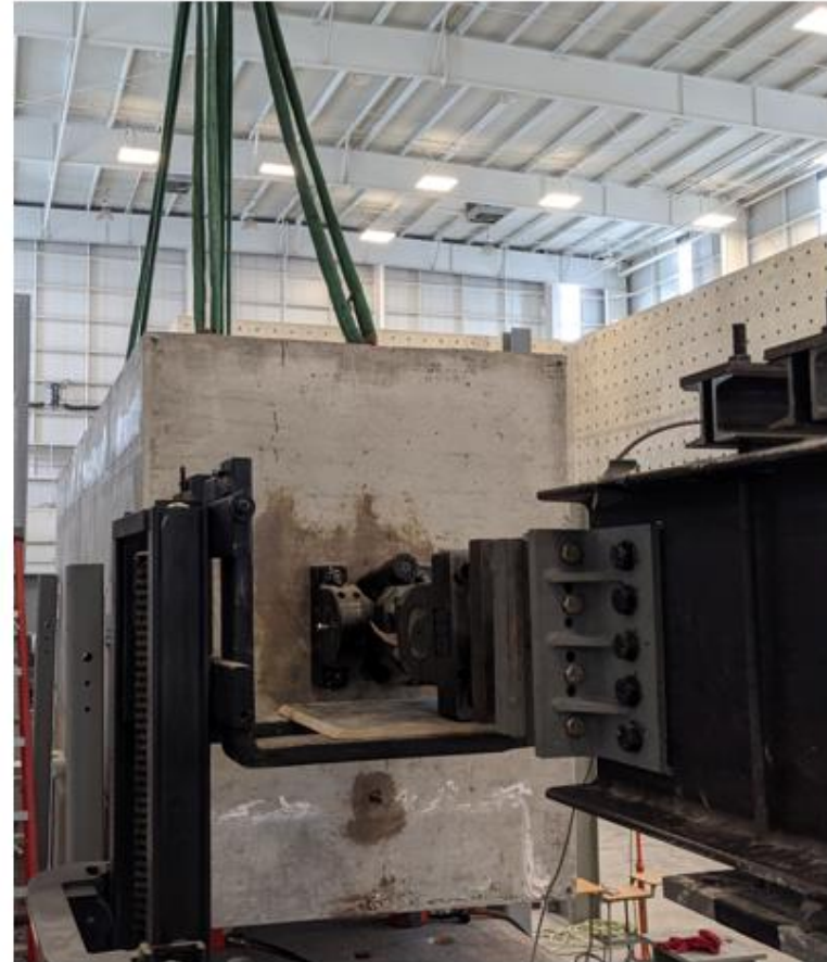
(3) Walkie-Stacker supports link, Crane lifts external mass. Spacer plates can now be inserted, and connection tightened
