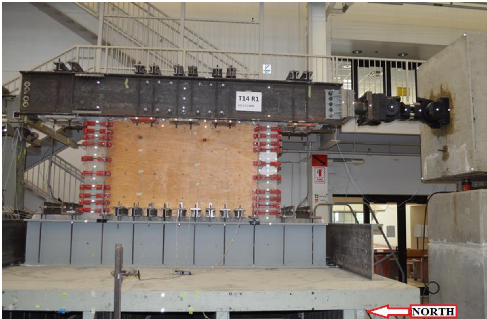
Figure 3-5: Frame Instrumented with Optitrack Target Layout B, Optotrack Layout B (Photograph)
