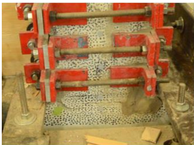
(b) South Column West Face, Repaired
