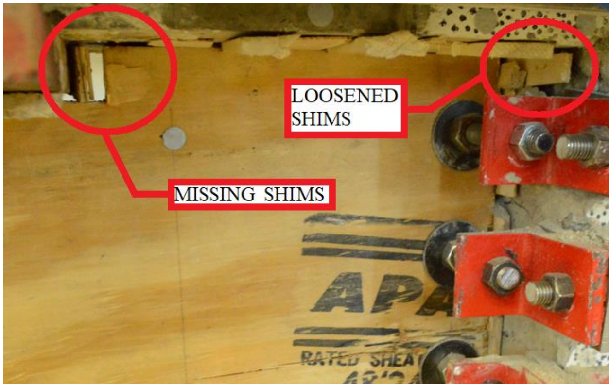
Figure 3-15: Deterioration of Shim Edge-Joint after Frame 1 Run 86, Series F1-C-2PB
