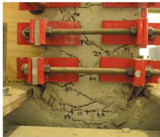
(c) North Column East Face after Frame 1 Run 108
