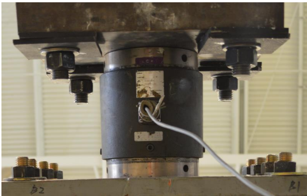
Figure B-4: Lebow 3156-100K Load Cell
