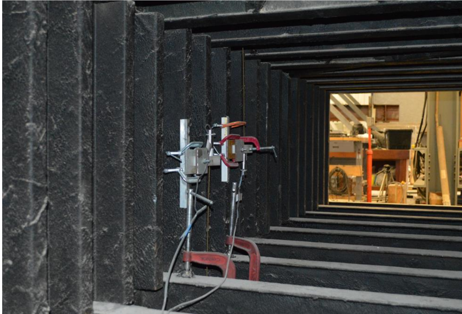
Figure 2-20: Simulator Platform LVDTs (North Pair)
