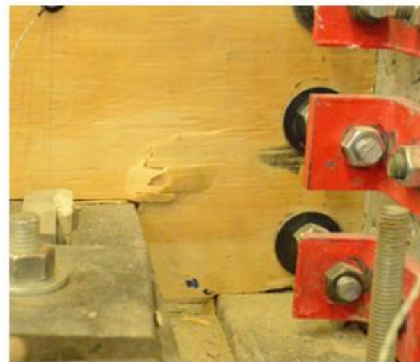
(b) South Edge Splitting, West Face Bottom
