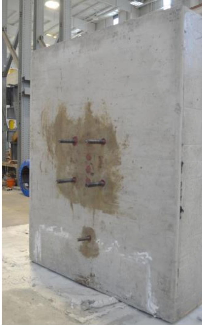
Figure A-21: Four 1-in. High-Strength Threaded Rods Embedded into North Face of External Suspended Mass (Monical, 2022, Figure B-24)
