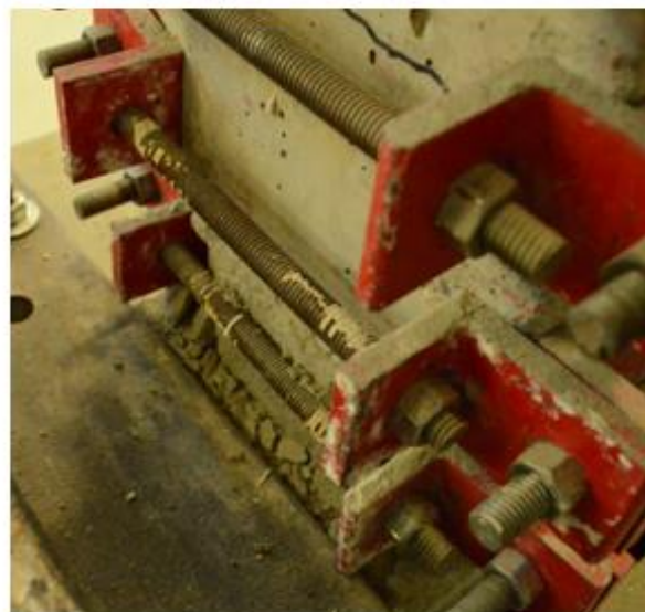
(c) South Column Base South Face Repair Mortar Spalling after Run 89
