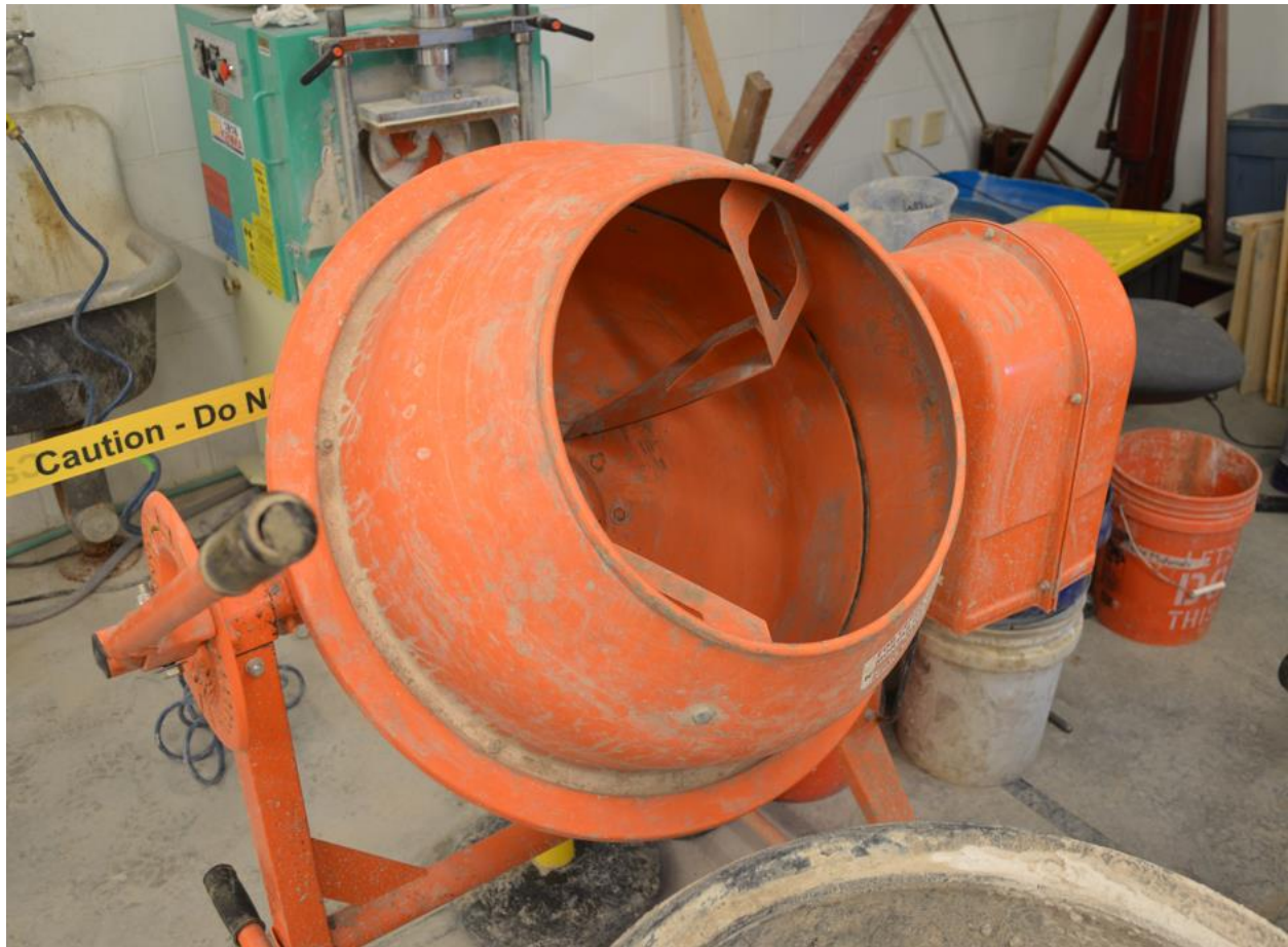
Figure A-1: Bowen Lab Concrete Mixer with 120lb, 3.5 Cubic Foot Capacity
