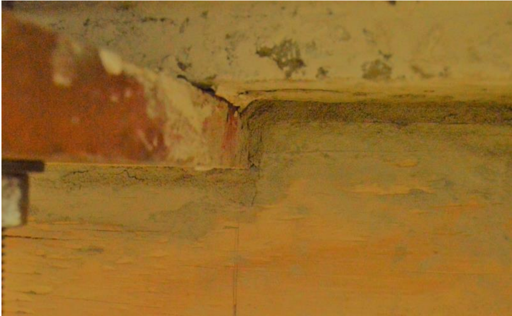
Figure 3-6: Mortar Edge-Joint Between Infill and Frame prior to Series F2-C-4PB
