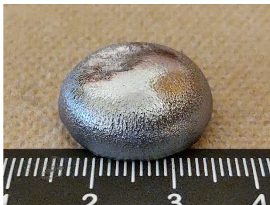
Figure 3-8 A typical ingot shape after fabrication. The shape, presence of a shrinkage cavity, and luster of the final product is relevant for data storage purposes.
