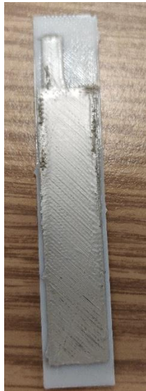
Figure 3.7 - Additively Manufactured Sensor Sample
