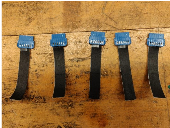
Figure 4.28 - ETPU initial samples back side post stretch test
