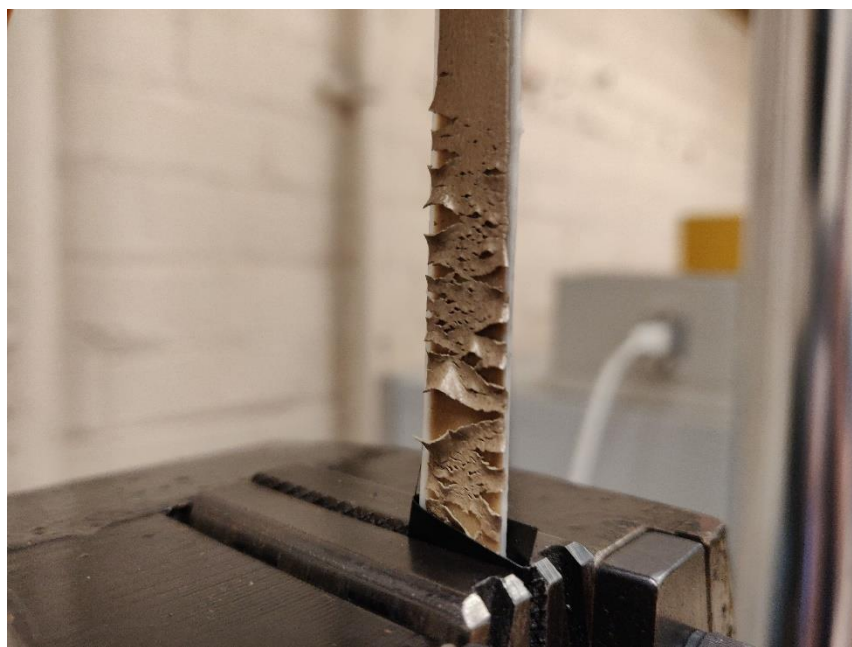
Figure 5.1 - Fluorine Rubber Ink Sample 2 during stretch testing
