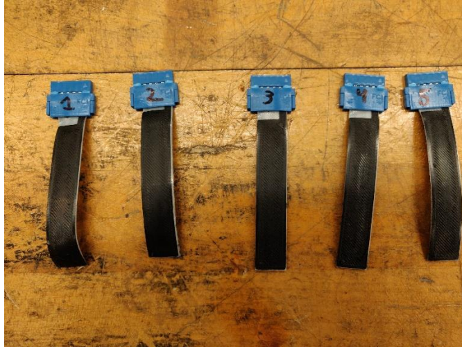
Figure 4.27 - ETPU initial samples front side post stretch test
