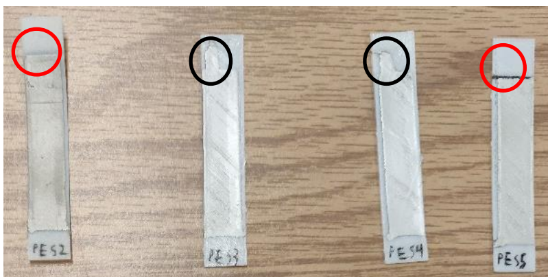
Figure 4.14 - Missing fingers for blue clips on PE873 Samples 2 & 5
