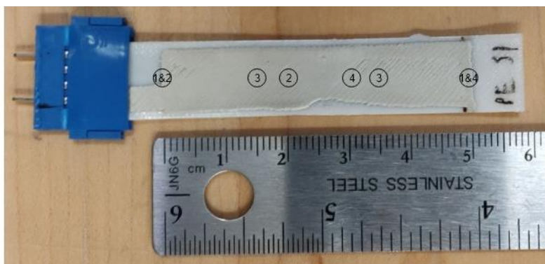
Figure 3.19 - Locations for resistance measurements for sensor samples
