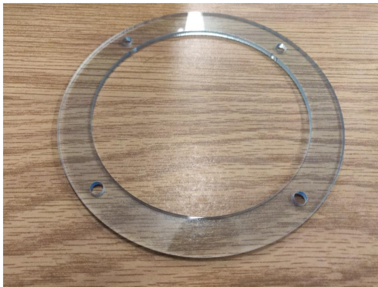
Figure 3.24 - Acrylic ring for holding strain on actuator samples
