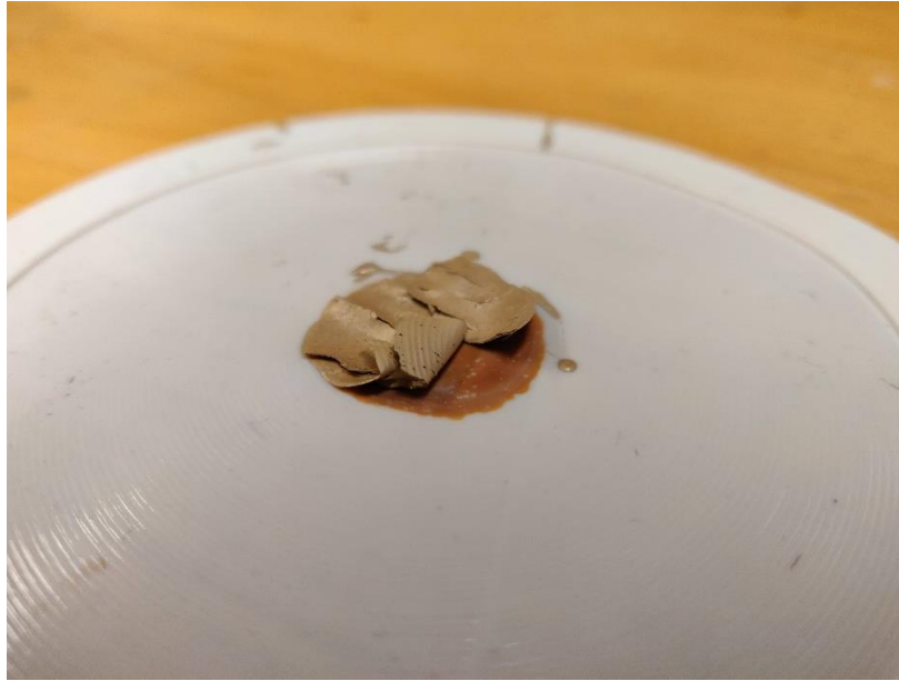
Figure 4.15 – Fluorine Rubber Ink actuator post additional annealing
