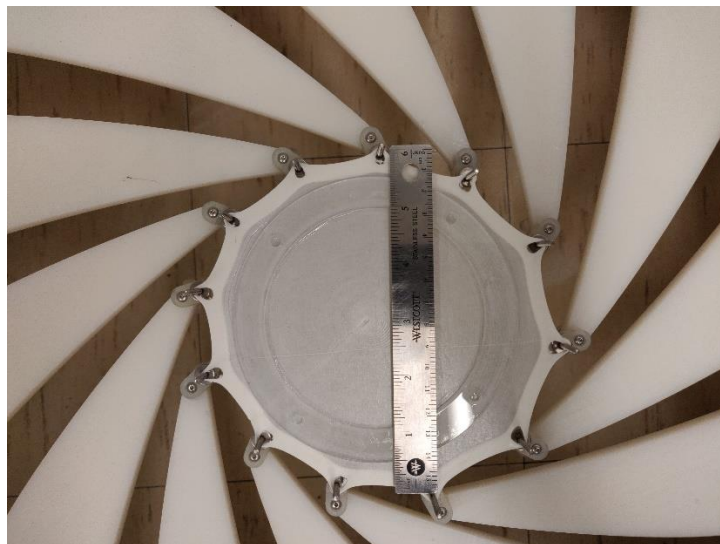
Figure 3.10 - Dielectric blank being strained on iris stretcher prior to actuation testing
