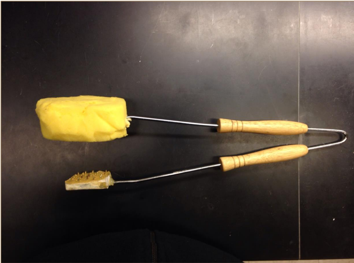
Figure 5.1. Modified inoculation device used in this study. The 5x5 grid of thumbtacks is used to injure corn leaves, while sponge simultaneously delivers inoculum.
