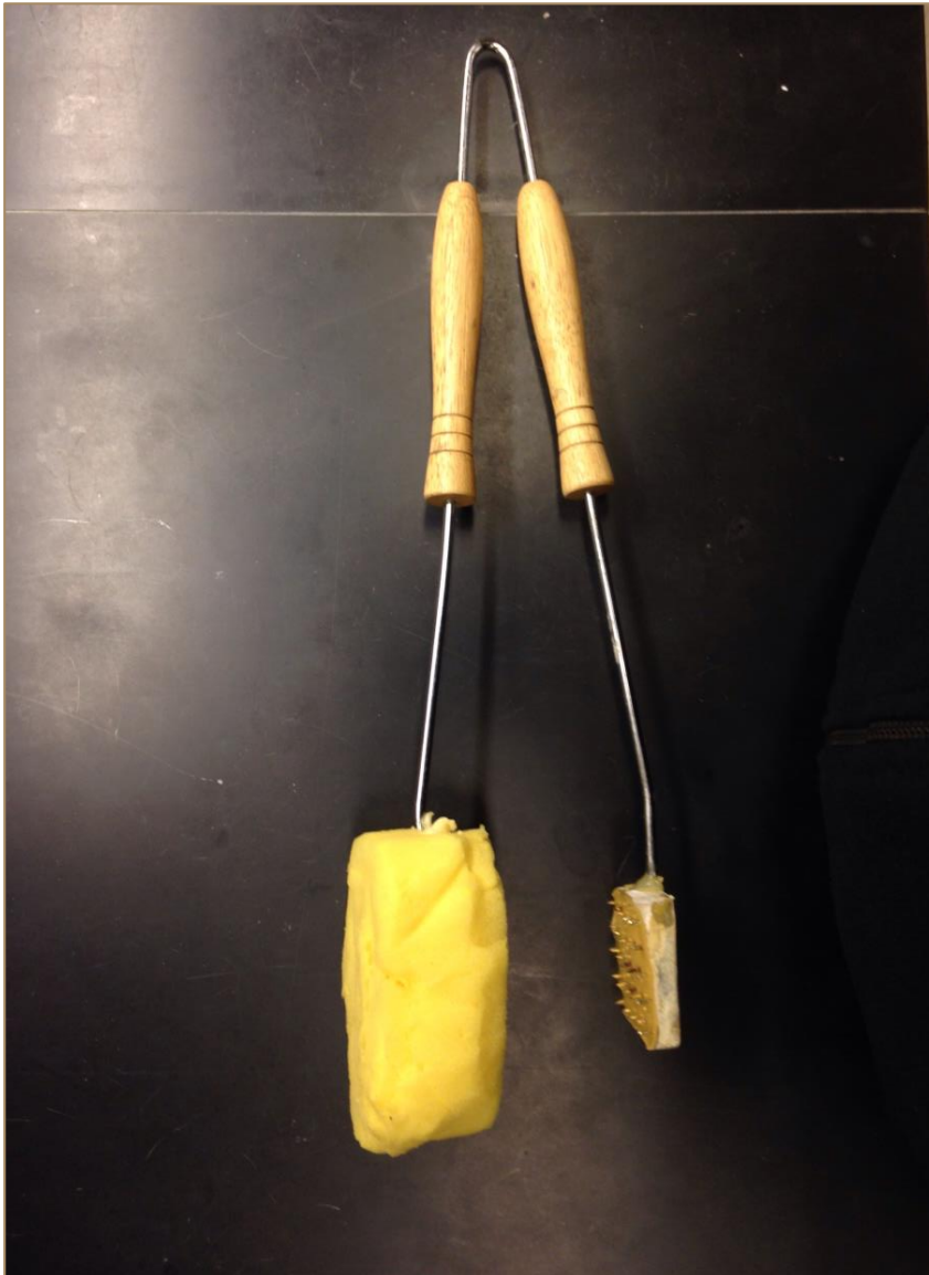
Figure 4.1. Modified inoculation device used in this study. The 5x5 grid of thumbtacks injures corn leaves, while sponge simultaneously delivers inoculum.
