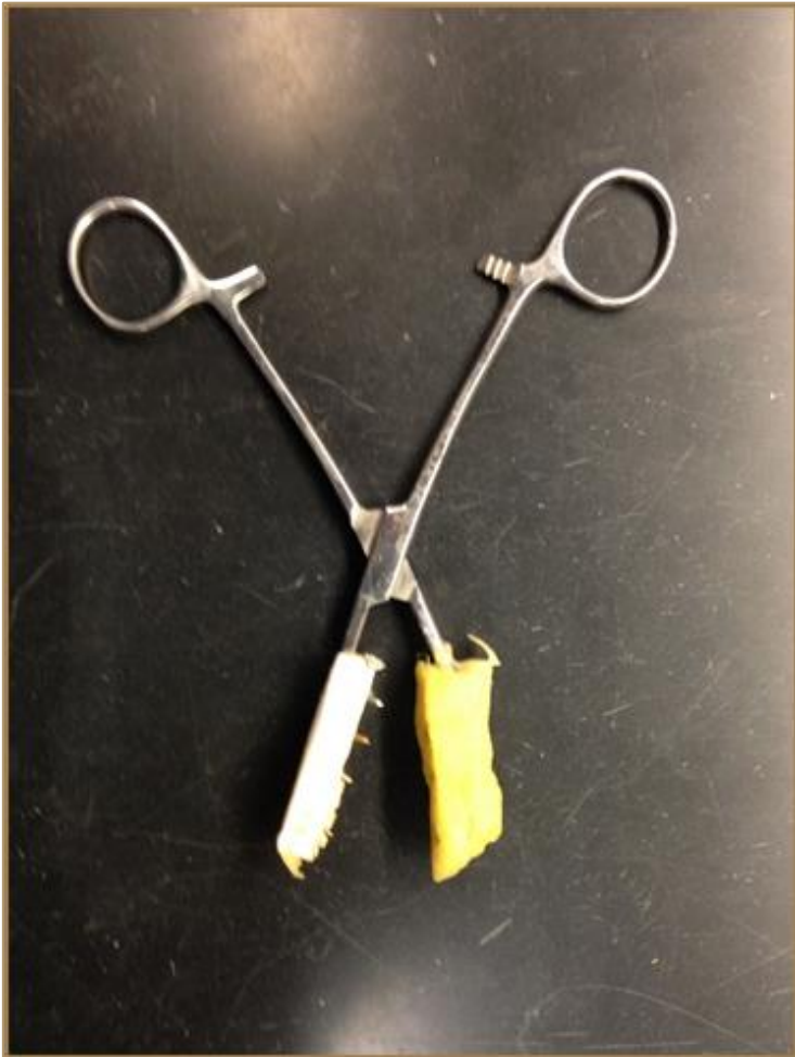
Figure 4.3. Modified inoculation device used in this study. The 5x1 grid of thumbtacks injures small leaves, while sponge simultaneously delivers inoculum.
