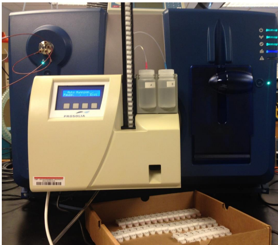
Figure 1.3 Commercial paper spray ion source sold by Prosolia. The cartridges stack in the center tower and are analyzed one at a time. The solvent and the potential are applied through the software and after the method is developed it is fully automated.
