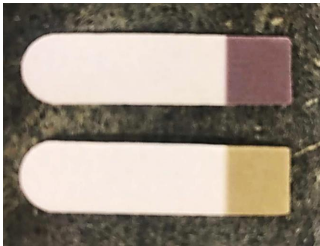
Figure 1.10 Commercial pSERS substrate. The top pSERS substrate has gold nanoparticles inkjet printed onto it and the bottom has silver nanoparticles inkjet printed onto it.
