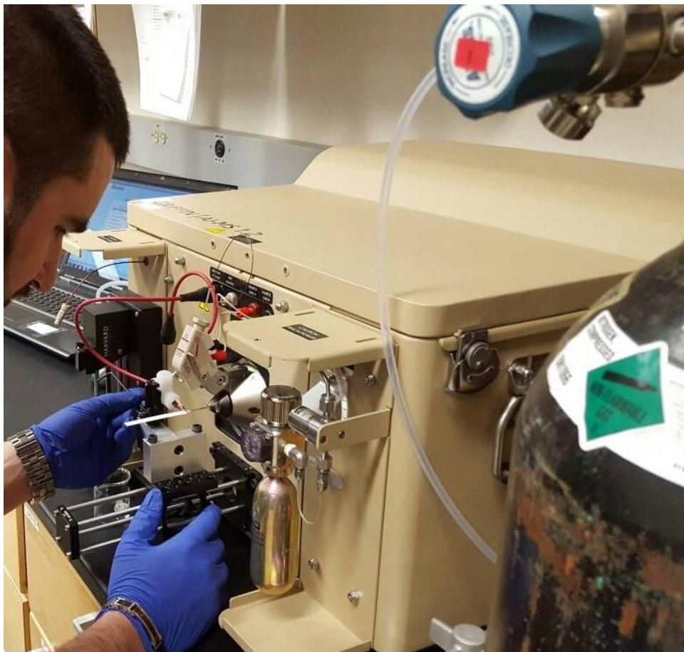
Figure 1.7 The FLIR System AI-MS 1.2 portable mass spectrometer. The AI-MS 1.2 weighs 45 kg and can perform both positive and negative ionization, as well as, multiple stages of mass analysis. Paper spray ionization is being performed in the photograph.
