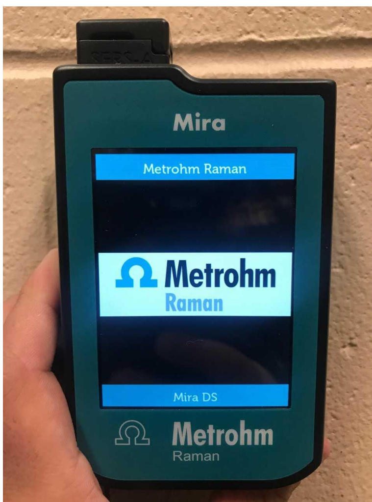
Figure 1.11 Portable and handheld Metrohm Mira Raman spectrometer with the pSERS attachment.
