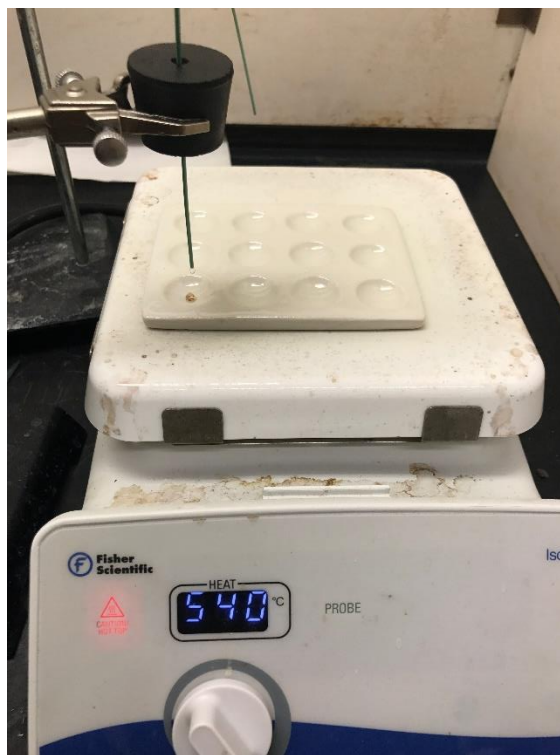
Figure 7.2 Photograph of the Leidenfrost setup for a Suzuki cross-coupling reaction.
