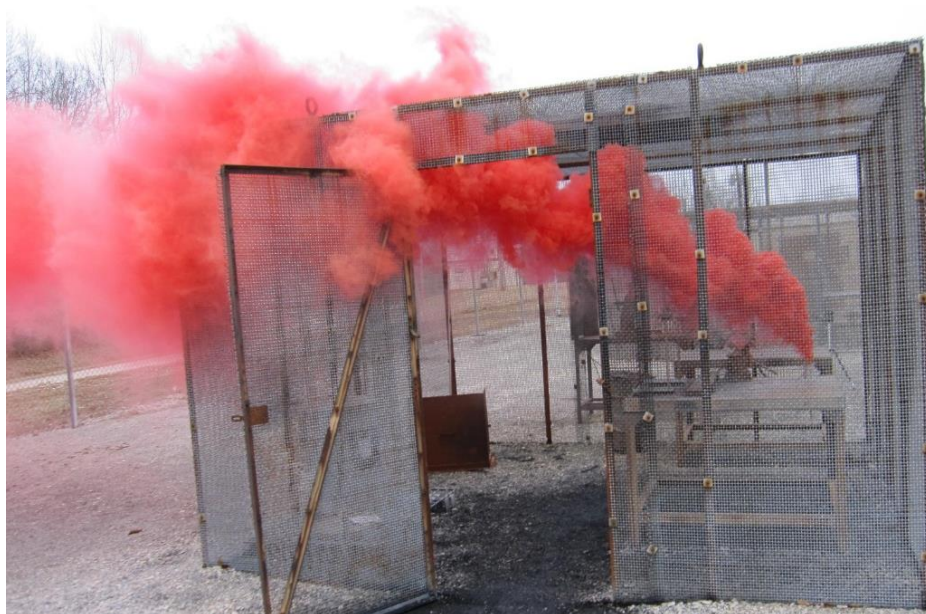
Figure 4.1 Mk124 smoke being functioned in a burn cage. Filter paper, swabs, and glass wool were positioned around the smoke to collect samples.
