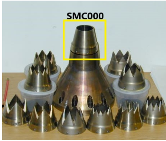
Figure 4.1. SMC000 nozzle mounted on a base (center) along with a collection of chevron nozzles [17].
