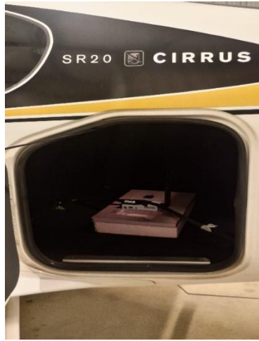
Figure 8: The mount ensures that the location and direction of the equipment is consistent in all flight tests.
