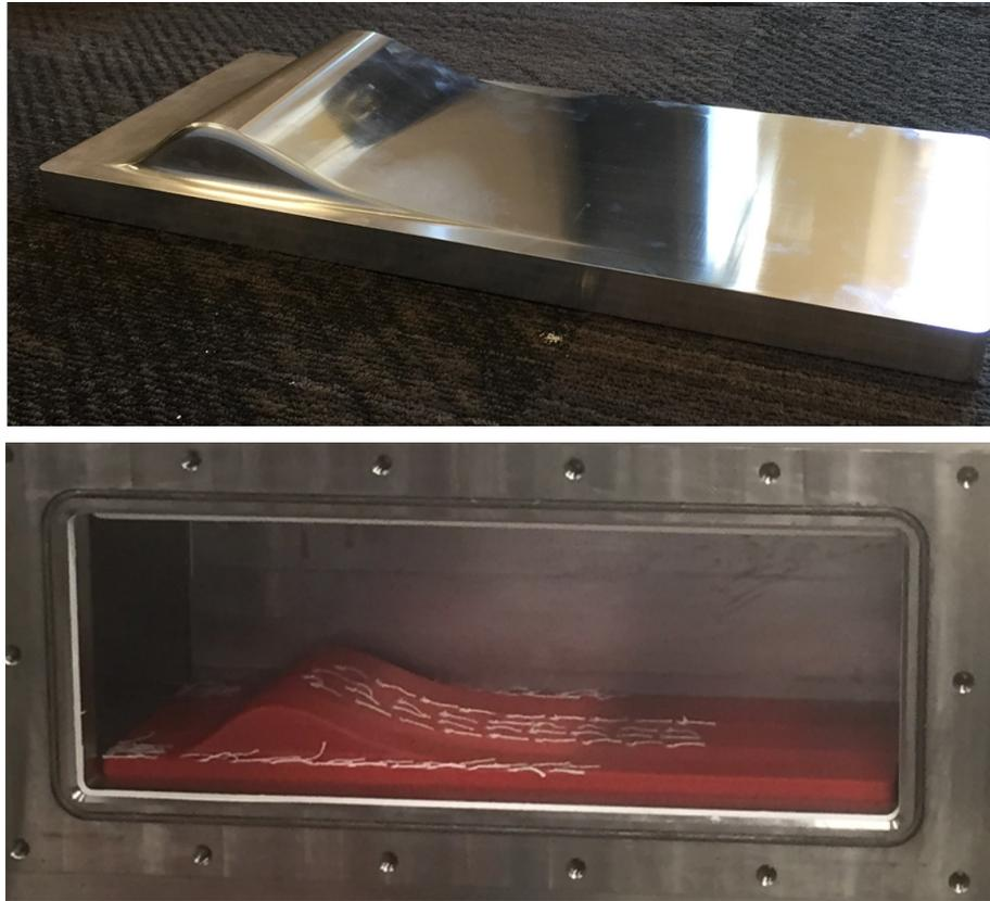
Fig. 4.46. Flow Separation Domain test article
