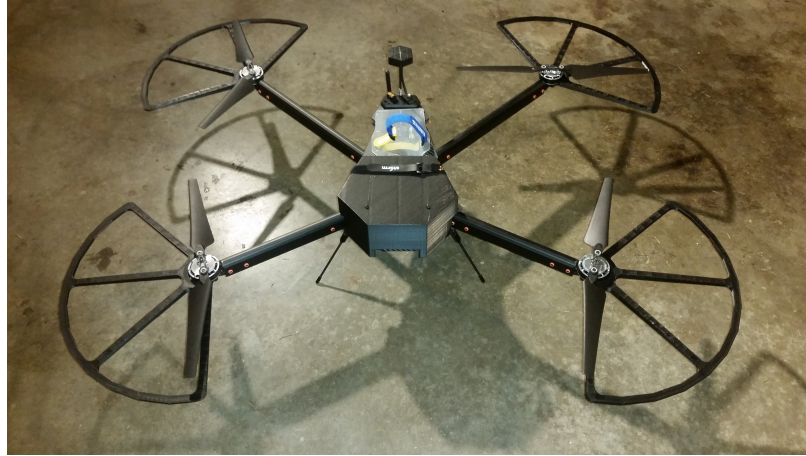
Fig. 5.1. Tarot Peeper quadrotor with custom 3D printed onboard computer canopy, prop guards, and optical flow sensor.
