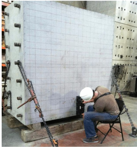
Fig. 2.17. The concrete specimen and the MIRA device used for the experimental data [33]. 20 defects are embedded in the specimen.
