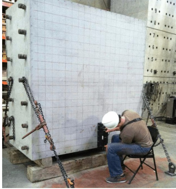
Fig. 1.12. The concrete specimen and the MIRA device used for the experimental data [33]. 20 defects are embedded in the specimen.
