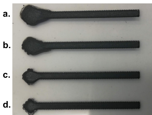
Figure 3.14 Varied y -pixel pitch 1.9 mm wide samples with pixel pitches of: (a) 0.2 mm, (b) 0.25 mm, (c) 0.33 mm, and (d) 0.5 mm.
