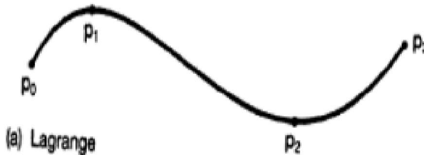
Fig. 2.1. Lagrange interpolation of a curve
