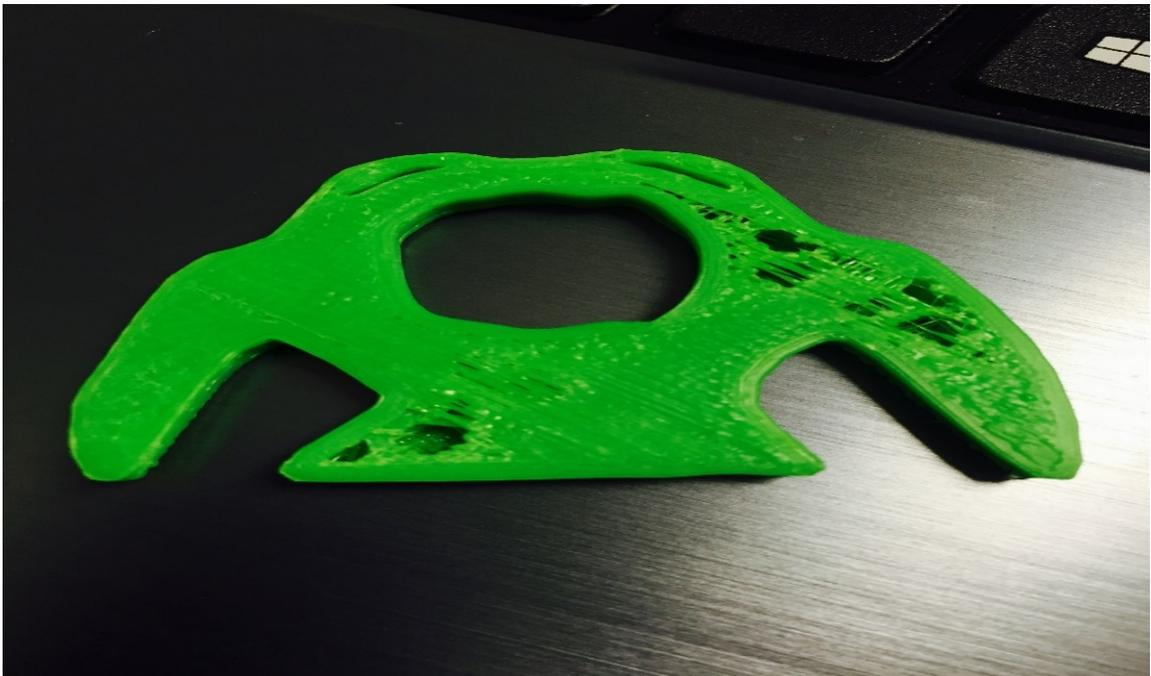
Fig. 5.36. Topological optimized structure developed using 3D printer with NURBS optimal parameters
