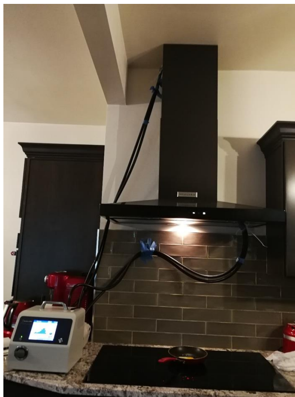
Figure 2.9 Setup of the NanoScan SMPS and OPS to determine the kitchen hood nanoaerosol removal efficiency.
