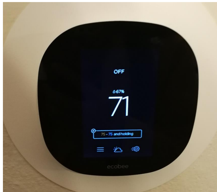
Figure 2.7 The Ecobee3 lite thermostat.
