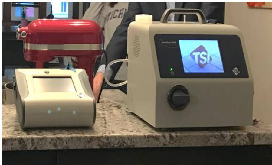
Figure 2.5 OPS (left) and NanoScan SMPS (right).
