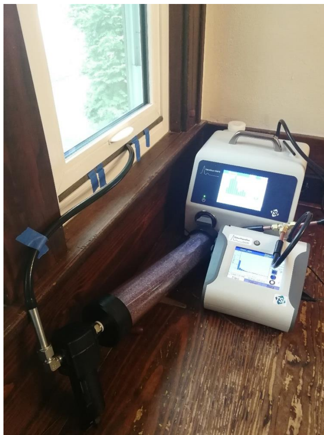
Figure 2.10 Setup of the diffusion dryer, NanoScan SMPS, and OPS for outdoor air sampling.
