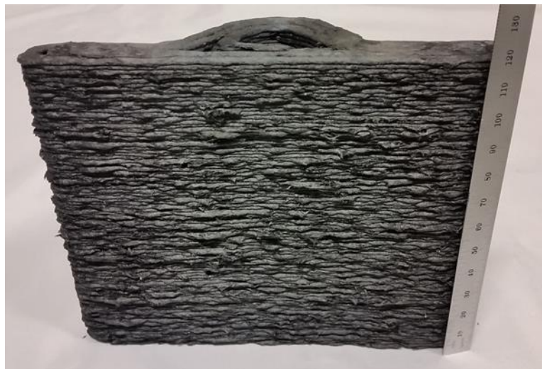
Figure 5.30 Stringer tool printed in CAMRI with 50% by weight of carbon fiber reinforced PPS (scale in mm).
