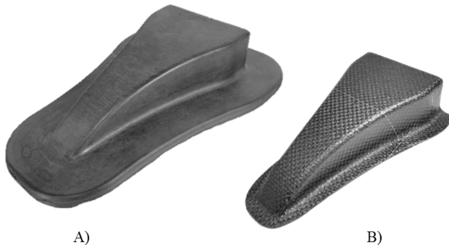
Figure 2.19 A) One-sided tool printed with 50% by weight of carbon fiber reinforced PPS for autoclave manufacturing process. B) Part manufactured on printed tool with IM7-8552
