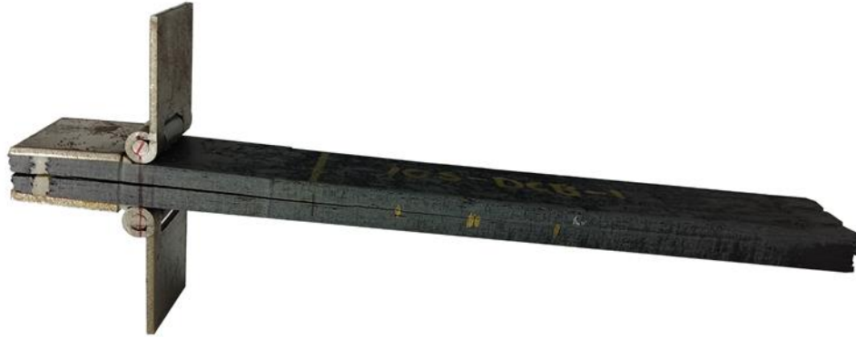
Figure 6.9 Example of printed DCB specimen prepared with piano hinges.
