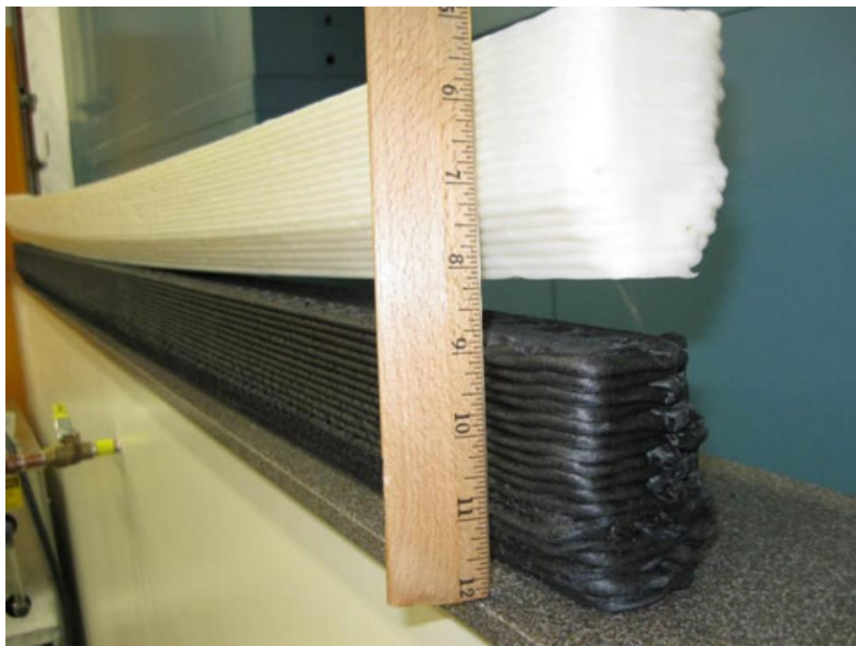
Figure 7.5 Warping of ABS vs CF-ABS in Large Scale FFF [2].
