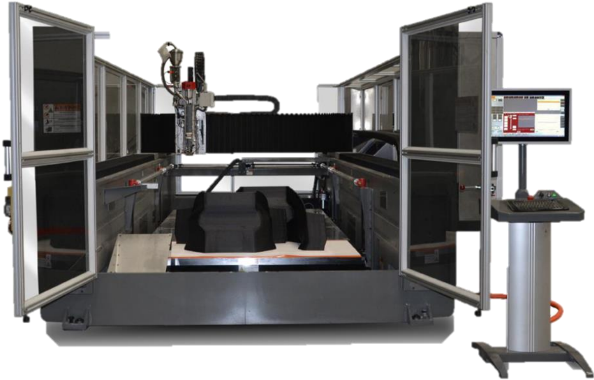
Figure 2.7 BAAM – Big Area Additive Manufacturing system developed by Cincinnati Incorporated ® [7].
