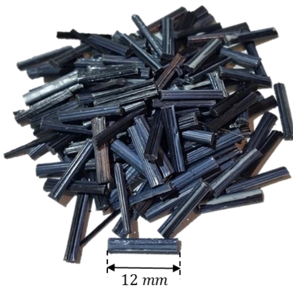
Figure 2.12 Pellets of Polyphenylene Sulfide reinforced with long discontinuous fibers.
