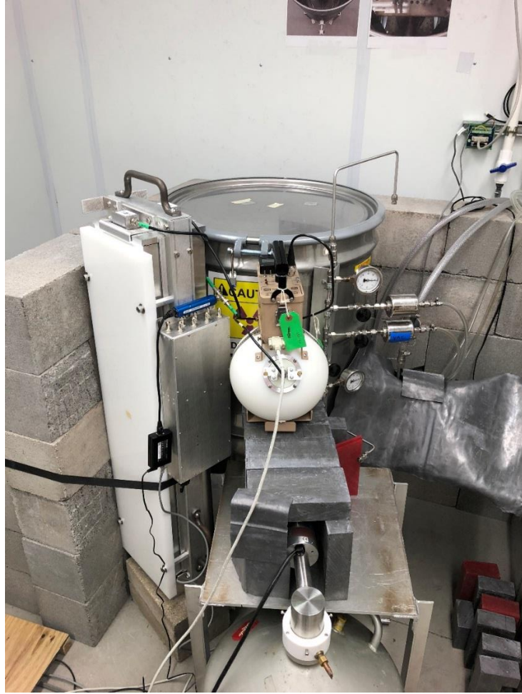
Figure 3.7 Experimental setup for the transient analysis of neutrons in UTA-1.
