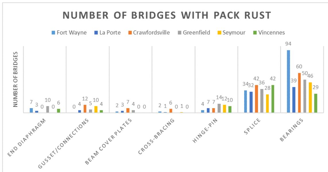
Fig. 4.22. Number of bridges with pack rust in bridge members
