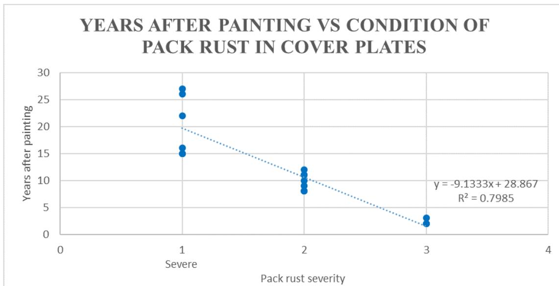
Fig. 4.32. Number of years after painting and the condition of pack rust in cover plates
