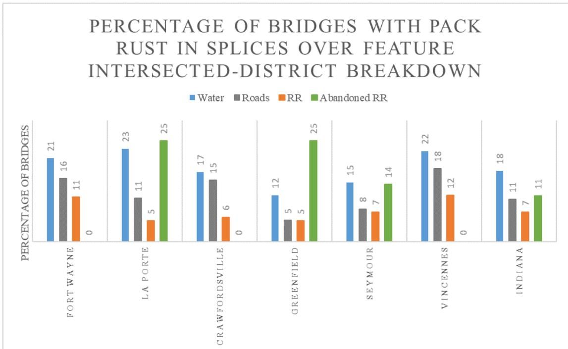
Fig. 4.26. Percentage of bridges with pack rust in splice over feature intersected
