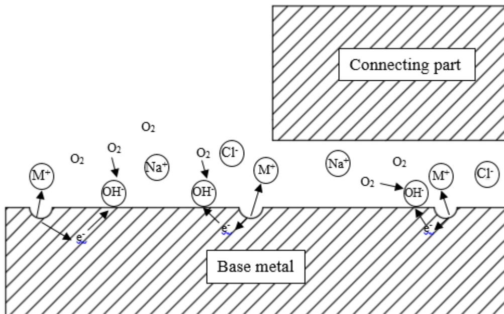
Fig. 2.3. Initial stage of corrosion
