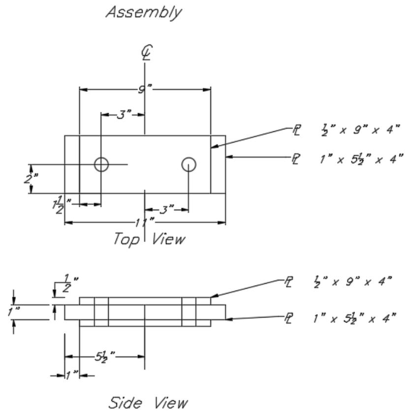
Fig. 5.6. Assembly of the splice connection with 7/8-in diameter bolts
