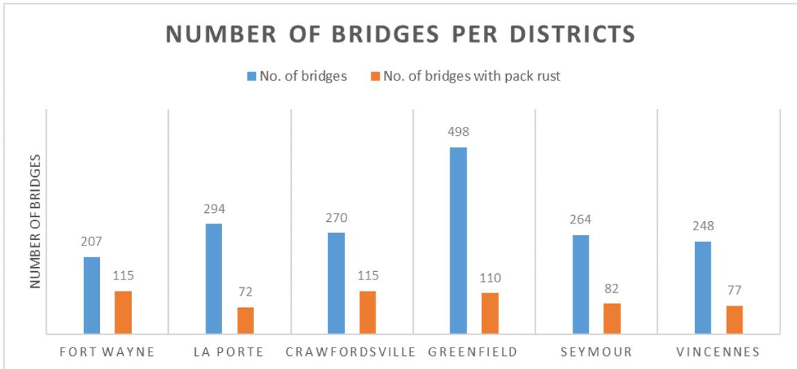
Fig. 4.19. Total number of bridges and number of bridges with pack rust in different districts
