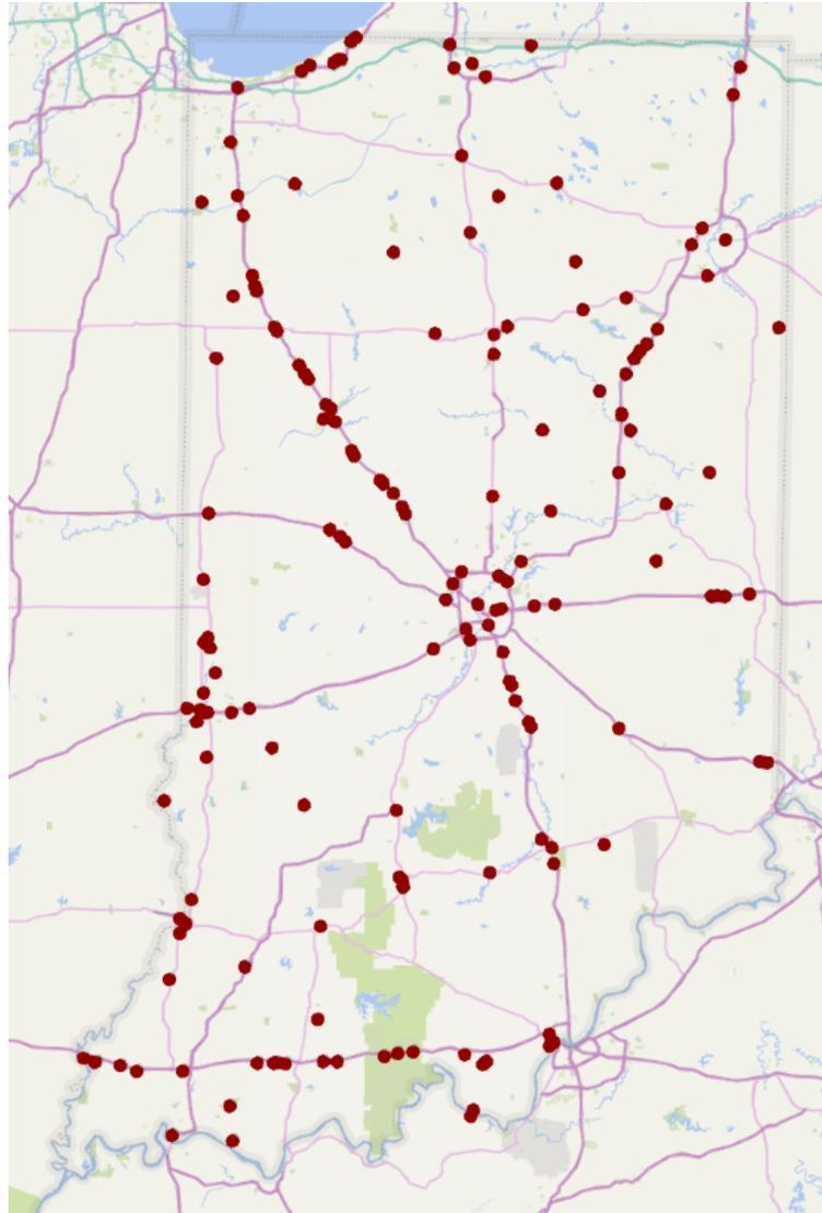
Fig. 4.31. Location of bridges with pack rust in splices
