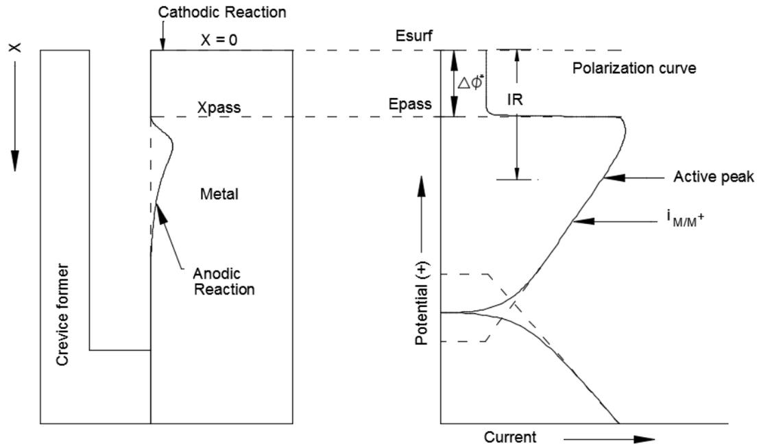
Fig. 2.6. Schematic of metal with crevice on the left and its matching polarization curve on the right [9]
