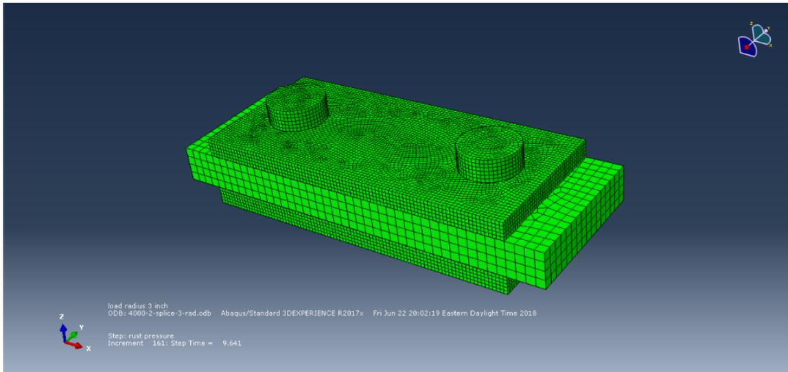
Fig. 5.9. Region over which pack rust pressure is applied
