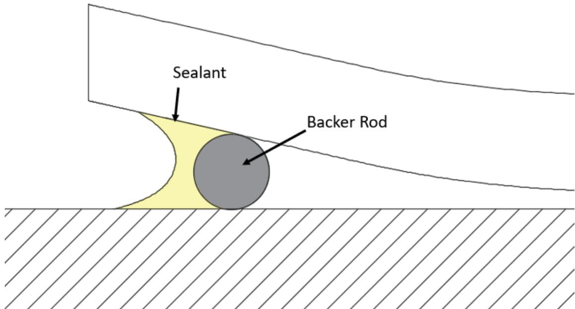
Fig. 3.3. Schematic diagram for backer rod and sealant
