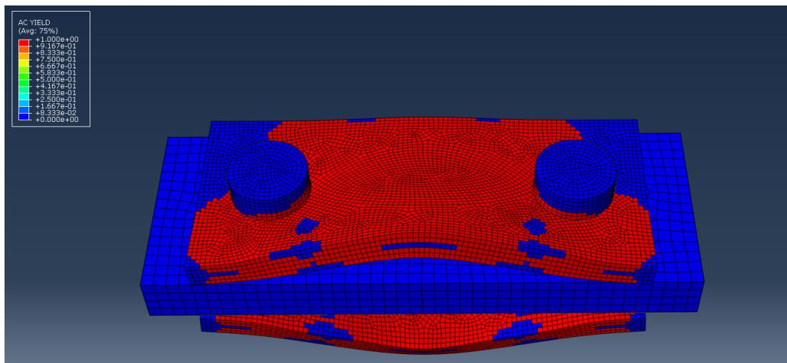
Fig. 5.18. Yielded region of splice plate at 1-in deformation
