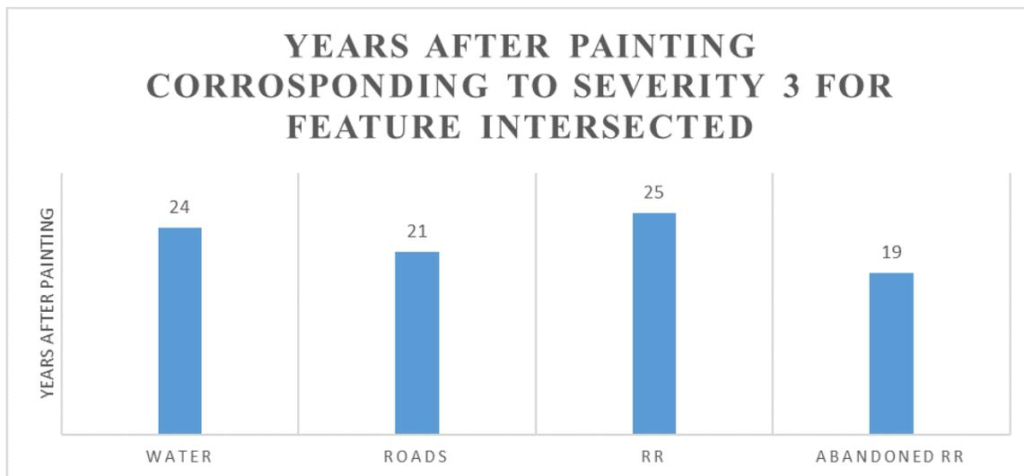
Fig. 4.29. Years after painting corresponding to severity rating 3 for feature intersected
