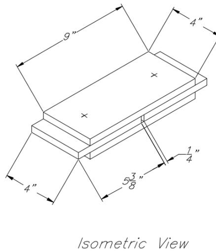
Fig. 5.4. Isometric view of the splice connection with a gap between the flange plates
