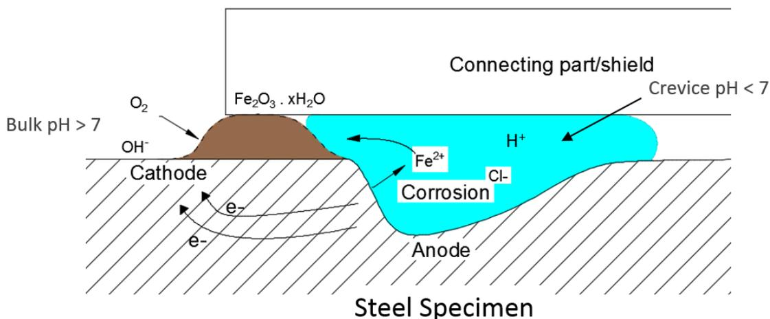
Fig. 2.5. Rust deposit at the mouth of the crevice and acidification of crevice solution
