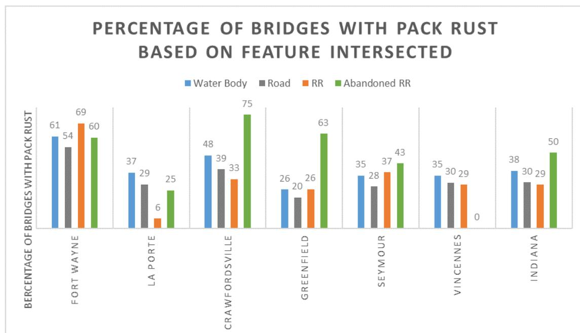
Fig. 4.21. Percentage of bridges with pack rust based on features intersected
