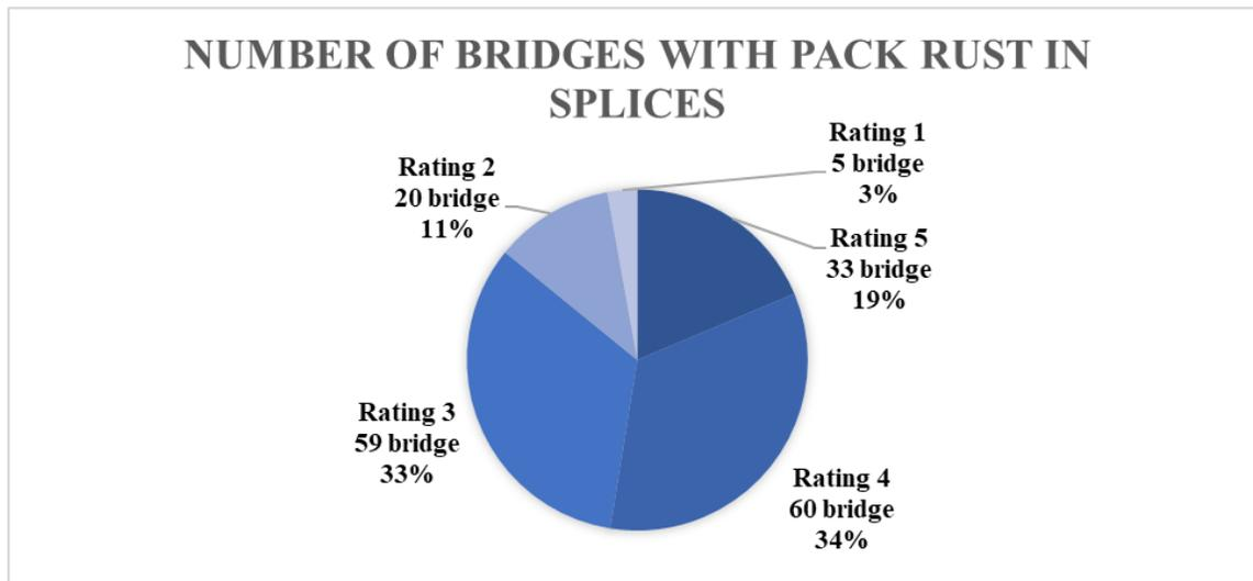
Fig. 4.24. Number of bridges with pack rust in splices classified by pack rust rating
