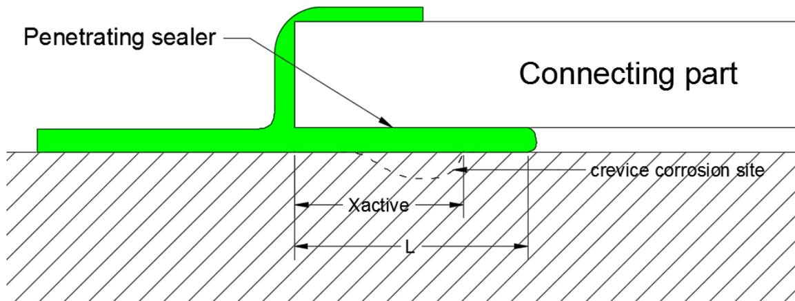
Fig. 3.2. Schematic diagram for penetrating sealers
