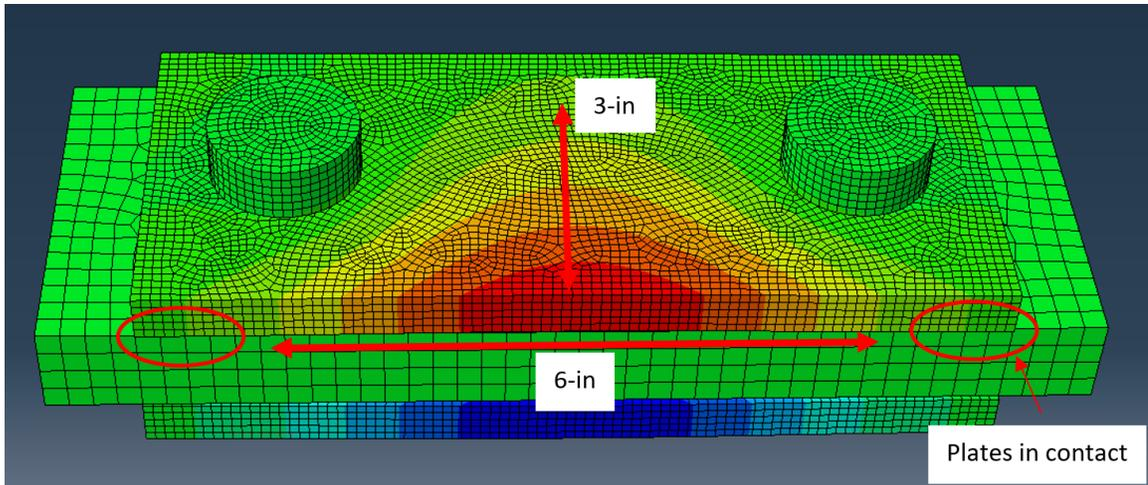
Fig. 5.17. Splice plate deflection at 1800 psi pressure
