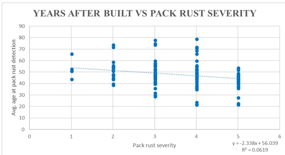
Fig. 4.30. Relation between years after built and pack rust severity in splices
