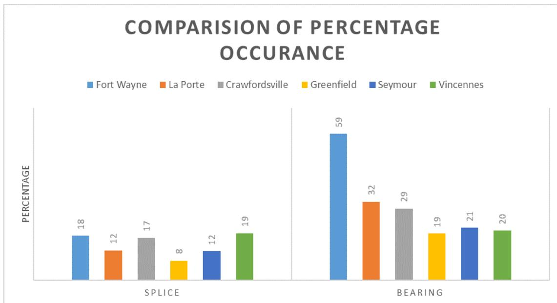
Fig. 4.23. Percentage of pack rust occurrence in splices and bearings for each district
