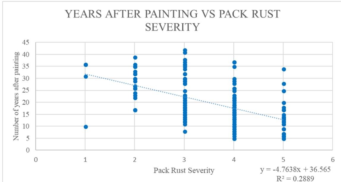
Fig. 4.28. Relation between years after painting and pack rust severity in splices
