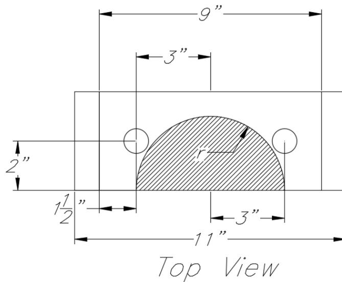
Fig. 5.7. Region over which pack rust pressure is applied
