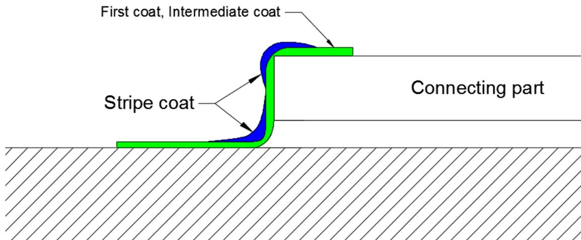
Fig. 3.1. Paint film and stripe coat thickness
