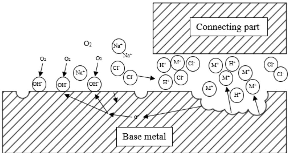
Fig. 2.4. Corrosion at a later stage
