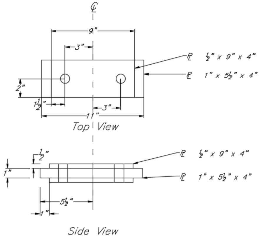
Fig. 5.3. Assembly of the splice connection with 1-in diameter bolts
