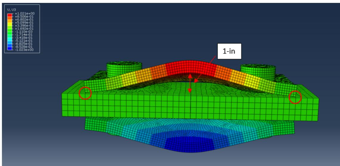
Fig. 5.19. 1-in of splice plate deflection at 2960 psi pressure
