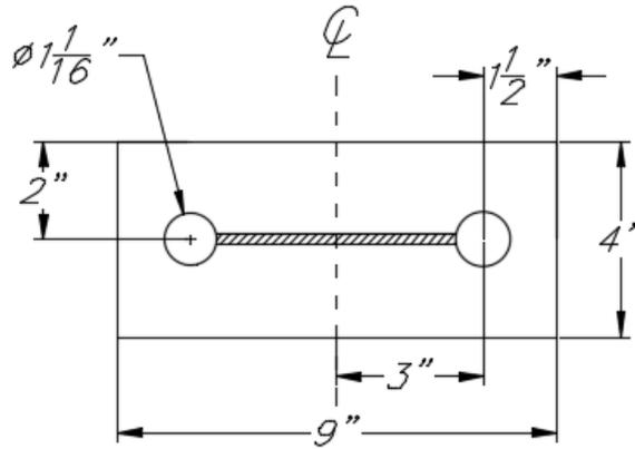
Fig. 5.15. Simplified beam element
