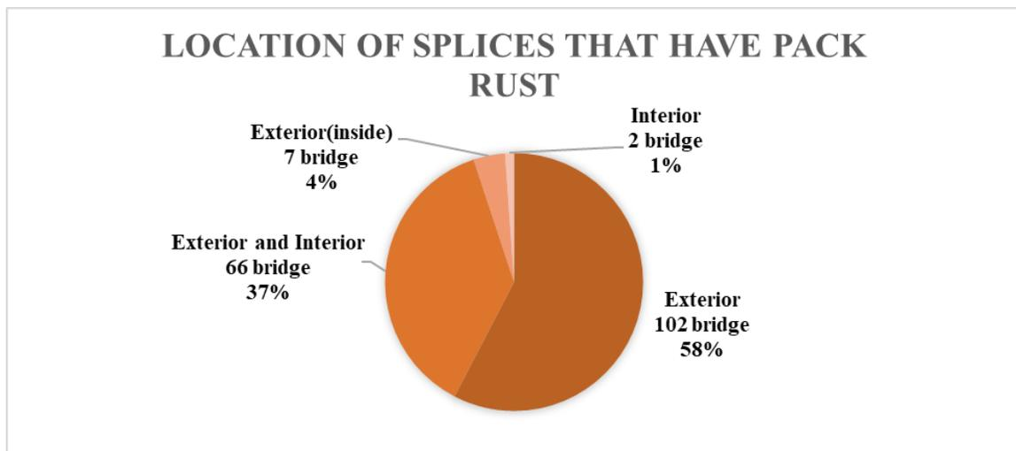
Fig. 4.25. Location of splice connections that have pack rust
