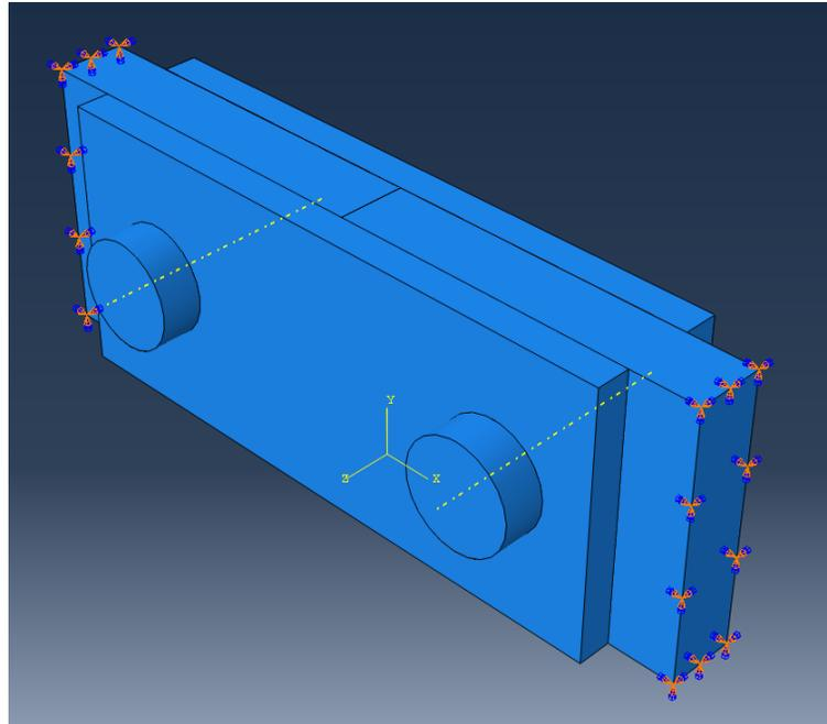
Fig. 5.8. Boundary condition applied in the model
