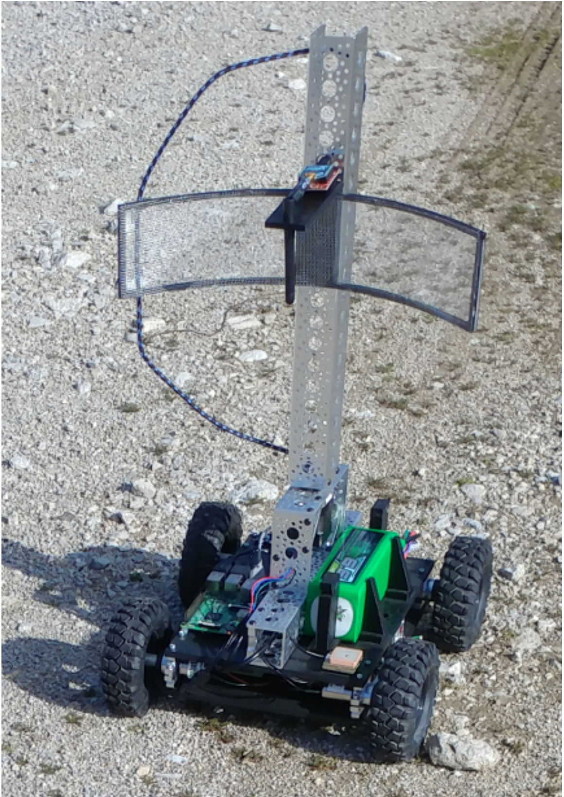
Figure 4.18. Custom-made parabolic dish section antenna.
