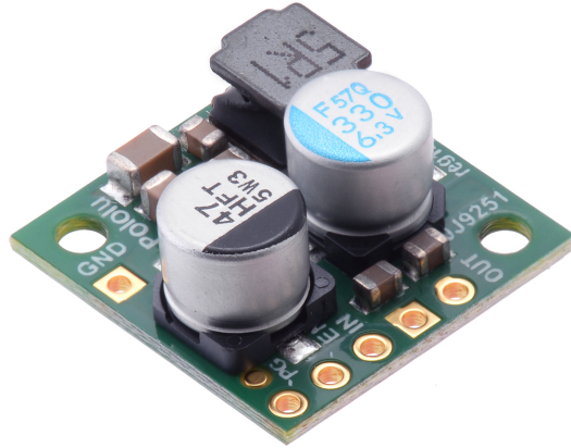
Figure 3.7. 5V step-down voltage regulator for Raspberry Pi.
