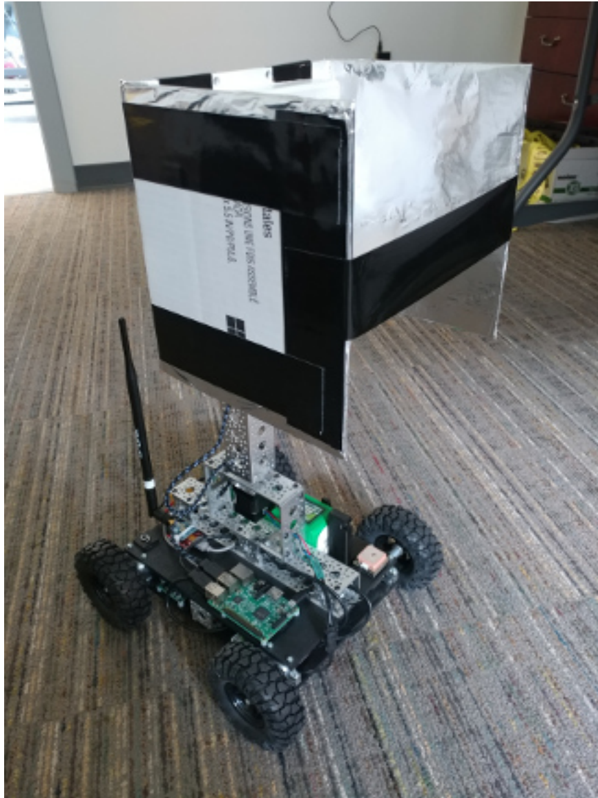
Figure 4.15. Unsuccessful attempt to attenuate unwanted RF radiation with aluminum foil.
