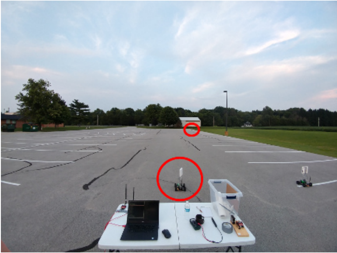
Figure 5.16. Trial 17: step 10. The more distant highlighted robot has requested an extension, which the closer highlighted robot has been assigned to (notice its antenna in mid-rotation).
