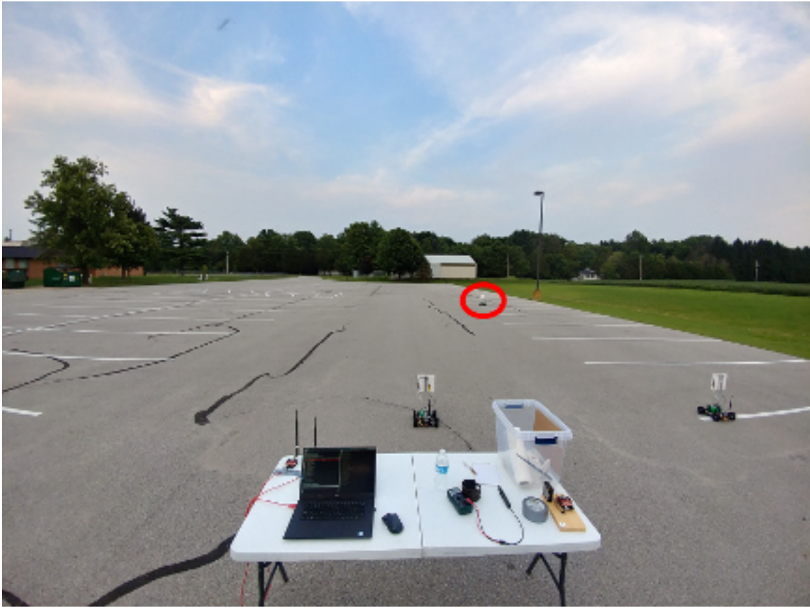
Figure 5.11. Trial 17: step 5. The highlighted robot continues to track toward the beacon.
