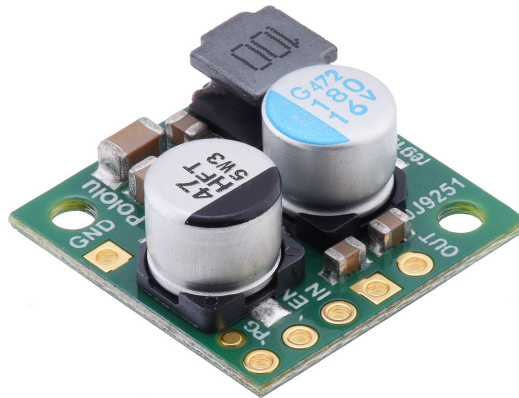
Figure 3.6. 12V step-down voltage regulator for stepper motor.
