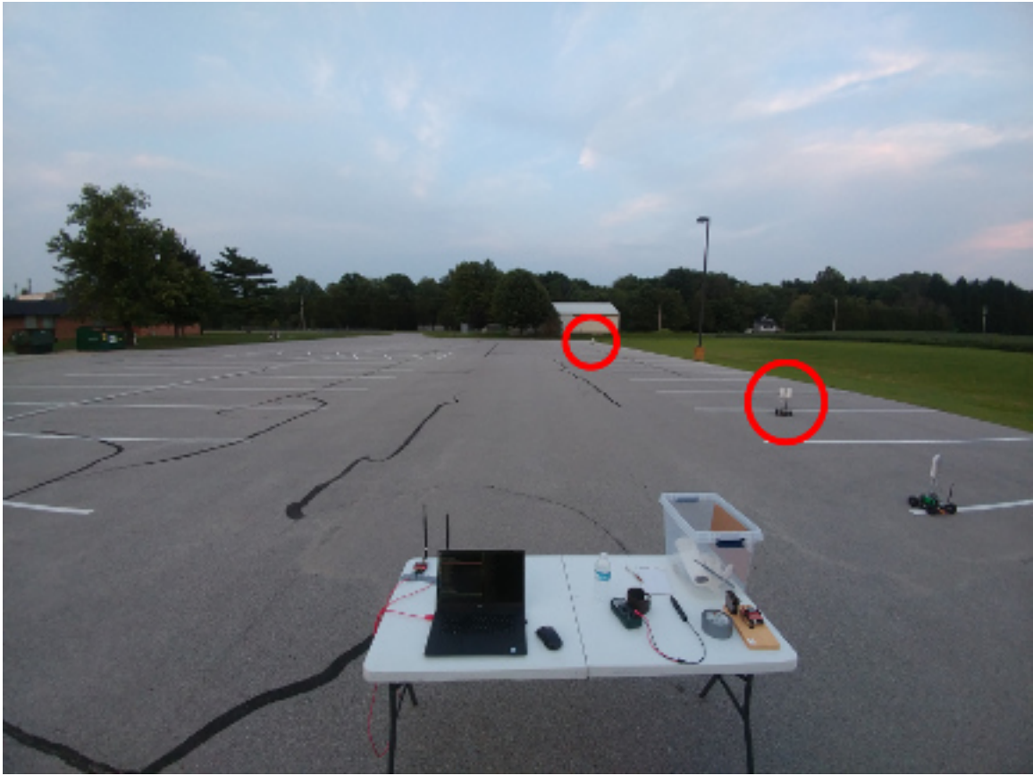
Figure 5.17. Trial 17: step 11. The more distant highlighted robot was bumped by the closer highlighted robot. The closer robot has now called for its own extension, which the remaining robot is in the process of executing.
