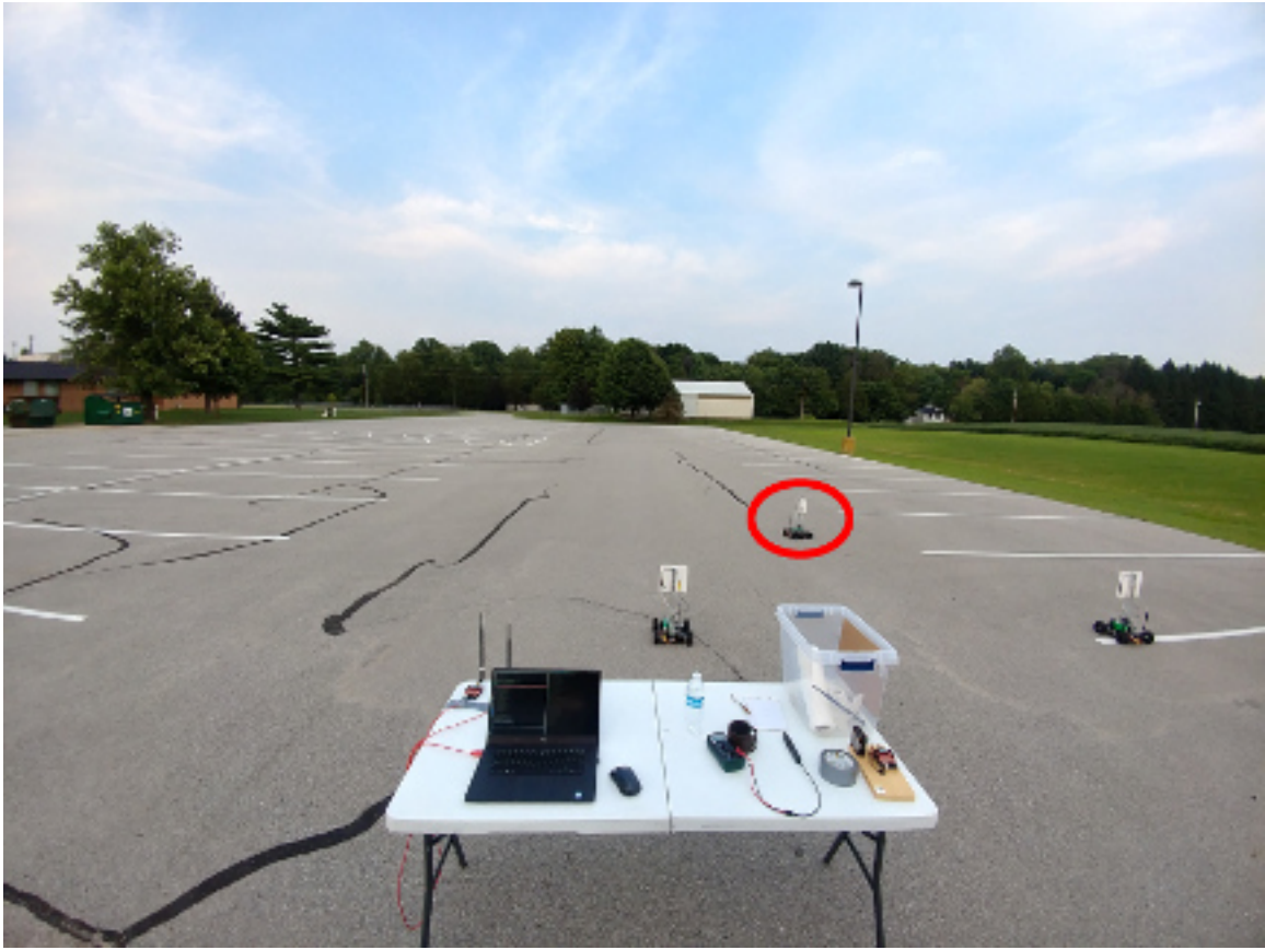
Figure 5.8. Trial 17: step 2. The highlighted robot has completed one search iteration and has moved one step toward the beacon.
