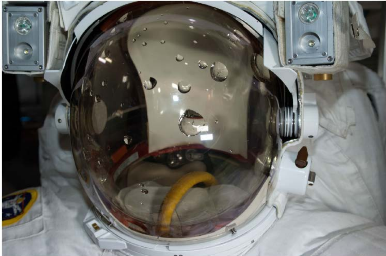
Figure 5.16: EVA suit water intrusion picture [NASA, 2013]
