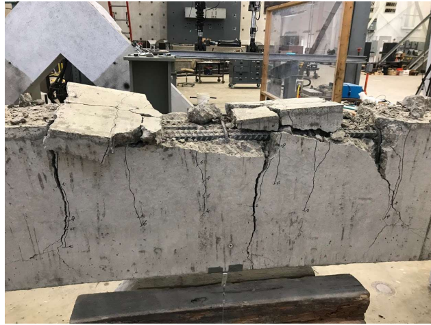
Figure 3.9: Typical Confined Specimen Failure (C3/60-40-5-100)
