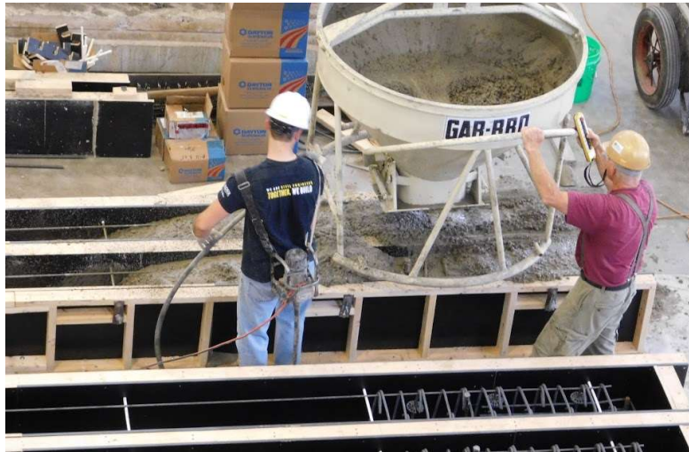
Figure 2.17: Casting Procedure for Specimens
