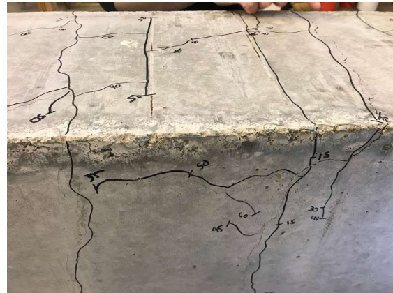
c) Tension and Side Faces of Specimen U-120-5-M
