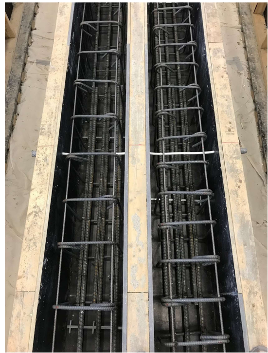
b) Confined Lap Splice (Left: C3/60-60-5-100, Right: C3/60-60-5-150)
