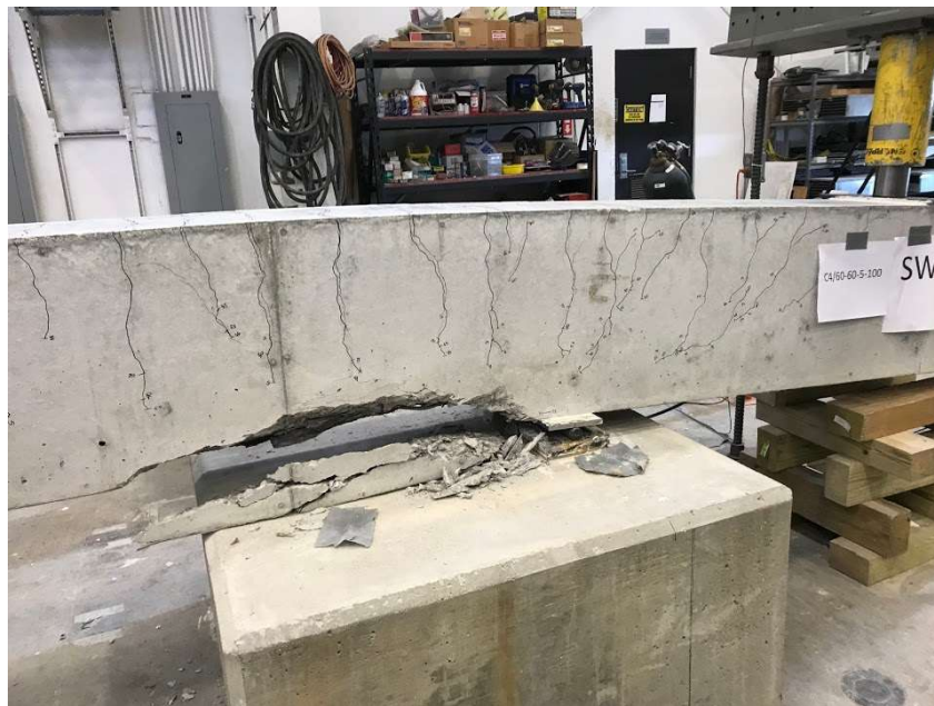
Figure 3.10: Flexural Failure (C4/60-60-5-100)
