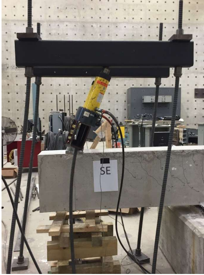
Figure 2.22: Dywidag Bars Yielding in Testing of U-80-5
