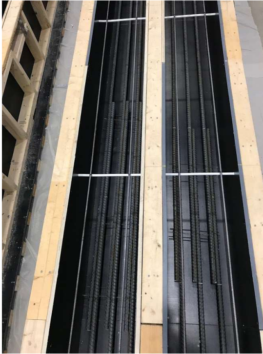
a) Unconfined Lap Splice (Left: U-60-5, Right: U-40-5)
