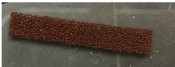
Figure 3.1.: The \text{MnO}_2 coated GF sheet cut in the required dimension of 2.5 cm x 0.6 cm.
