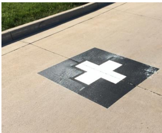
Fig. 6.5 Painted plus target on concrete road
