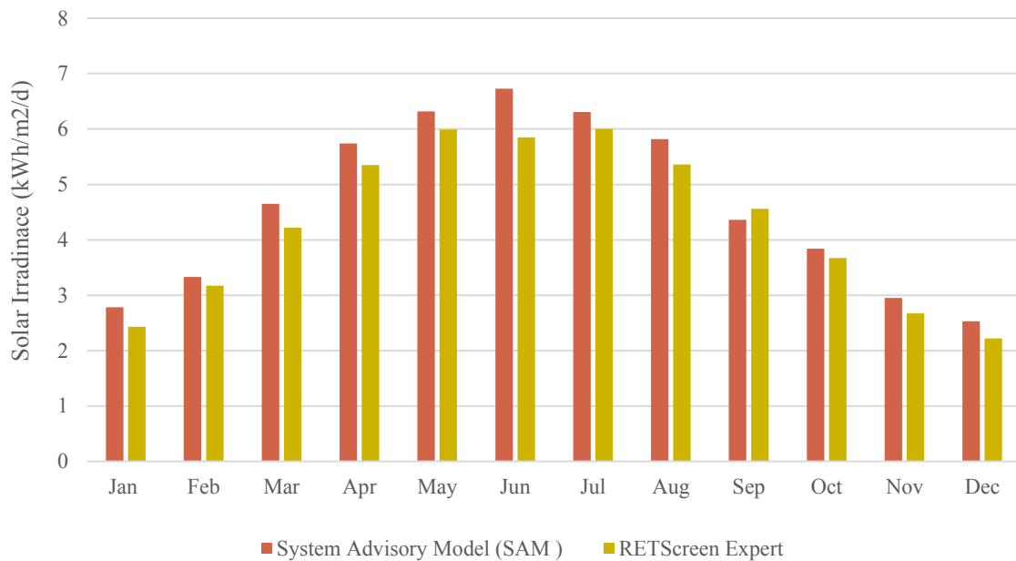
Figure 3.6 Irradiance on horizontal surface at Atlanta, GA ( \text{kWh/m}^2/\text{d} )
