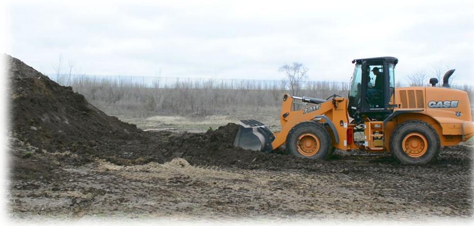
Figure 9.1. Wheel loader pushing a material pile during a Grading Test.
