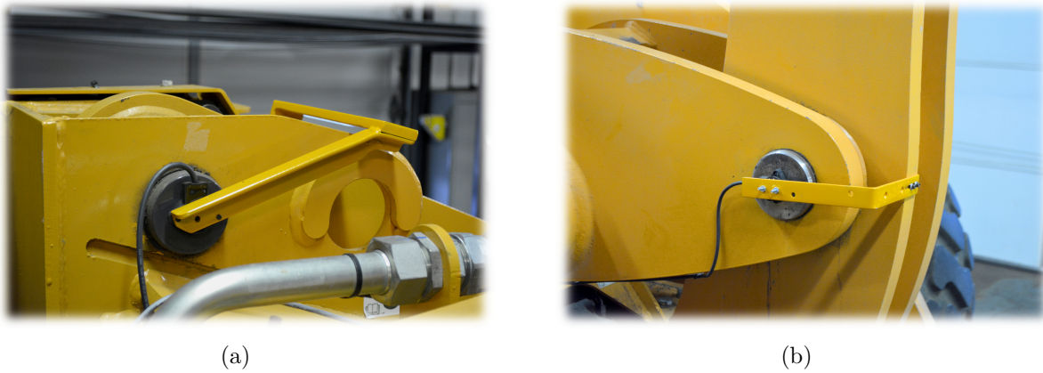
Figure 7.5. Angle sensors installed at (a) boom and (b) bellcrank pins.
