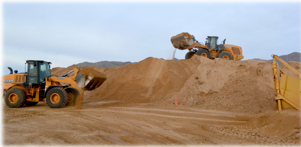
Figure 9.8. Test setup for final Productivity Tests, showing test wheel loader (left) and backfill loader (top) at the digging pile with dumping area to the right.
