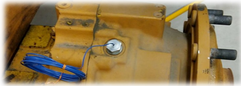
Figure 7.6. Wheel hub thermocouple mounting.
