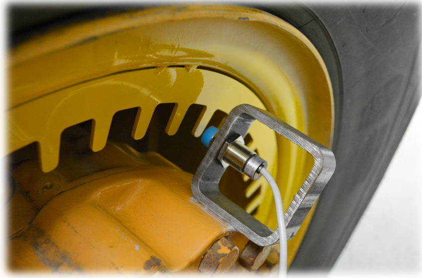
Figure 7.3. Inductive wheel speed sensor with encoding wheel mounted on vehicle wheel rim.
