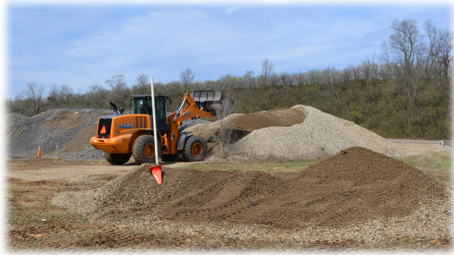
Figure 9.2. Productivity Test setup, showing wheel loader at the digging pile with dump pile in the foreground (white pole and orange traffic cone indicate dumping height and location).
