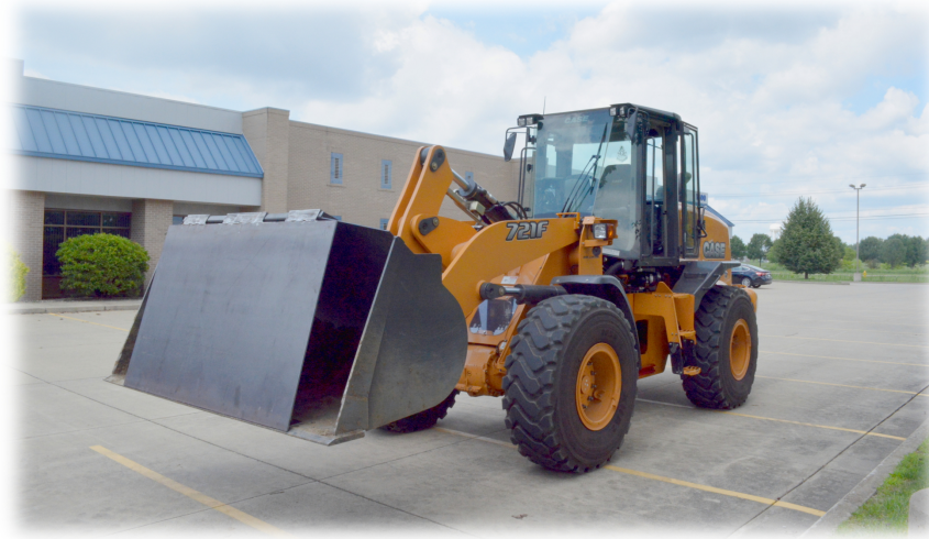
Figure 8.6. Plate mounted on wheel loader bucket for pushing against tires.
