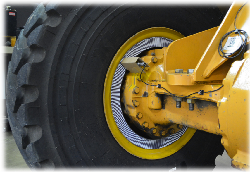
Figure 7.4. Optical wheel speed sensor with encoding wheel mounted on vehicle wheel rim.
