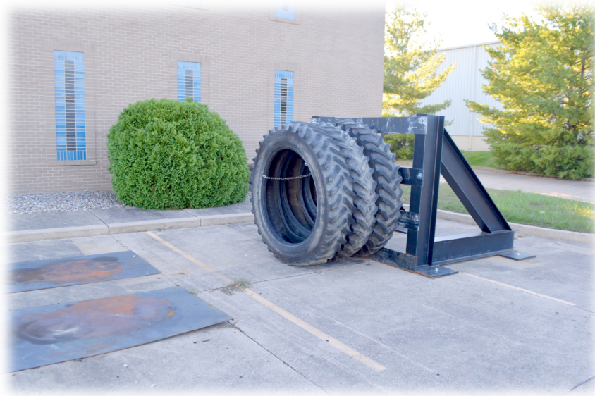
Figure 8.5. Test barrier used for experimental testing at Maha Laboratory, showing the tires and two of the four steel plates.
