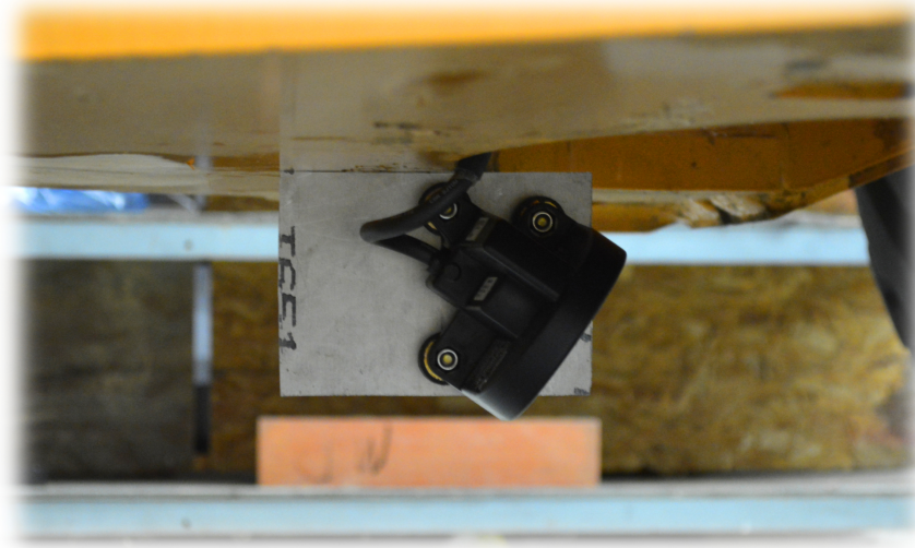
Figure 7.2. Ground speed sensor mounted on reference machine.
