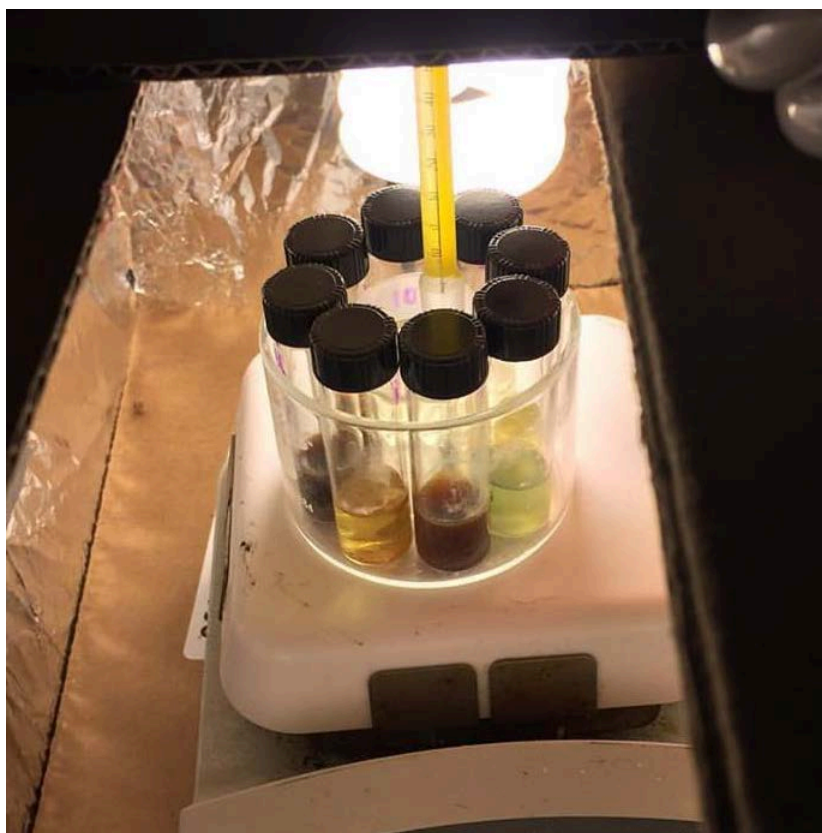
Figure 5.1 Example of reactions stirring in the engineered photo-reactor.
