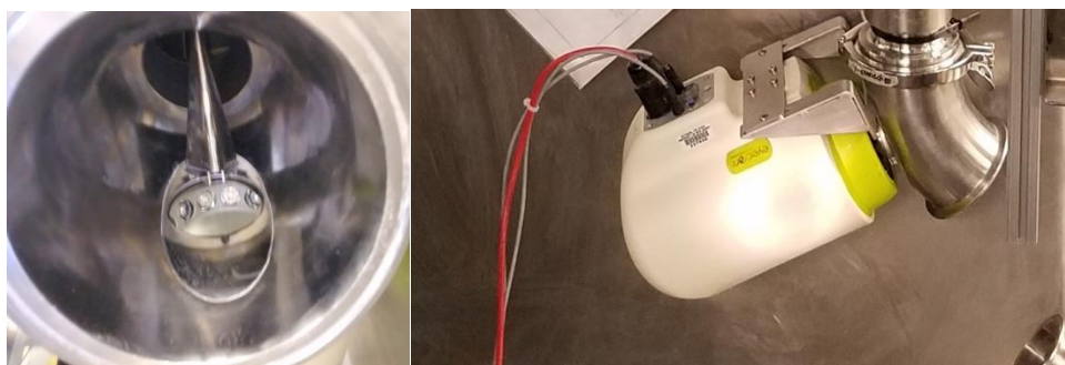
Figure 5.2. Y-connection configuration for real-time granules PSD monitoring
