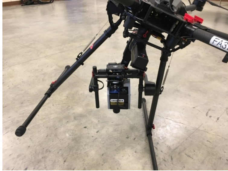
Figure 5.7: DJI Ronin MX 3-axis brushless gimbal stabilizer that maintains the scanner in nadir view
