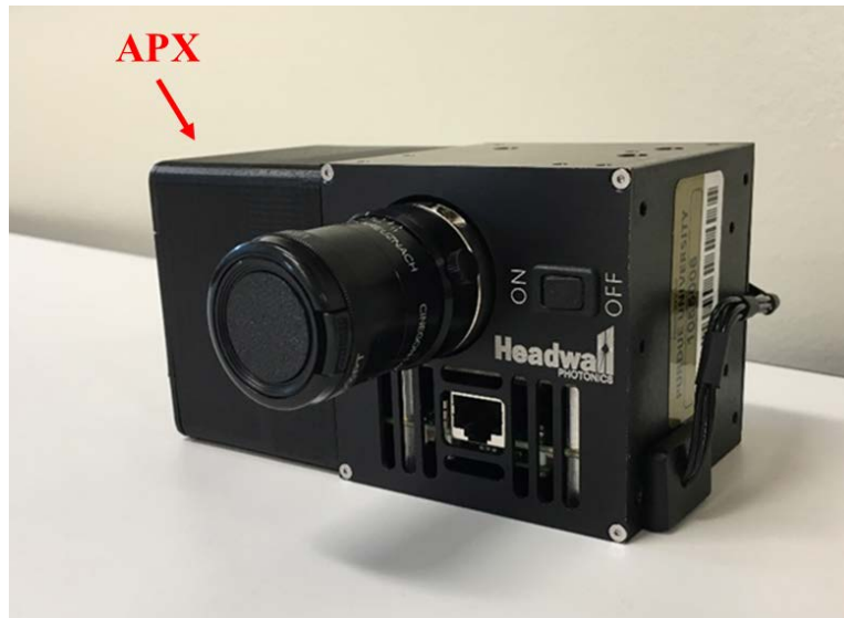
Figure 5.4: Trimble APX-15 UAV (V2) attached to the Nano-Hyperspec push-broom scanner
