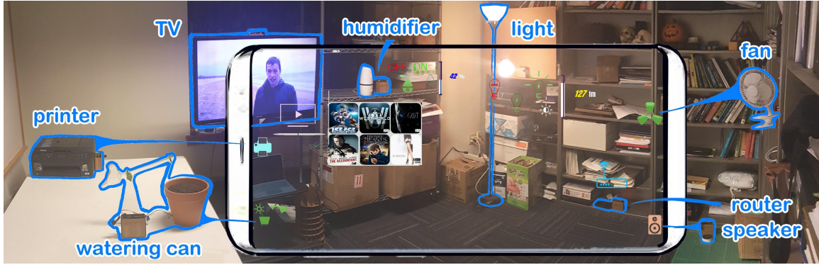
Figure 5.1. Scenariot is a method for discovering and localizing IoT devices with a SLAM-based AR device. We embed UWB distance measurement units on the controllers of each IoT device. We register the discovered devices spatially in the AR scene to enable new spatial aware interactions.
