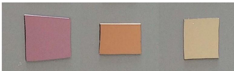
Figure 4.2 Digital images of ALD titanium nitride on silicon for thickness of (a) 89 nm (b) 55 and (c) 28 nm .
