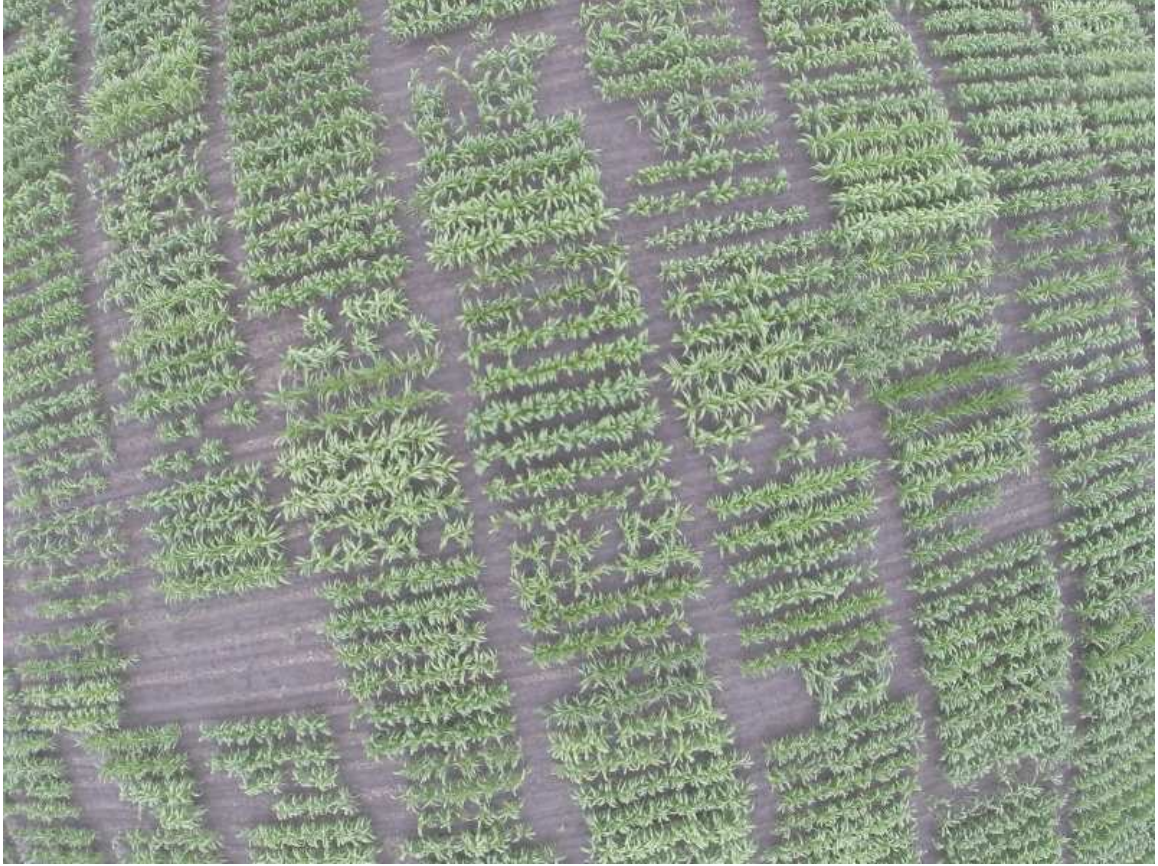
Fig. 2.3.: Example of a perspective image, an original image with distortion, as taken from a GoPro camera. This is an extreme case of perspective distortion from the 2015 dataset, used for illustration purposes. Non-GoPro cameras used in posterior years do not show such high distortion.
