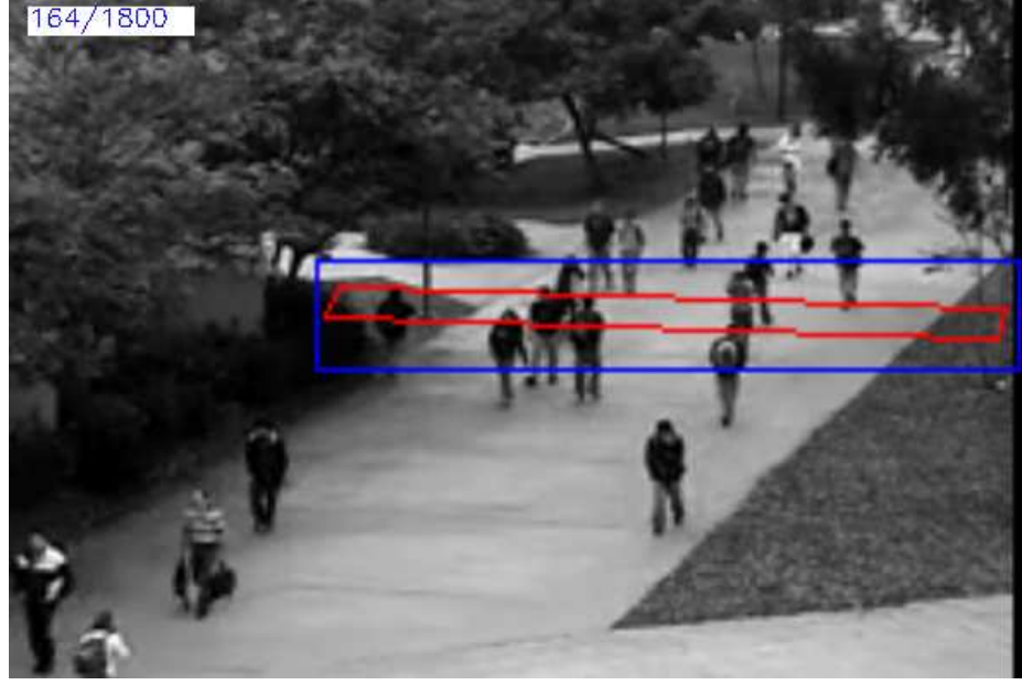
Fig. 5.1.: Example of a ROI and a Tripwire drawn over a frame of a surveillance video. ROI is in blue, and Tripwire in red. Source: [57]
