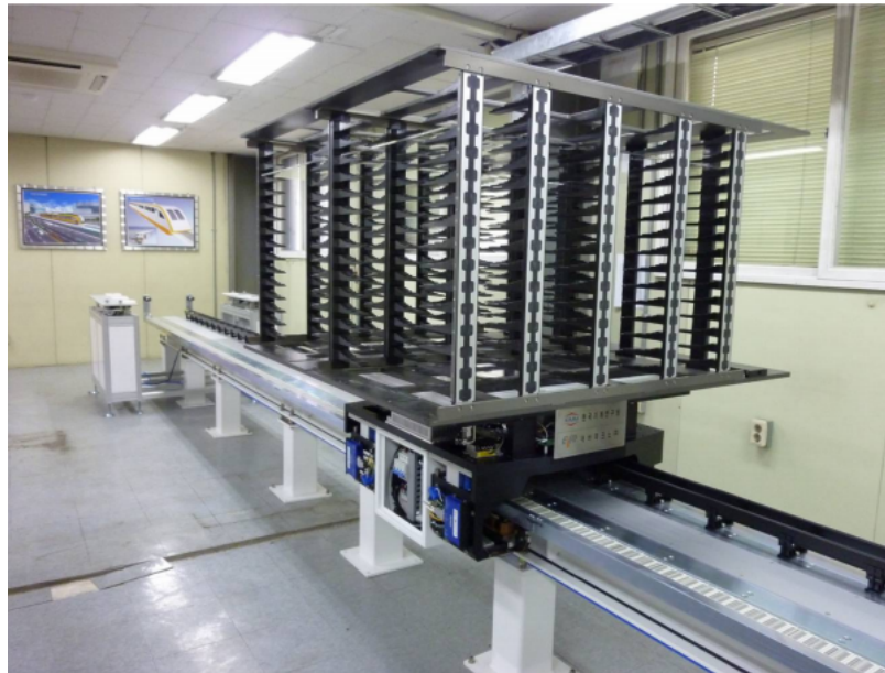
Figure 1.4. Magnetic levitation conveyor system for carrying LCD glass [22].
