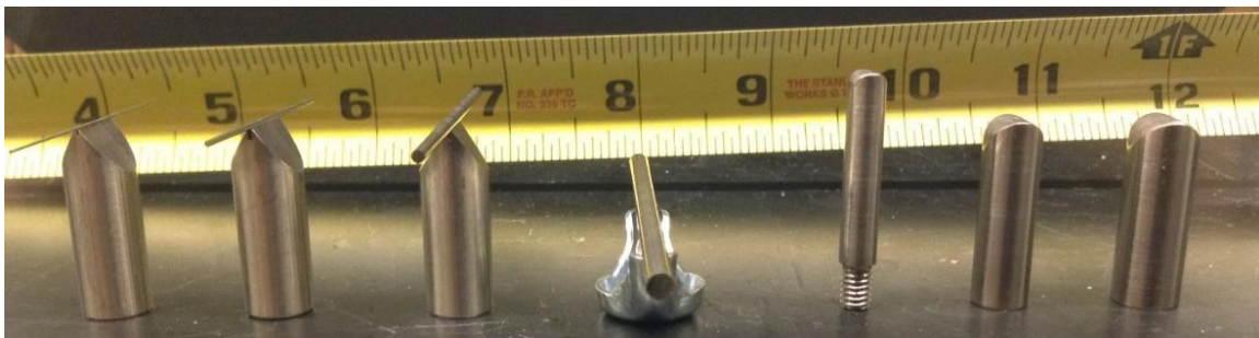
Figure 4: Seven different indenters used in transverse loading experiments. From left to right, the indenters possess radii of curvature of 0.20, 0.40, 0.79, 1.59, 2.50, 3.81, and 4.50 mm.
