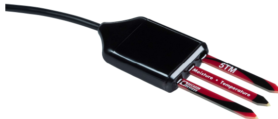
Figure 8-3 Integrated soil moisture-temperature sensor (METER Group Inc.)
