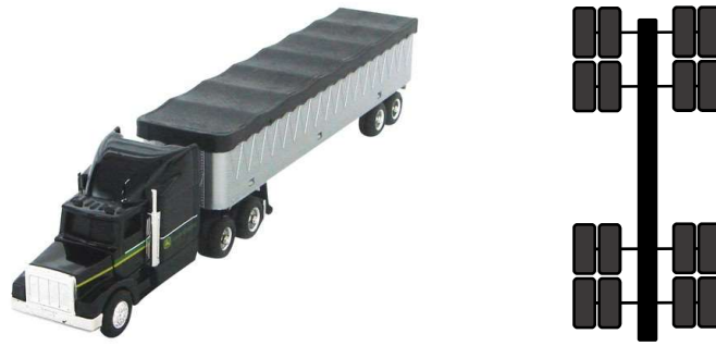
Figure 6-5 Truck, including two tandem axles, each with dual tires
