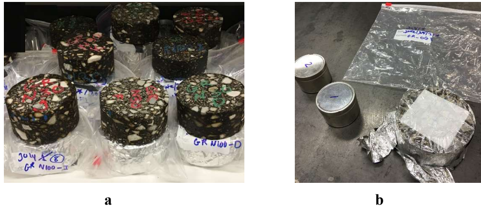
Figure 4-3 Filter-paper test a) stored samples with extra cores on top, b) opening samples after the seven-day equilibrium period
