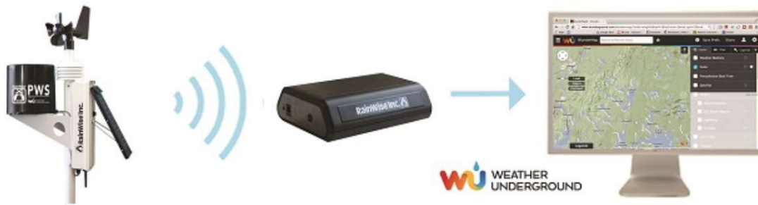
Figure 8-4 Weather station with wireless capability (RainWise Inc.)
