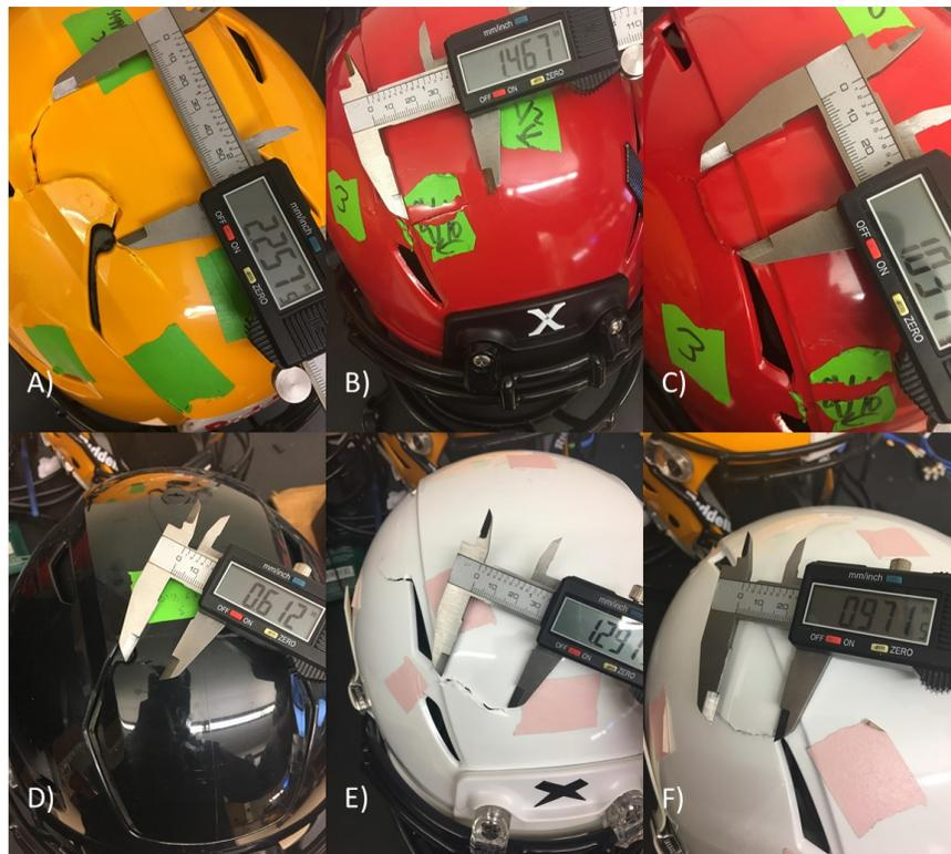
Figure 5.4. Crack length visible on various helmets. A) is the Riddell Youth Speed Flex, B) and C) are the Xenith Epic+ Youth, D) is the Riddell Speed Flex, E) and F) are the Xenith Epic+ helmets.
