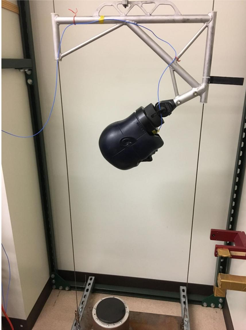
Figure 2.1. An unhelmeted NOCSAE Drop Tower rig pictured in the HIRRT Laboratory and performed testing following the NOCSAE football helmet and lacrosse helmet testing from 2013.
