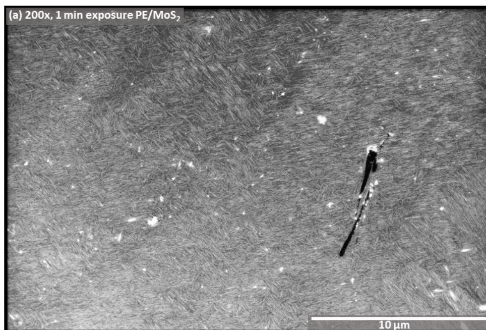
Figure B.3 SEM image of AuNW adsorption at 200x dilution with 1-minute exposure on diyne PE/MoS 2 .
