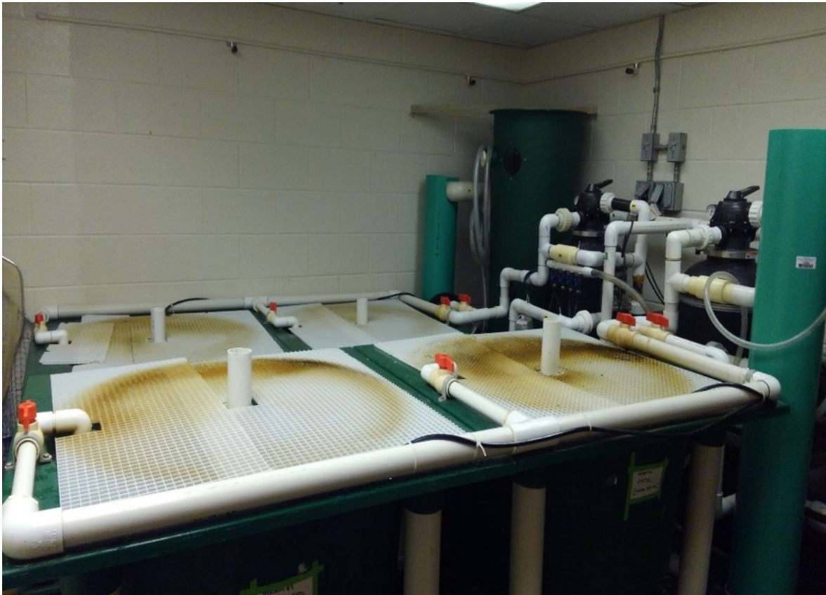
Figure 1. Recirculating aquaculture systems. This picture shows the two identical recirculating aquaculture systems used for this experiment. Both systems consist of two identical 200 gallon tanks that drain into a 400 gallon sump located beneath the tanks. Each system is filtered by its own sand filter that can be seen in the picture. The water is then returned to the tanks to complete the system.
