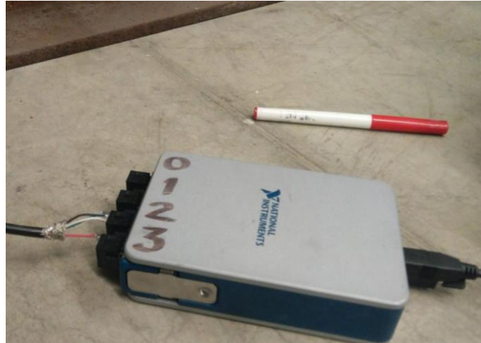
Figure C-5 NI 9219 Input Module and cDAQ-9171
