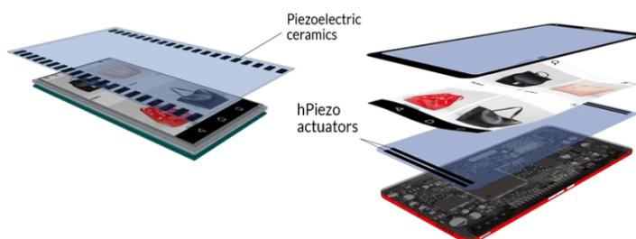
Fig. 2.16 Structure of piezoelectric friction haptic display.
