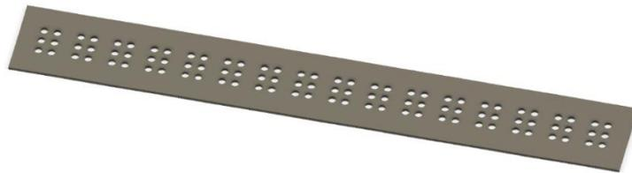
Fig. 3.23 Drawing of the top plate for the ‘braille stick’ for 3D printing.
