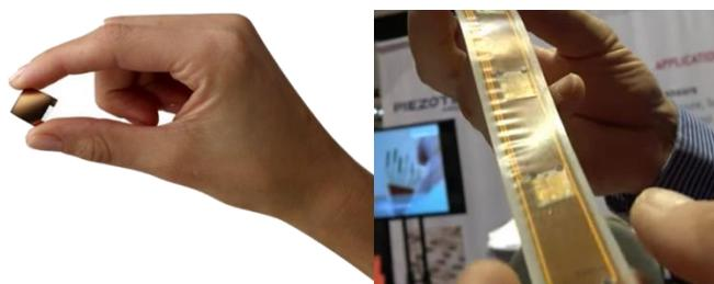
Fig. 2.18 Electroactive polymer actuator (Novasentis).
