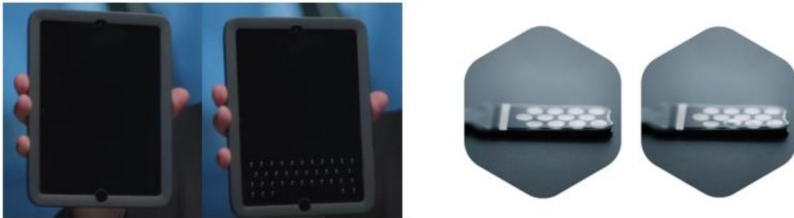
Fig. 2.19 Haptic actuators and operations using microfluidics (left) and pneumatic (right).
