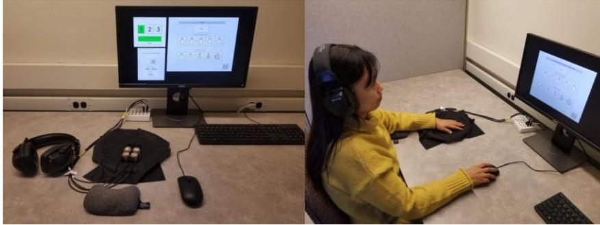
Fig. 4.9 Experimental setup: (left) noise-reduction headset, the factor array display, elbow support, computer monitor and mouse; (right) the participant in the middle of the affective rating experiment.
