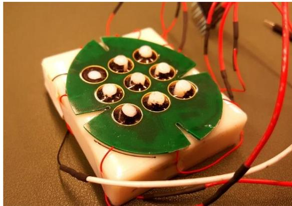
Fig. 3.25 3-by-3 electroactive polymer tactile display.
