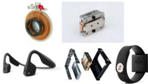
Fig. 2.10 Voice-coil haptic actuators and products.
