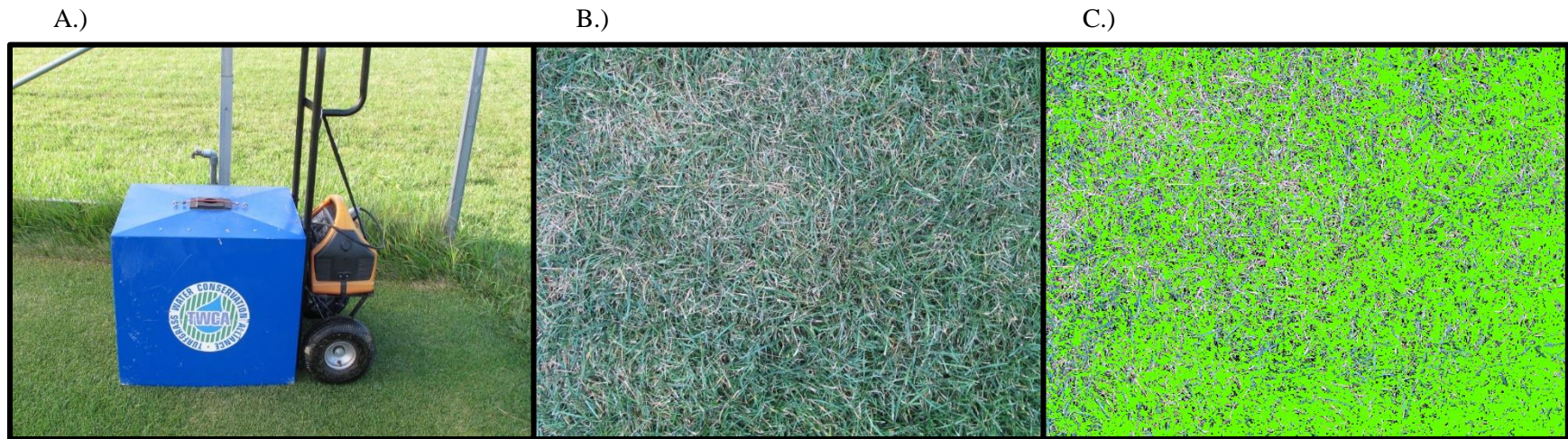
Figure A.3. Field study digital image measurement and analysis procedures. Digital image analysis was performed two times per week to quantify green coverage during deficit irrigation event. A light box equipped with an external battery (MotoMaster Eliminator PowerBox, Toronto, ON) to power four LED light bulbs (675 lumens, 5000 K) (A) was placed over the center of each plot to take a digital image (B). Images were taken using a Canon PowerShot G12 camera (Canon U.S.A. Inc., Huntington, NY). A Java-based software program, Turf Analyzer, was used to calculate green coverage (hue, saturation, and brightness ranges: 70-170, 10-100, 0-100, respectively) for the irrigation trigger using a 70% green coverage threshold ( GCT_{70} ) (C).
