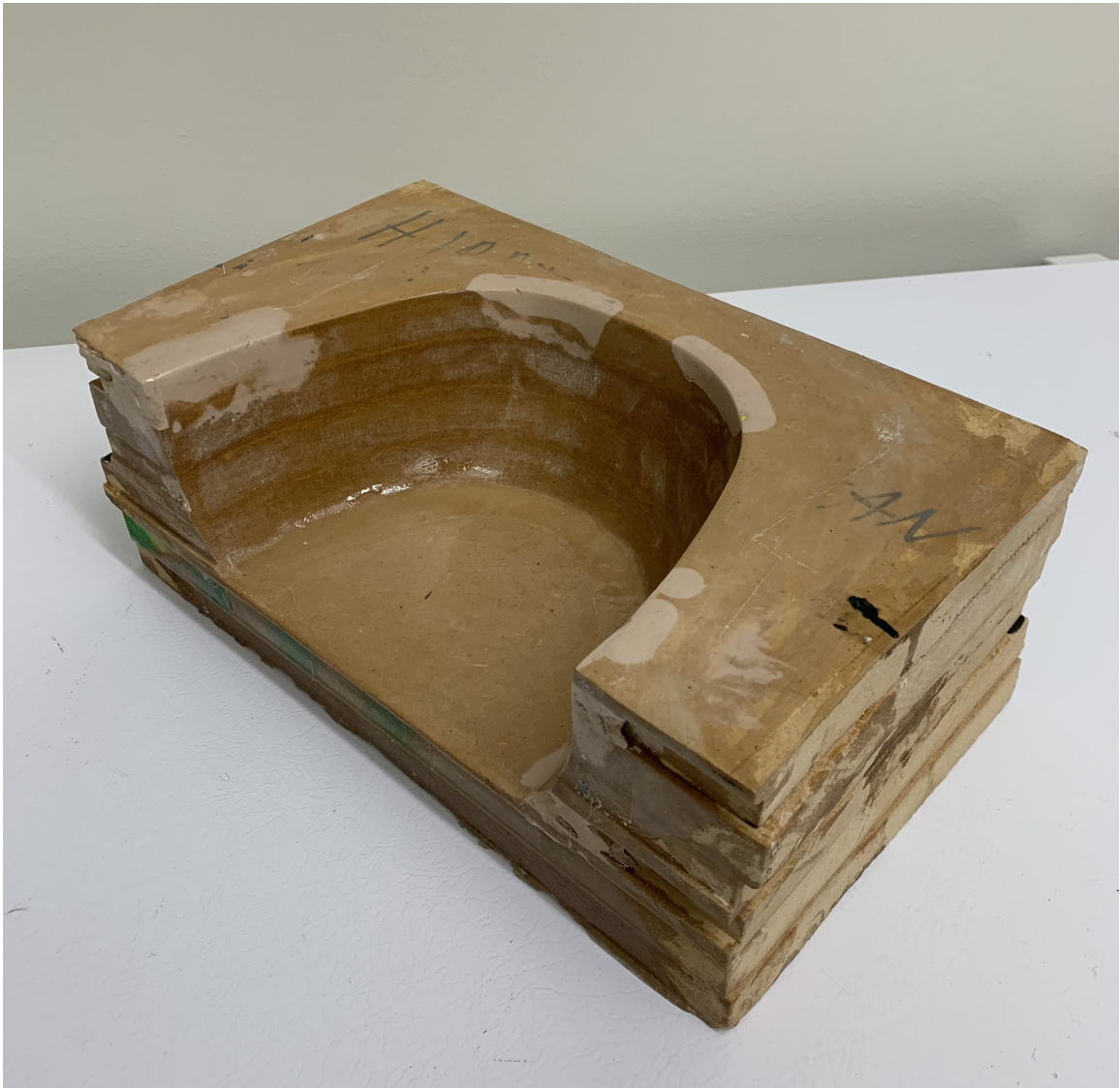
Fig. 3.4. Photograph taken of the real tool to be utilized during the manufacturing of the composite shell. MDF was the preferred material during construction, and clear sanding and CNC defects can be seen. A smooth surface finish was obtained, and the shiny appearance is given by the resin coating.
