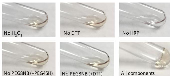
Fig. 4.1: Tilt test of HRP-mediated thiol-norbornene hydrogel. All components: 200 U/mL HRP, 0.5 mM  $\text{H}_2\text{O}_2$ , 3.5 wt% PEG8NB, and 14 mM DTT.
