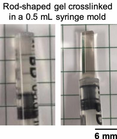
Fig. 4.5: HRP-crosslinked thiol-norbornene hydrogel with a diameter of 4 mm and a length of 15 mm (200 U/mL HRP, 0.5 mM  $\text{H}_2\text{O}_2$ , 3.5 wt% PEG8NB, and 14 mM DTT).
