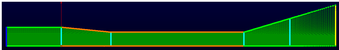
Fig. 2.7 2D Inlet-Isolator Grid Boundary Conditions
