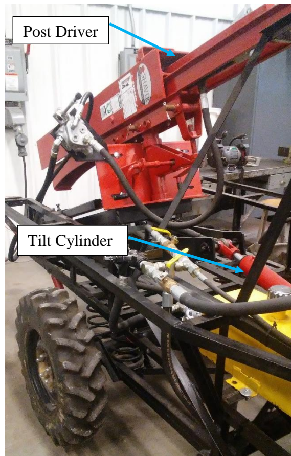
Figure 11 Basic Nomenclature of Well-Driver PUP (Personal photograph, 2018)
