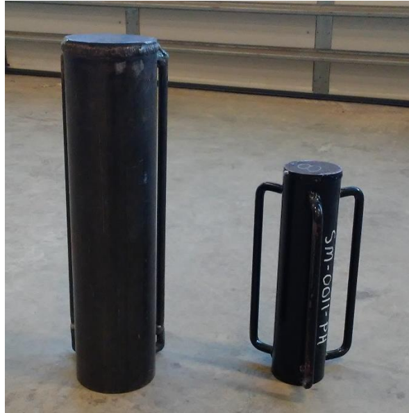
Figure 23 Shaver Drive Sleeve vs. Well Point Drive Sleeve Comparison (Personal photograph, 2019)
