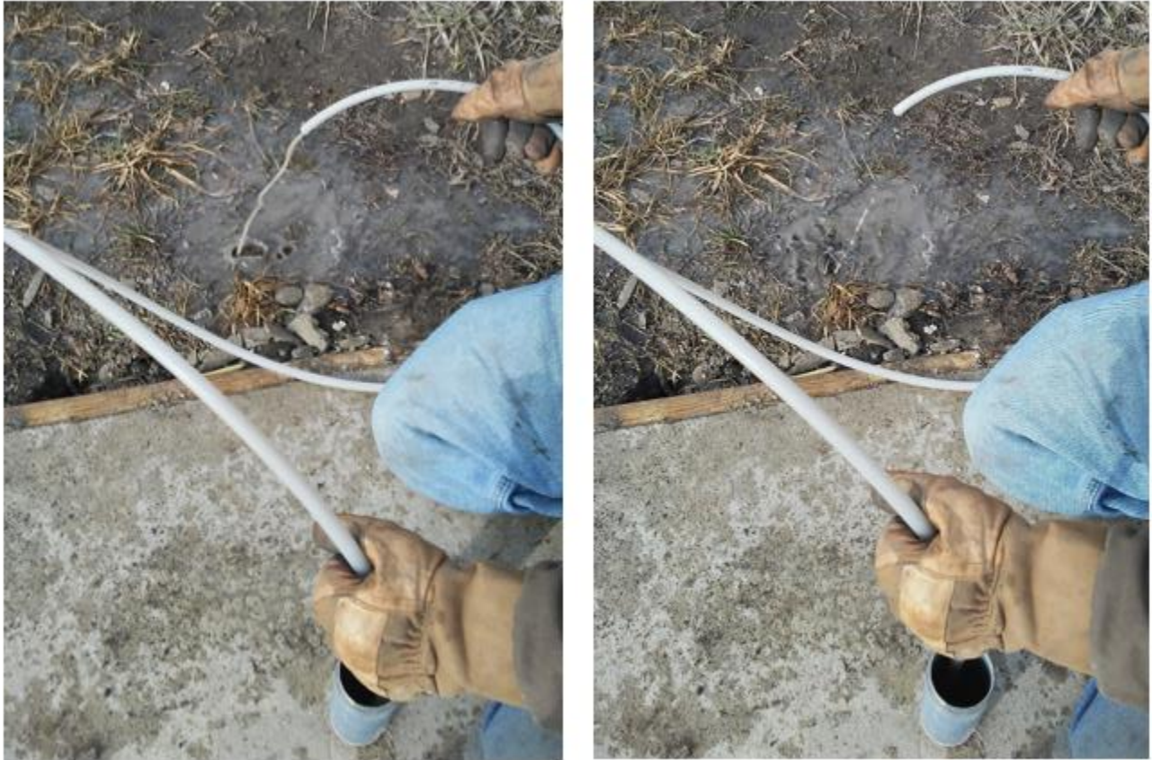
Figure 40 Surging Test Well 2 with an Inertial Pump (Personal photograph, 2019)
