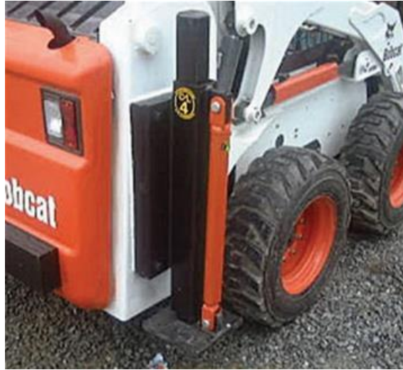
Figure 13 Skid Steer Outrigger Design (Everything, 2019)
