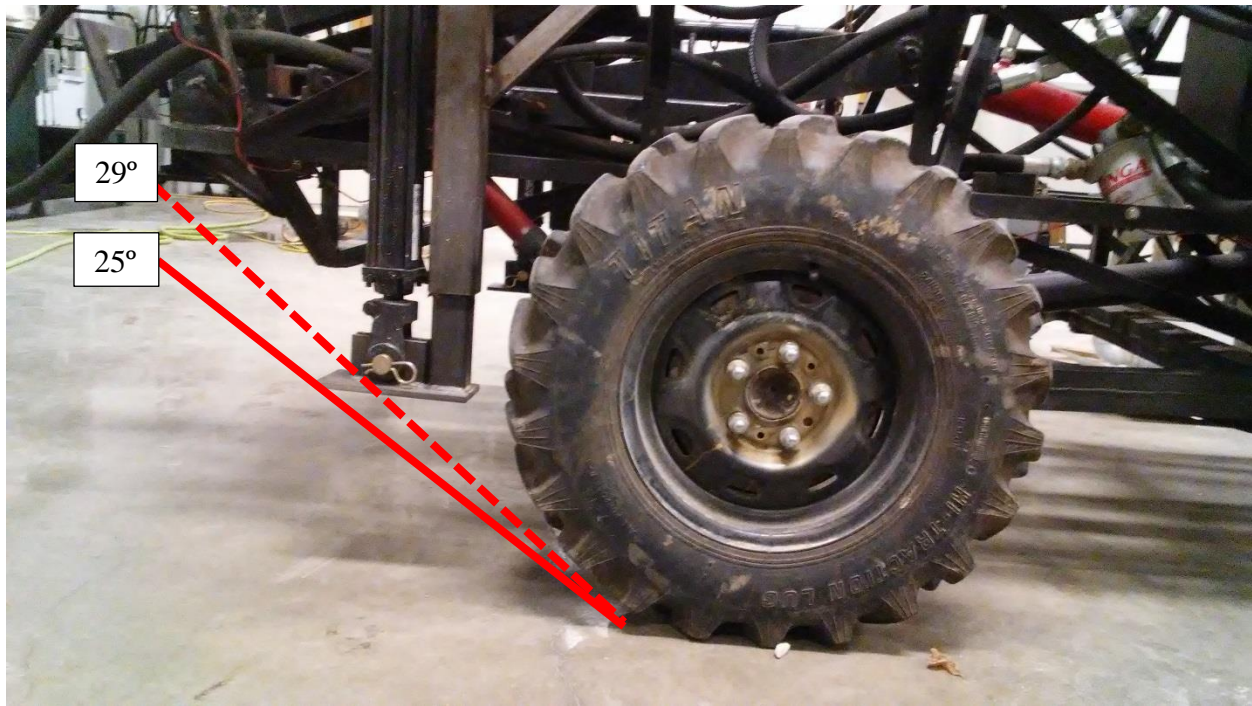
Figure 19 Reduction in Departure Angle Shown on PUP (Personal photograph, 2019)
