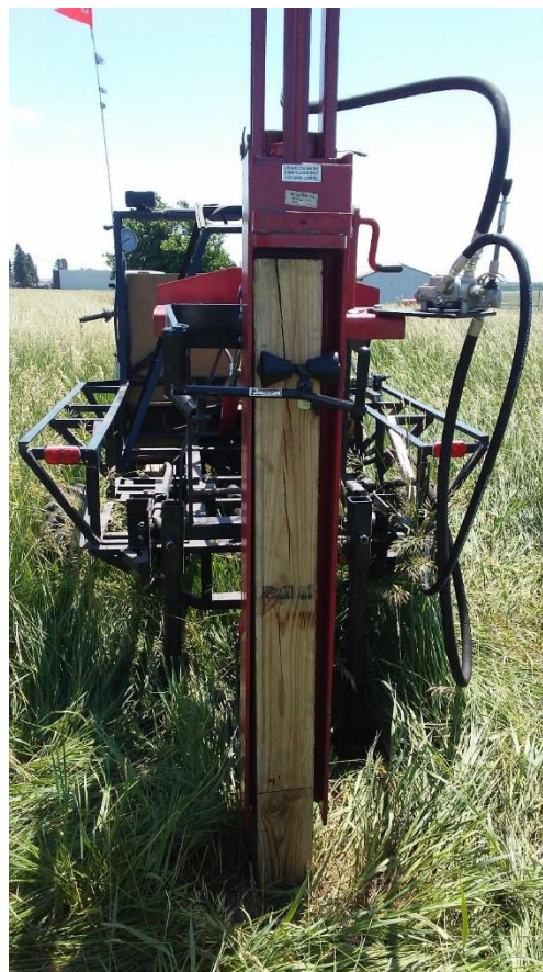
Figure 27 Test Driving a 4"x6" Wood Post (Personal photograph, 2018)
