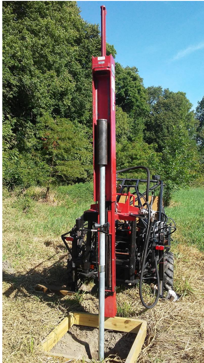
Figure 25 Fabricated Well Point Drive Sleeve in Use (Personal photograph, n.d.)
