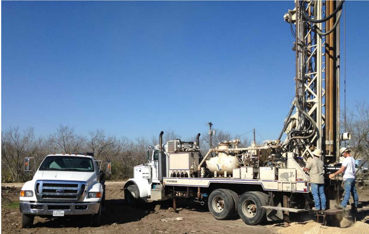
Figure 5 Typical Equipment for a Drilled Water Well (Utopia, n.d.)
