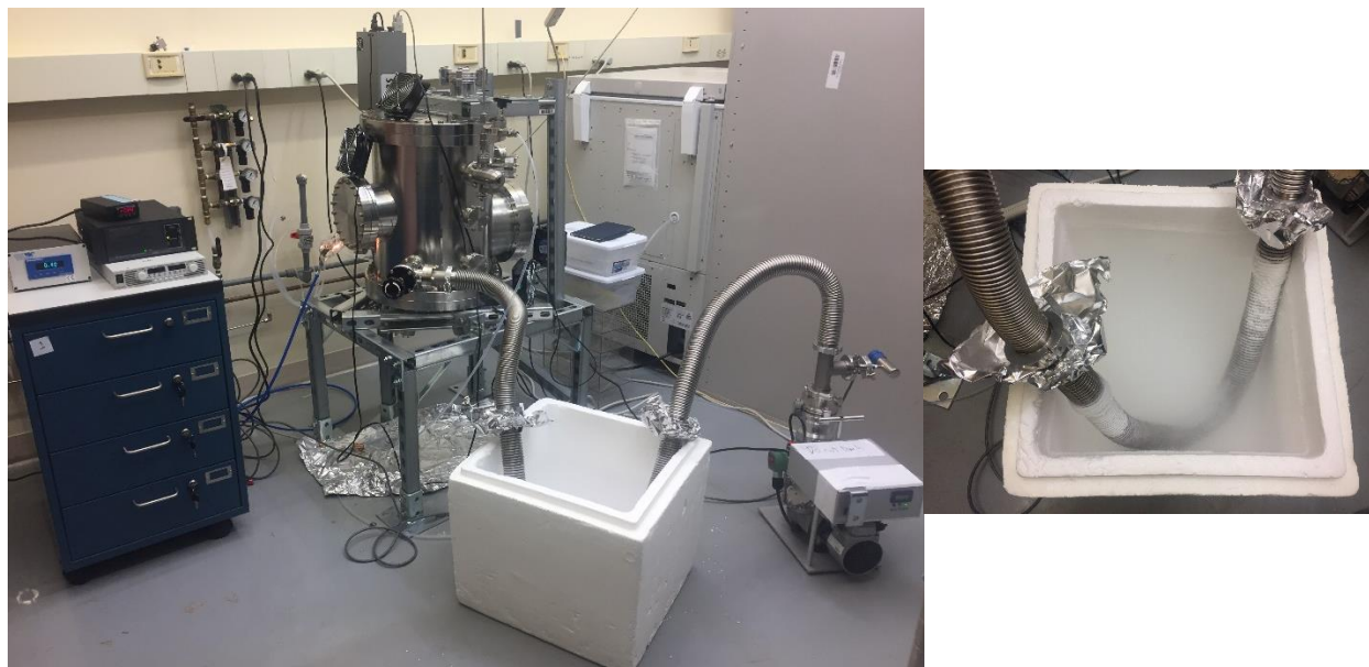
Fig. 6.18 Traps connected to the chamber in liquid nitrogen
