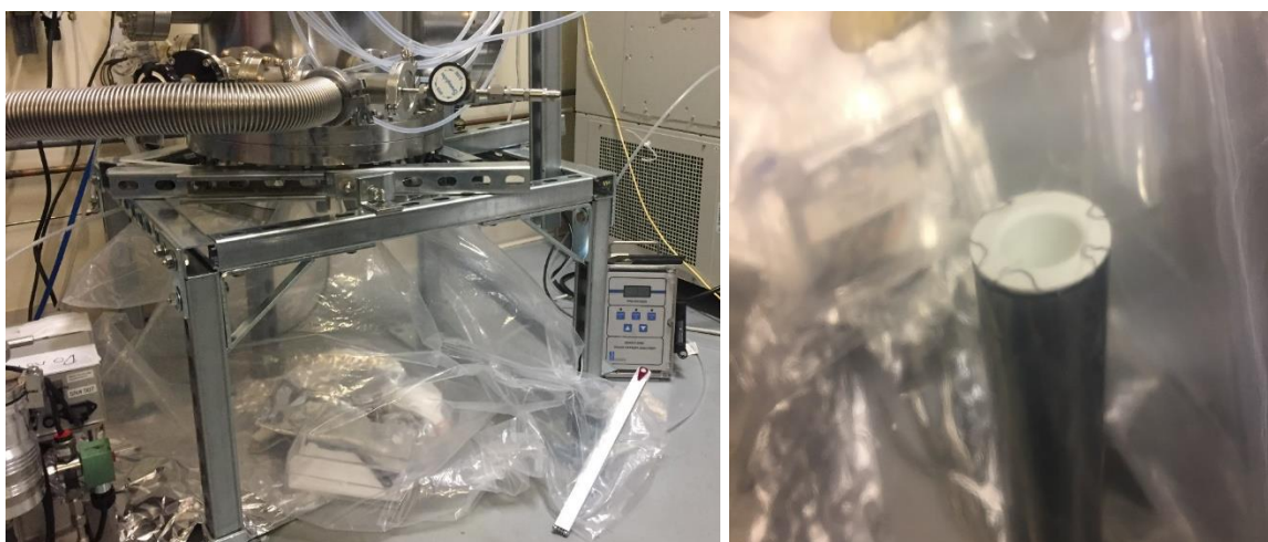
Fig. 6.12 Ar bag placed below chamber for crucible loading and the loaded crucible to the cell inside the Ar bag
